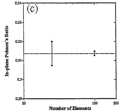
Figure 8. Effect of the number of Voronoi cell elements on the range of in-plane properties for the microstructure consisting of 0.2 volume fraction of elliptical inclusions (aspect ratio in the range 1–2). One of the 100 element square RMEs used is shown in (a), while one of the 25 element square RMEs used is shown in Figures 5(a) and 5(b).
