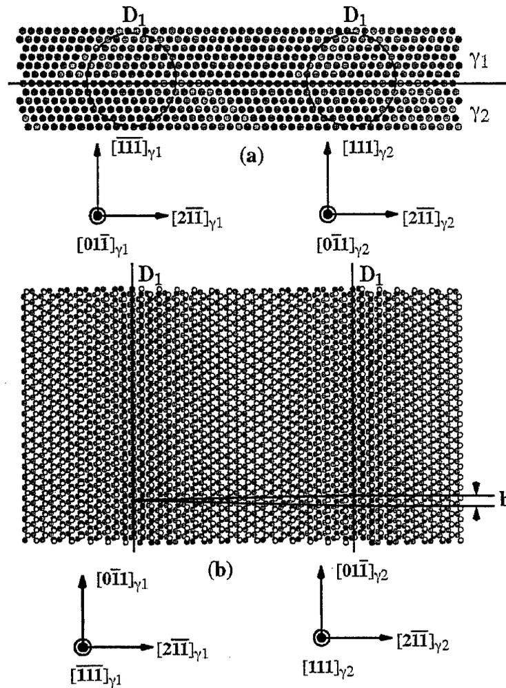
Figure 10 Equilibrium configuration of the  $(\bar{1}11)_{\gamma_1}/(111)_{\gamma_2}$  interface (bicrystal D): (a) Atomic positions projected onto the  $(01\bar{1})_{\gamma_1}/(0\bar{1}1)_{\gamma_2}$  plane; (b) Atomic positions projected onto the  $(\bar{1}11)_{\gamma_1}/(111)_{\gamma_2}$  interface plane. Interfacial screw dislocations are marked as  $D_1$ .
