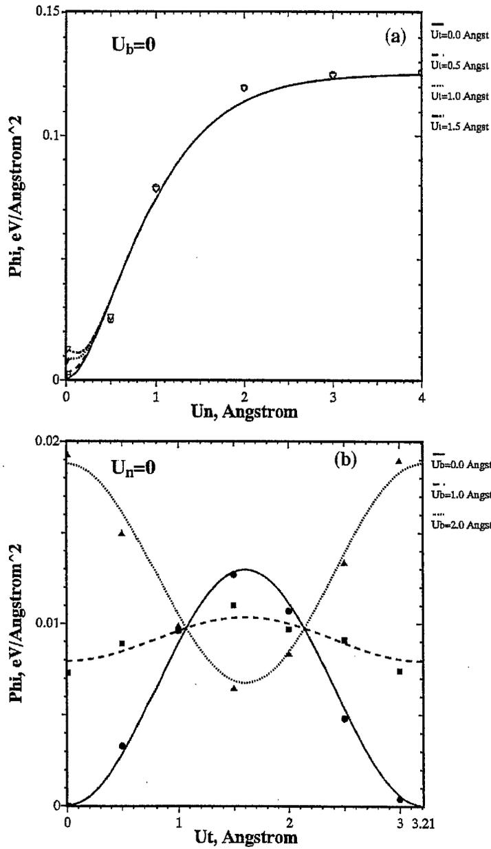
Figure 11 Variation of the decohesion potential for the  $(110)_\beta/(111)_\gamma$  interface with the normal displacement  $U_n$  in the  $[\bar{1}\bar{1}0]_\beta/[\bar{1}\bar{1}\bar{1}]_\gamma$  direction and tangential displacements  $U_t$  and  $U_b$  in the  $[001]_\beta/[0\bar{1}\bar{1}]_\gamma$  and  $[\bar{1}\bar{1}0]_\beta/[2\bar{1}\bar{1}]_\gamma$  directions, respectively.
