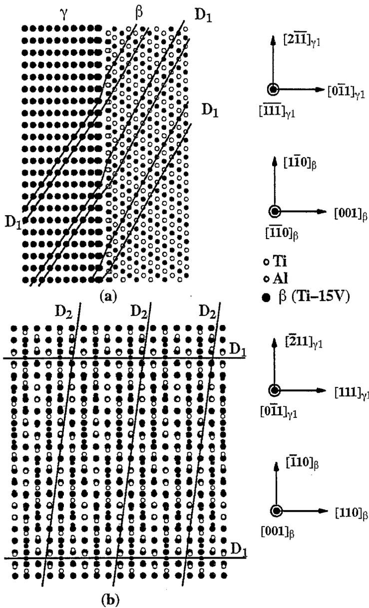
Figure 8 Equilibrium configuration of the  $(001)_{\beta}/(0\bar{1}\bar{1})_{\gamma}$  interface (bicrystal B): (a) Atomic positions projected onto the  $(\bar{1}\bar{1}0)_{\beta}/(\bar{1}\bar{1}\bar{1})_{\gamma}$  plane; (b) Atomic positions projected onto the  $(001)_{\beta}/(0\bar{1}\bar{1})_{\gamma}$  interface plane. Interfacial dislocations are marked as  $D_1$  and  $D_2$ .
