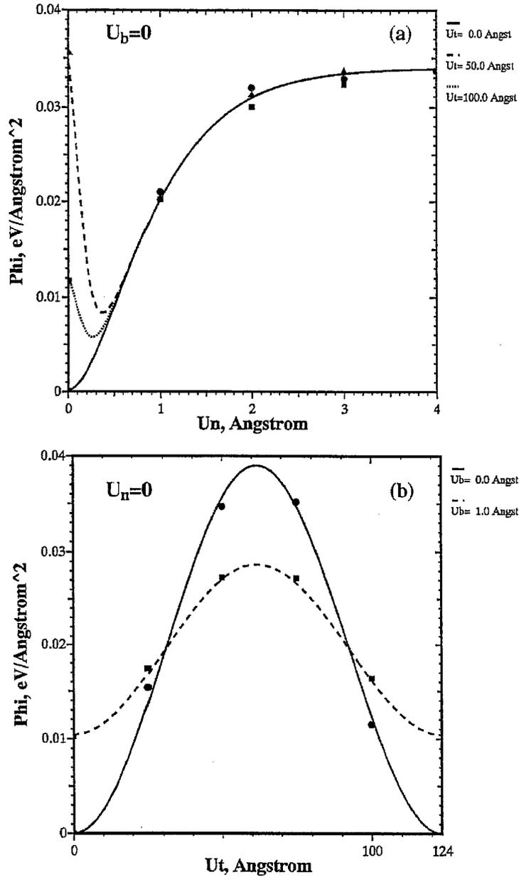
Figure 14 Variation of the decohesion potential for the interface  $(111)_{\gamma_1}/(111)_{\gamma_2}$  with the normal displacement  $U_n$  in the  $[\bar{1}\bar{1}\bar{1}]_{\gamma_1}/[111]_{\gamma_2}$  direction and tangential displacements  $U_t$  and  $U_b$  in the  $[0\bar{1}\bar{1}]_{\gamma_1}/[01\bar{1}]_{\gamma_2}$  and  $[2\bar{1}\bar{1}]_{\gamma_1}/[2\bar{1}\bar{1}]_{\gamma_2}$  directions, respectively.
