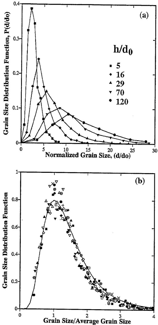
Figure 4. (a) The distribution function for the grain size normalized with respect to the average nucleus spacing,  $d_0$ , at five film thicknesses for the growth-rate parameter  $\alpha=1.5$ . (b) The distribution function for the grain size normalized with respect to the corresponding average grain size,  $\bar{d}$ , for five  $\alpha$  values and three film thicknesses.
