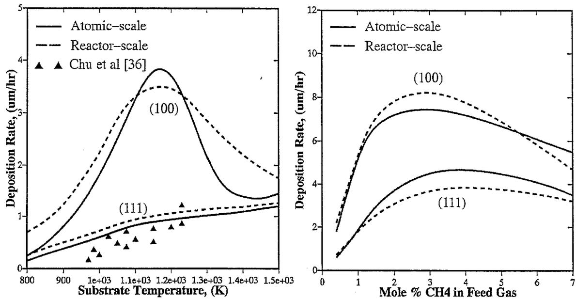
Figure 5. Reactor- and atomic scale analyses predicted (111)- and (100)-oriented film deposition rates as a function of (a) the substrate temperature and (b) concentration of CH<sub>4</sub> in feed gas. The remaining processing condition are as indicated in Figure 4.
