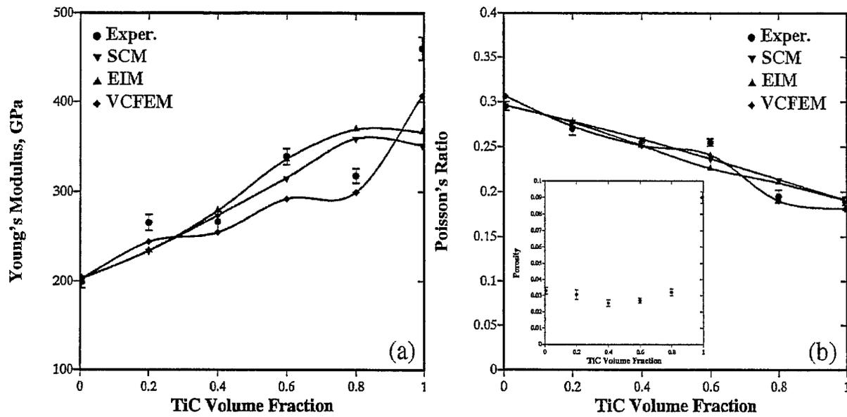
Figure 11. Comparison of the experimentally measured Young's modulus (a) and Poisson's ratio (b) in Ni<sub>3</sub>Al/TiC FGM with the ones predicted by the Self Consistent Method (SCM), the Equivalent Inclusion Method (EIM) and the Voronoi Cell Finite Element Method (VCFEM). The experimentally measured porosities are shown in the insert of figure (b).
