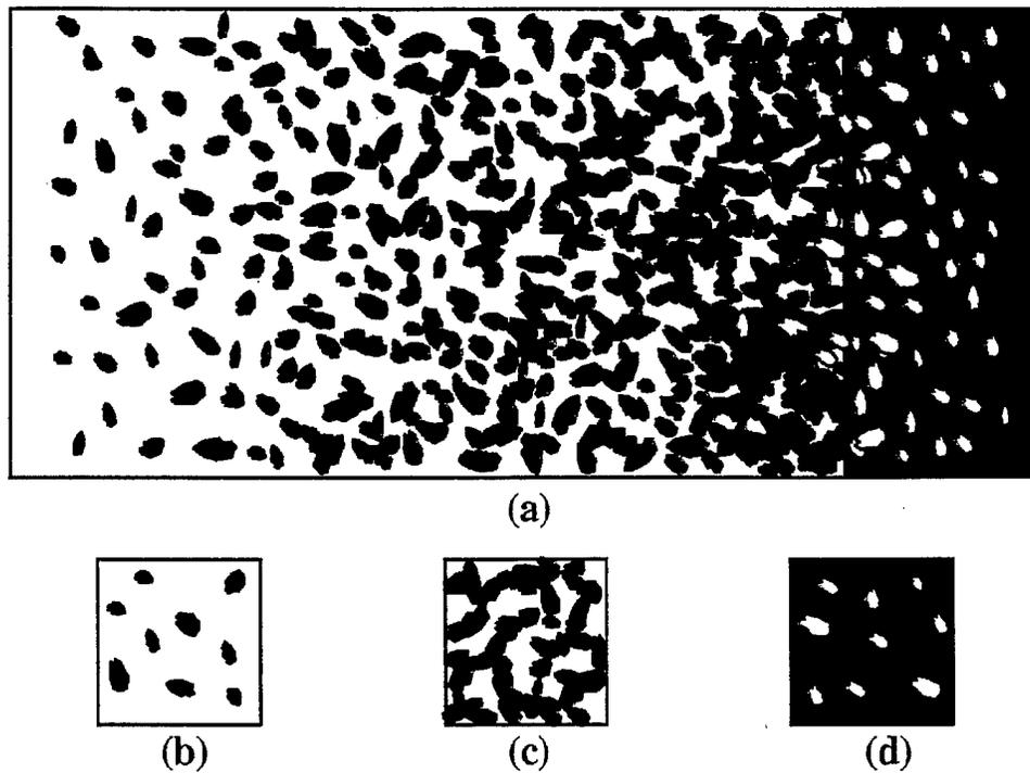
**Figure 5. (a) Schematic representation of the microstructure of a graded ceramic/metal region. The microstructure consisting of dispersed particles embedded in a continuous matrix is observed for large and small volume fractions of the metal and ceramic, as in (b) and (d). In the intermediate region where the volume fractions of the two materials are comparable to each other, the microstructure consists of intertwined clusters of the two phases.**
