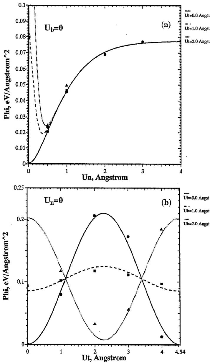
Figure 12 Variation of the decohesion potential for the interface  $(001)_\beta/(011)_\gamma$  with the normal displacement  $U_n$  in the  $[001]_\beta/[0\bar{1}1]_\gamma$  direction and tangential displacements  $U_t$  and  $U_b$  in the  $[1\bar{1}0]_\beta/[\bar{1}\bar{1}1]_\gamma$  and  $[1\bar{1}0]_\beta/[2\bar{1}\bar{1}]_\gamma$  directions, respectively.
