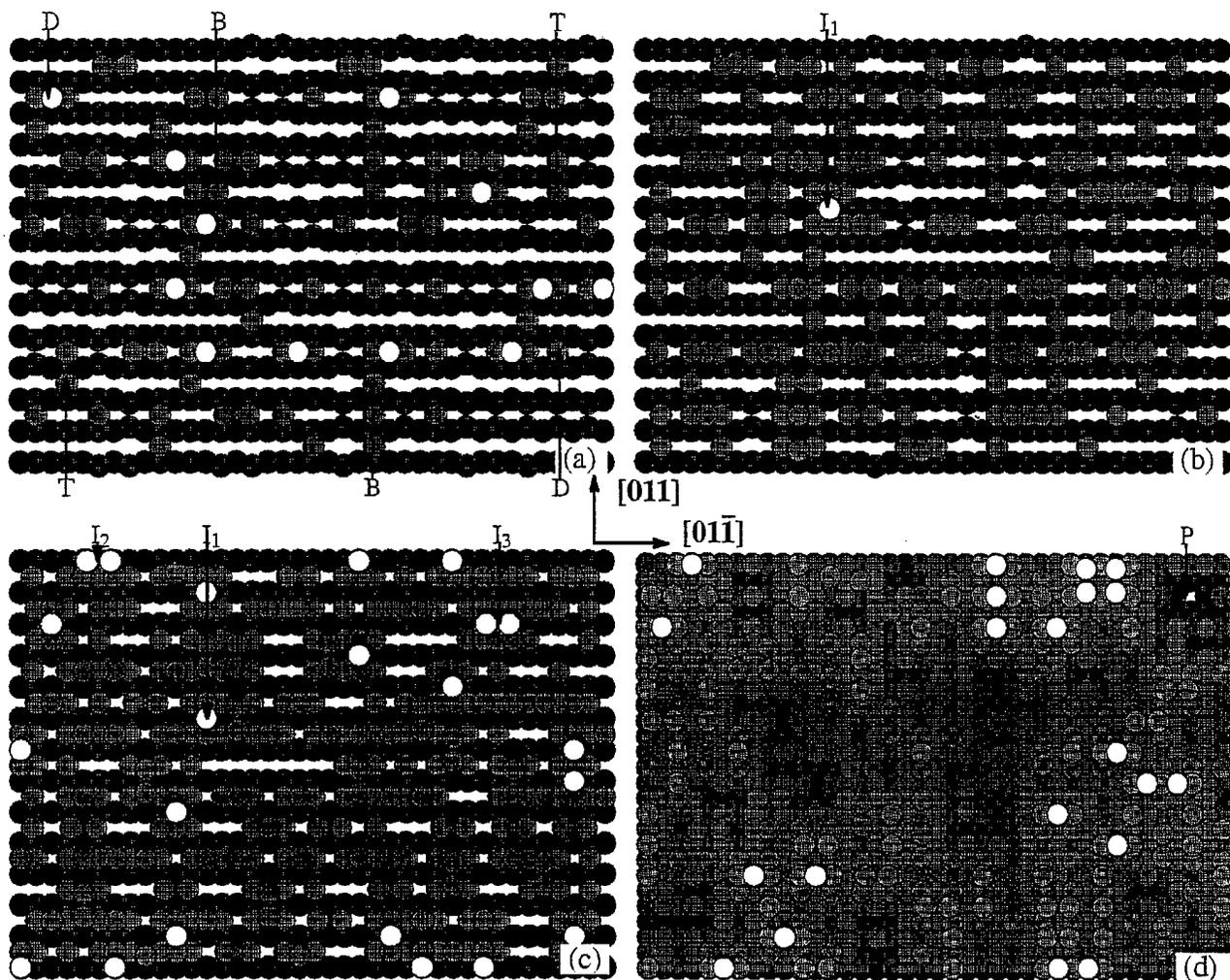
Figure 9. Top view of four (100) surface configurations obtained under the CVD conditions identical to the ones listed in Figure 5. Deposition times: (a) 0.01s; (b) 0.018s; (c) 0.032s and (d) 0.208s. Nomenclature: B—BCN mechanism, D—Dimer insertion mechanism, P—Pit, I—Island, T—Trough insertion mechanism.
