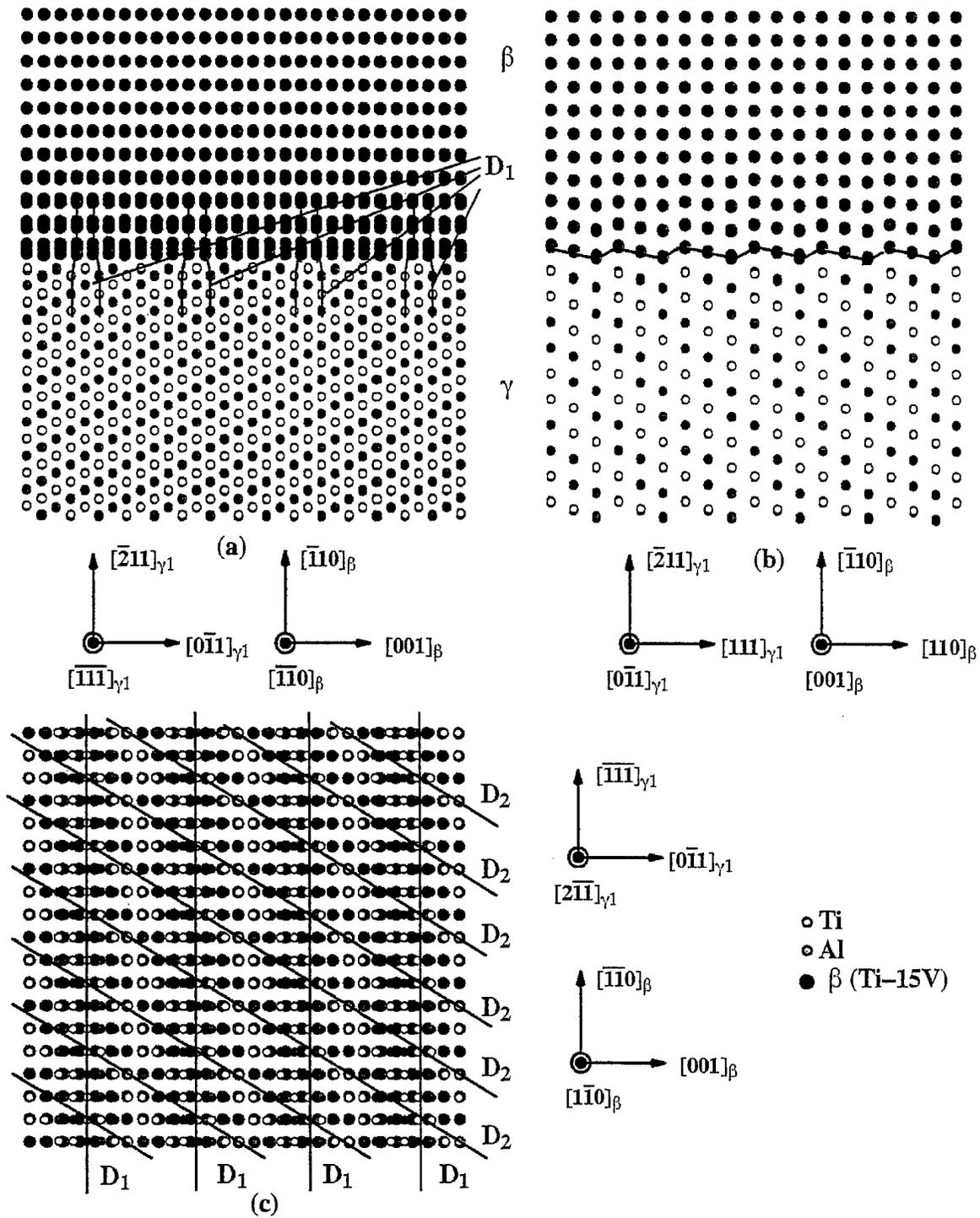
Figure 9 Equilibrium configuration of the  $(1\bar{1}0)_\beta / (2\bar{1}\bar{1})_\gamma$  interface (bicrystal C): (a) Atomic positions projected onto the  $(\bar{1}\bar{1}0)_\beta / (\bar{1}\bar{1}\bar{1})_\gamma$  plane; (b) Atomic positions projected onto the  $(001)_\beta / (0\bar{1}\bar{1})_\gamma$  plane; (c) Atomic positions projected onto the  $(1\bar{1}0)_\beta / (2\bar{1}\bar{1})_\gamma$  interface plane. Interfacial dislocations are marked as  $D_1$  and  $D_2$ .
