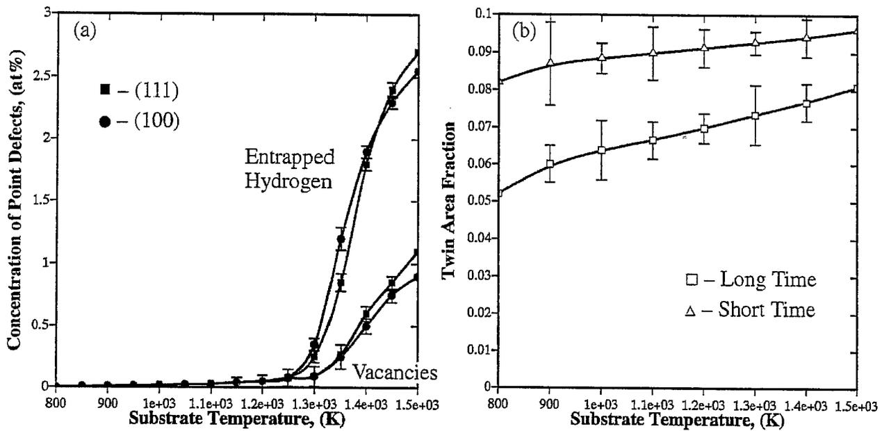
Figure 8. Effect of the substrate temperature on the concentration of vacancies and entrapped hydrogen atoms in (111)- and (100)-oriented diamond films, (a), and twins in (111)-oriented diamond films, (b), under the CVD conditions specified in Figure 5. Error bars represent on standard deviation over five simulation runs.
