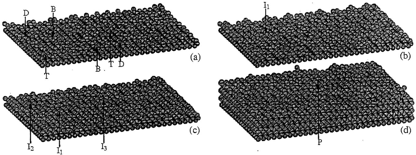
Figure 10. Side view of the four (100)-oriented diamond films shown in Figures 9(a)-(d).
