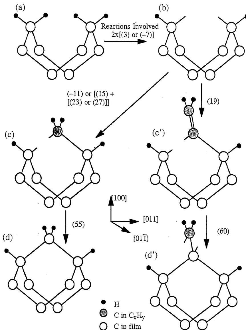
Figure 3. Growth of a (100)-oriented film by trough insertion mechanism. Open circles represent diamond carbon atoms, shaded circles designate hydrocarbon carbon atoms, and small black circles stand for hydrogen atoms. Surface reactions (listed in Table I) involved in various steps of the process are given in parenthesis.
