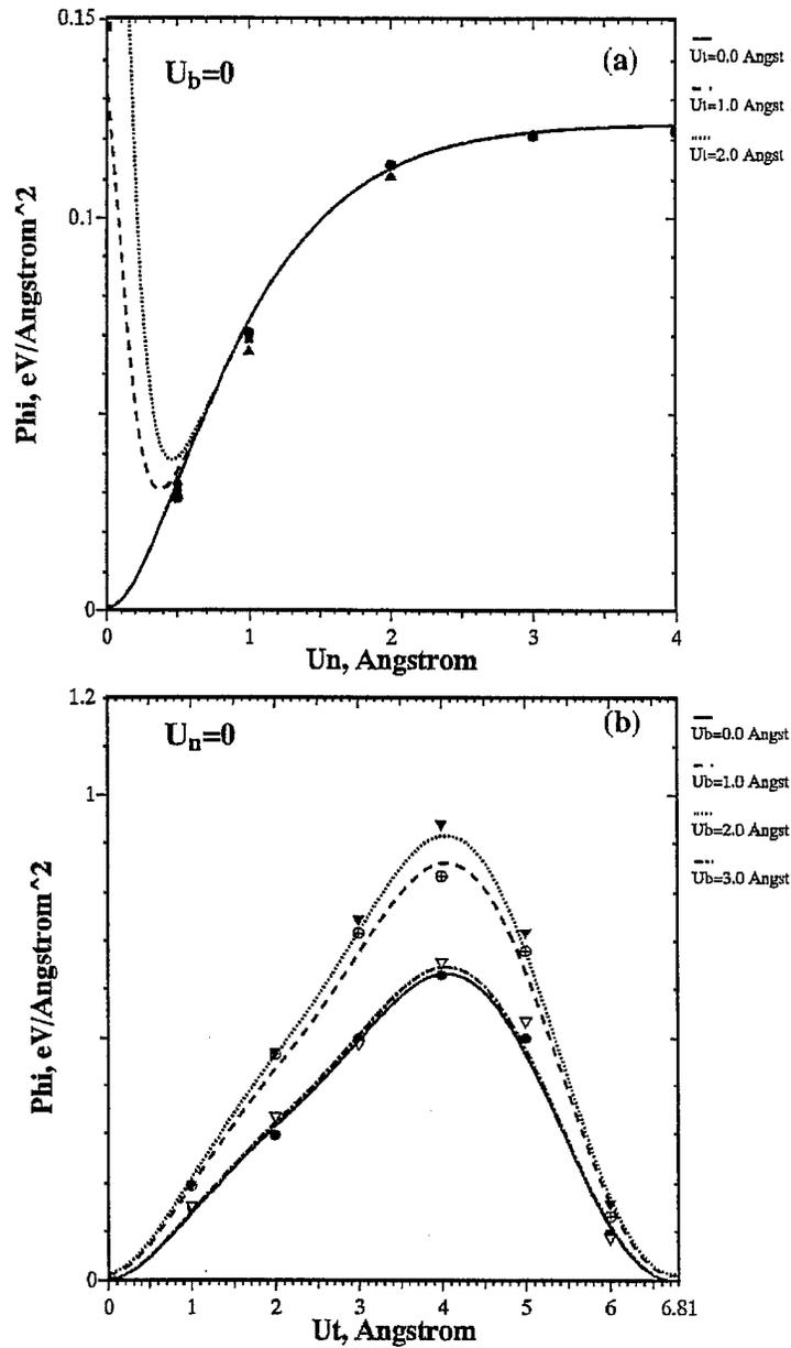
Figure 13 Variation of the decohesion potential for the interface  $(110)_\beta/(211)_\gamma$  with the normal displacement  $U_n$  in the  $[\bar{1}\bar{1}0]_\beta/[2\bar{1}\bar{1}]_\gamma$  direction and tangential displacements  $U_t$  and  $U_b$  in the  $[\bar{1}10]_\beta/[\bar{1}\bar{1}1]_\gamma$  and  $[001]_\beta/[0\bar{1}1]_\gamma$  directions, respectively.
