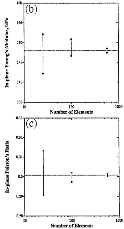
Figure 9. Effect of the number of Voronoi cell elements on the range of in-plane properties for the microstructure consisting of intertwined clusters of the two materials (volume fraction of the two materials  $\approx 0.5$ ). One of the 600 element RMEs used is shown in (a).
