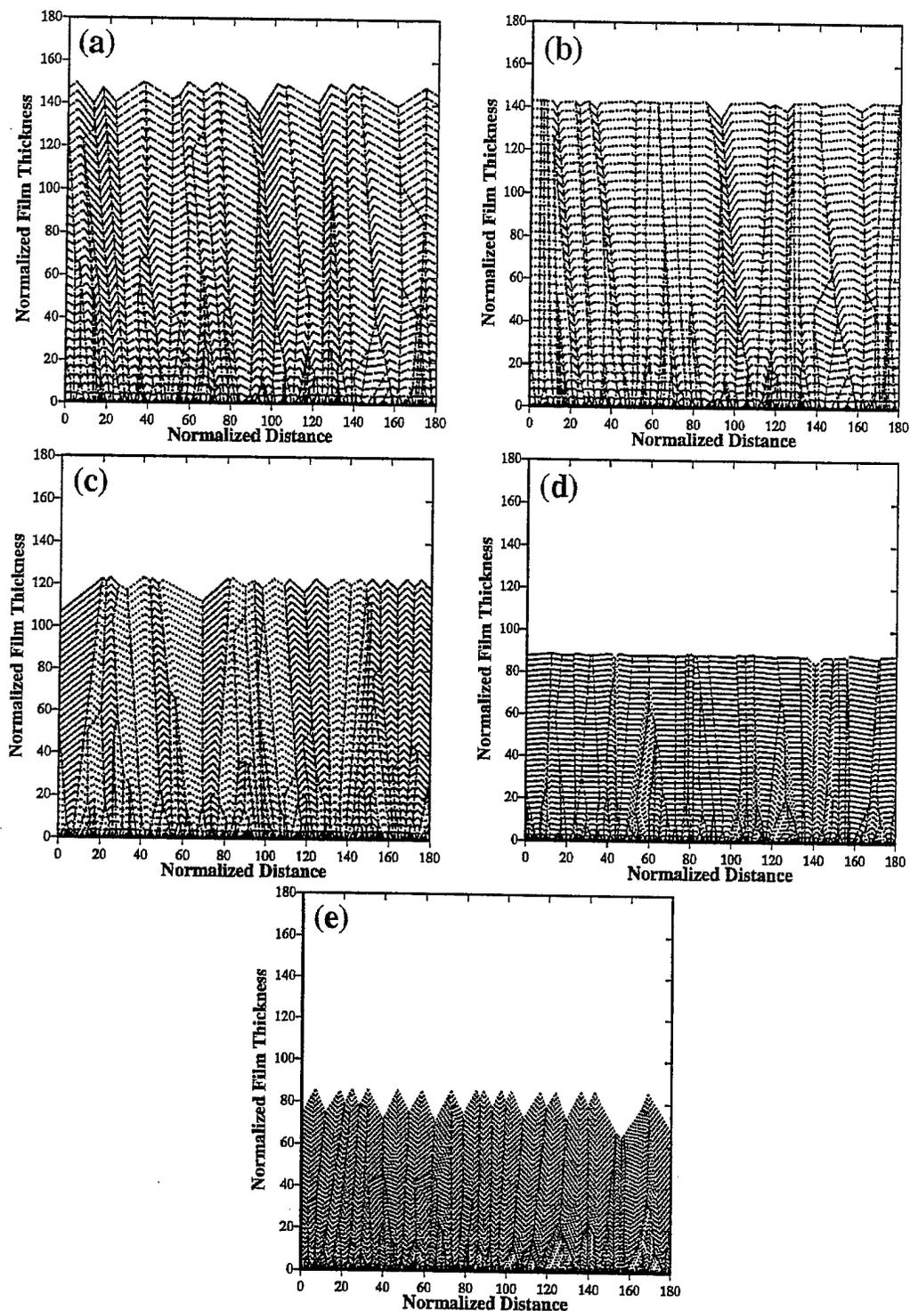
Figure 2. The microstructure of polycrystalline diamond films deposited under the growth-rate parameter,  $\alpha$  =: (a) 1.0; (b) 1.05; (c) 1.5; (d) 2.95 and (e) 3.0. Both the x- and y-axis are normalized with respect to the average nucleus spacing,  $d_0$ . The following line type nomenclature is used: dash-dot=grain boundaries, solid={100} facets, dotted = {111} facets, dashed = {100}/{100} facets, and three-dot space={111}/{111} facets.
