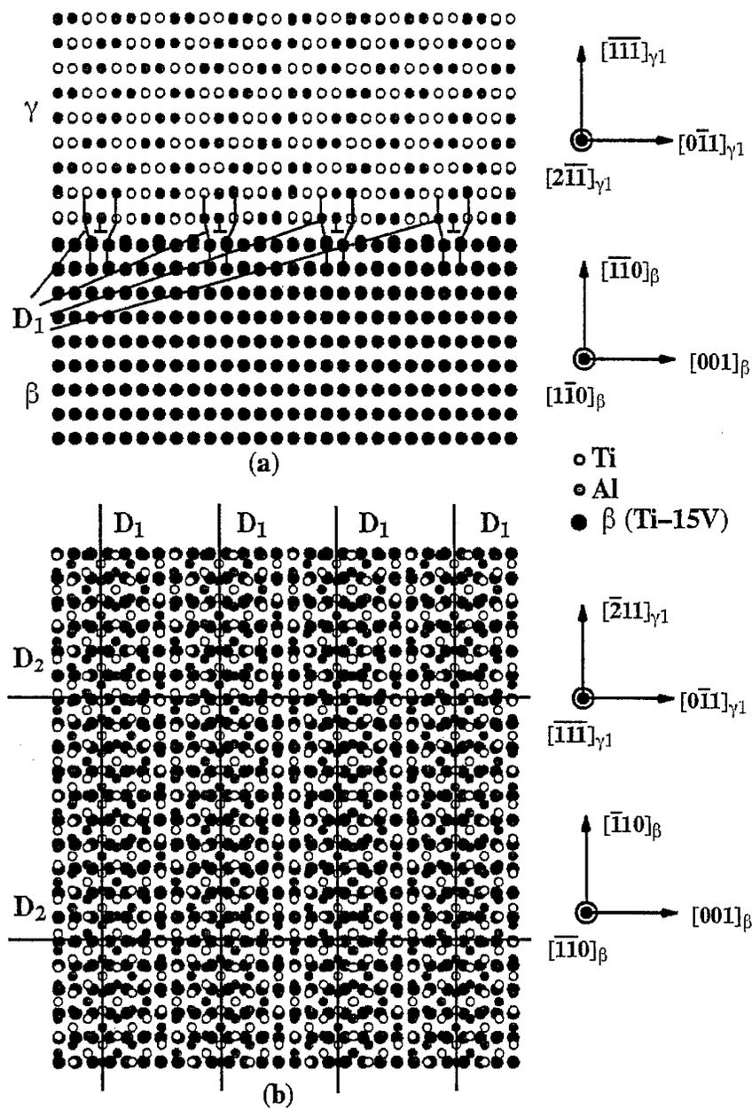
Figure 7 Equilibrium configuration of the  $(\bar{1}\bar{1}\bar{0})_{\beta}/(\bar{1}\bar{1}\bar{1})_{\gamma}$  interface (bicrystal A): (a) Atomic positions projected onto the  $(\bar{1}\bar{1}\bar{0})_{\beta}/(2\bar{1}\bar{1})_{\gamma}$  plane; (b) Atomic positions projected onto the  $(\bar{1}\bar{1}\bar{0})_{\beta}/(\bar{1}\bar{1}\bar{1})_{\gamma}$  interface plane. Interfacial dislocations are marked as  $D_1$  and  $D_2$ .
