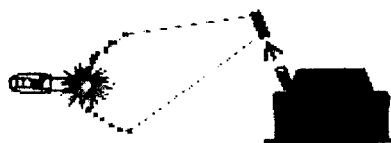
Figure 19: Schematic ARENA hard kill protection against missiles and rockets.
