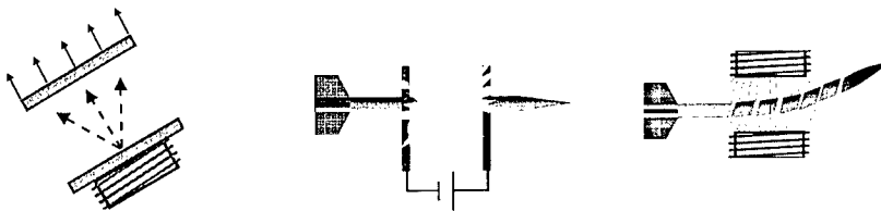
Figure 11: The major principles for electromagnetic armour.
