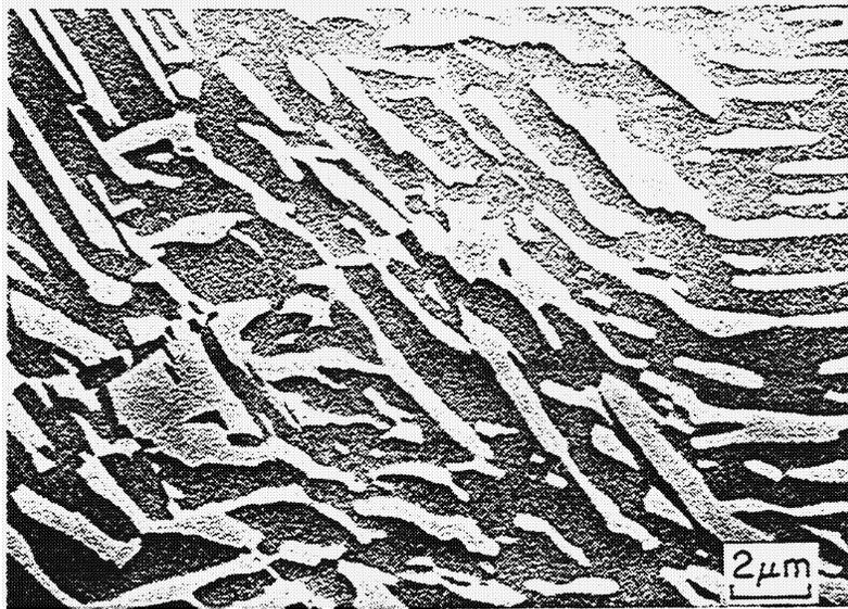
Figure 35. Ti-22Al-27Nb, beta solutionized and aged 500 hours at 900°C. O+B2 in alloy containing 1120 wppm oxygen. [Ref. 58]
