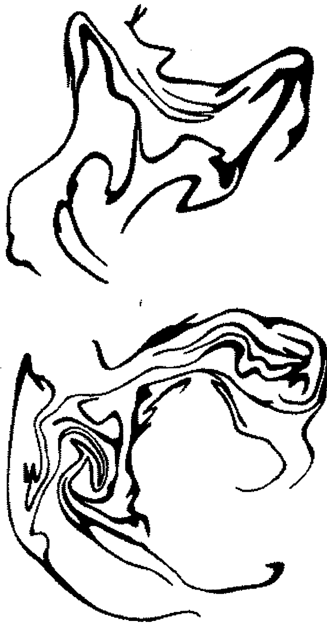
Figure 11: Further deformation of the butanol square in figure 10. According to Batchelor [1], the length of the filaments increases exponentially with t .
