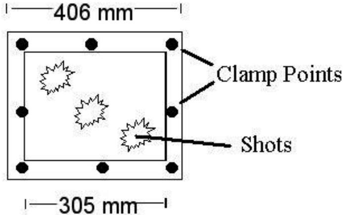
Figure 7. Front View of Ballistic Clamp Fixture.
