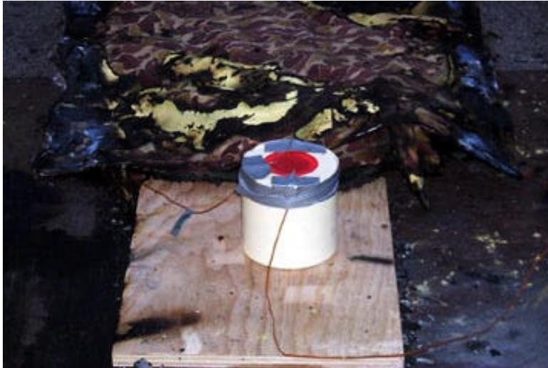
Figure 51. Instrumented Acceptor Stack of Ammunition After Several Experiments.
