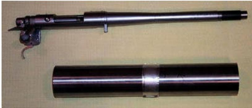
Figure 8. Modified Remington 700 Rifle (top) With 40-mm Smooth Bore Fragment Launcher Attachment (bottom).
