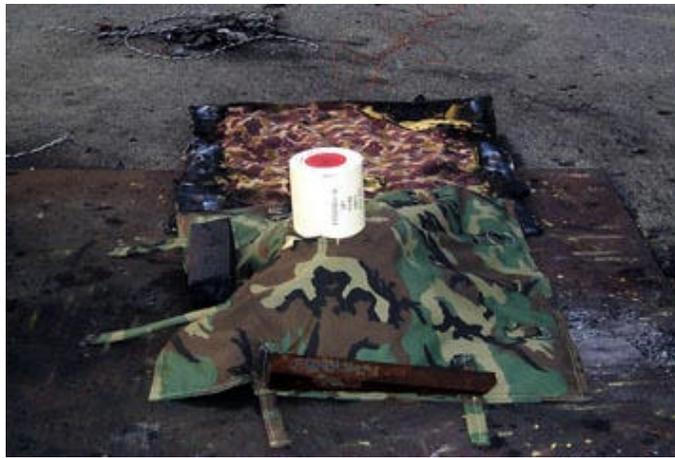
Figure 45. Uni-charge Placed on Top of a Covered Live (Uni-charge) Acceptor Before Ignition.
