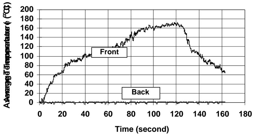
a. Unpainted shiny side (1000/800 aluminum) was exposed to  $84 \text{ kW/m}^2$  for 120 seconds.
