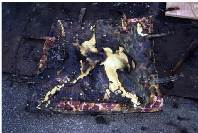
Figure 46. Typical Results From the Ignition of a Uni-charge on Top of an MST Blanket.
