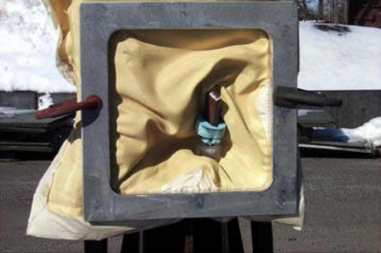
Figure 26. Blanket Clamped in Frame Impacted by a 454-g Steel Fragment.
