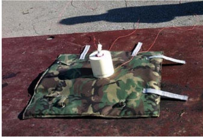
Figure 44. Uni-charge Placed on Top of a Covered Inert Acceptor Before Ignition.
