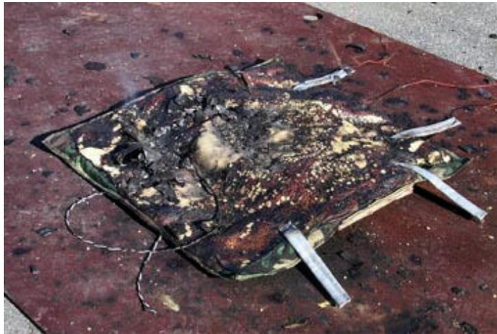
Figure 34. Typical Charred Remains of a Top-Burn Live Propellant Experiment.
