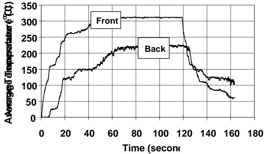
a. Unpainted surface was exposed to 84 kW/m<sup>2</sup> for 120 seconds.
