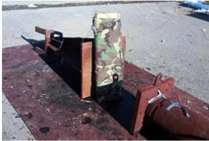
Figure 39. Setup of Uni-charge Experiment, in Which Four Uni-charge Packages Were Placed Inside the Steel Tube.
