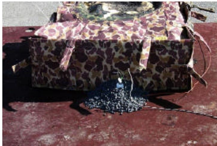
Figure 31. Side Burn Propellant Experiment (0.5 kg JA2) on a Covered Inert Acceptor Ammunition Crate.
