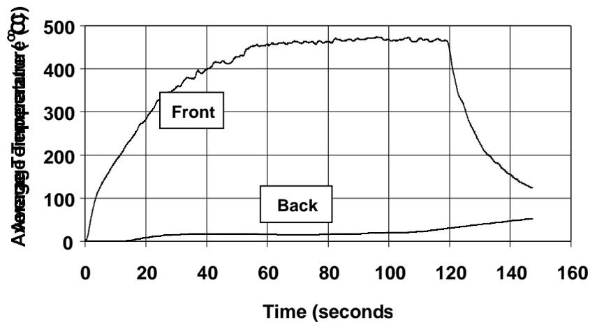
c. Black painted beige side (188 CH) was exposed to  $84 \text{ kW/m}^2$  for 120 seconds.
