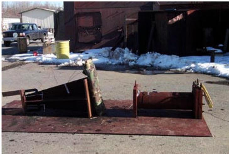
Figure 40. Setup of Uni-charge Experiment, Showing Stand-off Distance.
