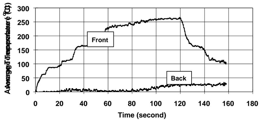
b. Unpainted beige side (188 CH) was exposed to  $84 \text{ kW/m}^2$  for 120 seconds.
