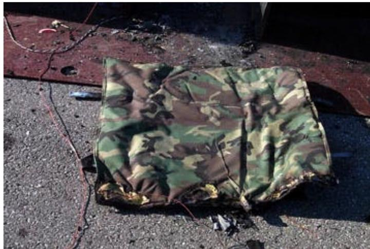
Figure 42. Back Surface of a Blanket Subjected to a Hot Gas Jet Emitted From Four Uni-charge Packages.
