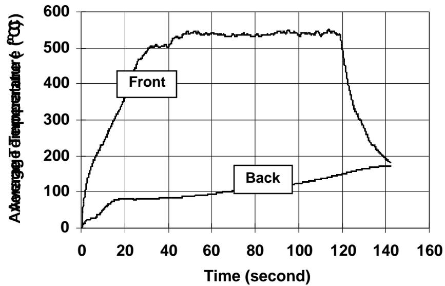
b. Black painted surface was exposed to 84 kW/m<sup>2</sup> for 120 seconds.
