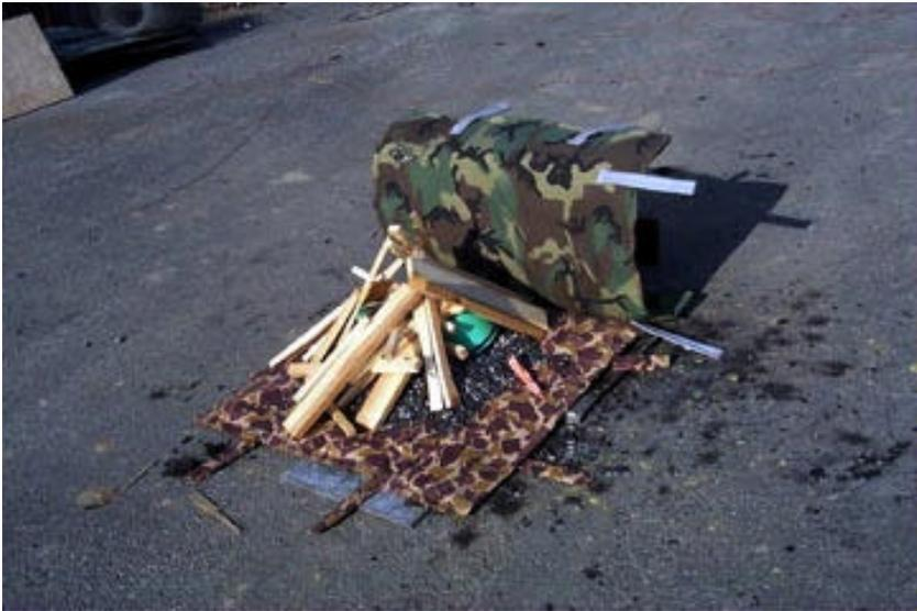
Figure 35. Setup of Bonfire Experiment Before Ignition.
