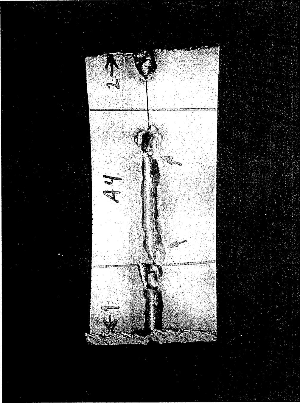
Figure 4-27: Root Face of Weld A4, Section 1-2
