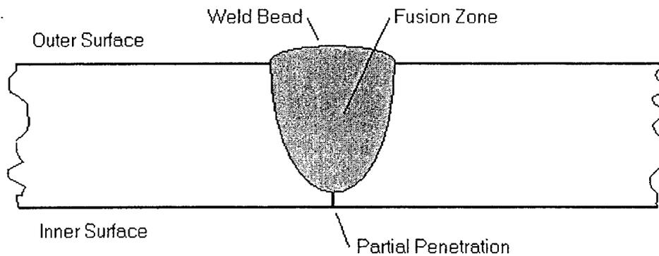
Figure 1-1: Schematic of a Partially Penetrated Weld Joint
