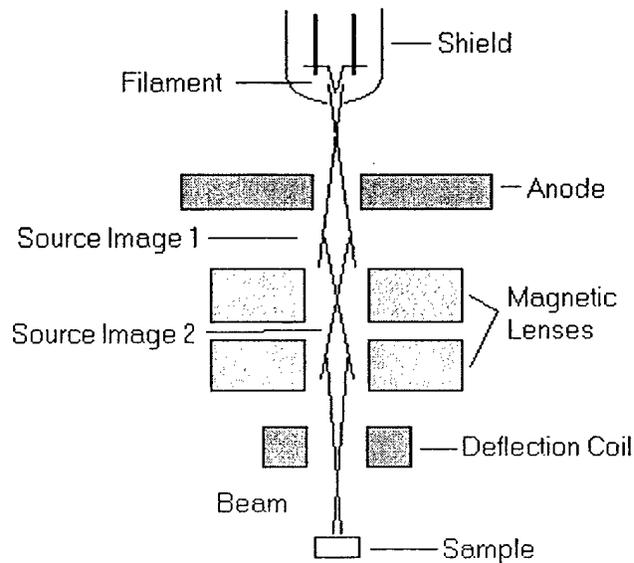
Figure B-1: SEM Cross-section
