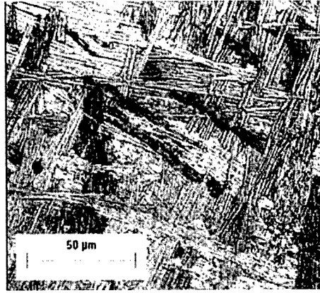
Figure 10: Microstructure of a layer band in the as-deposited material consisting of coarse colonies of acicular \alpha outlined in \beta .
