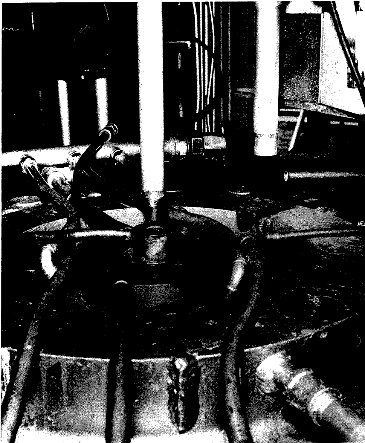
Figure 3.- Coated model in test position in Langley 11-inch ceramic-heated tunnel.
