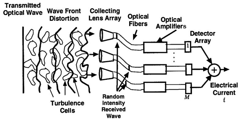
**Figure 1** Array of  $M$  direct detection receivers.
