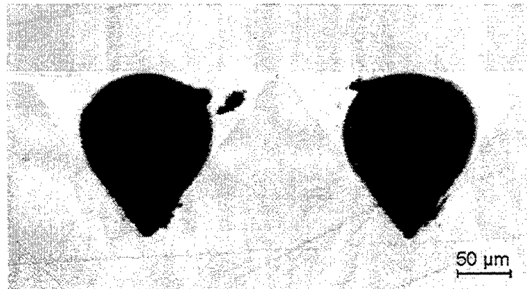
Fig. 20: Laser beam soldered fibers
