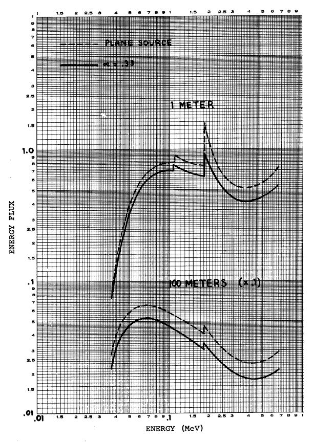
Figure 14. Differential energy spectra of the scattered energy flux at 1 and 100 meters for a .662 MeV source ( $^{137}$ Cs).
