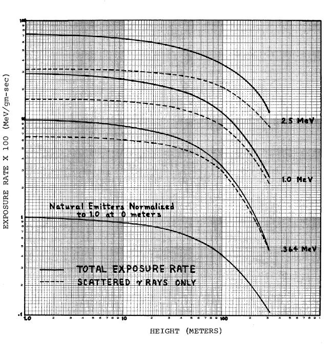
Figure 1. Total and scattered exposure rates versus height for uniformly distributed sources with energies of .364, 1.0 and 2.5 MeV and the single normalized curve of exposure rates for natural emitters.
