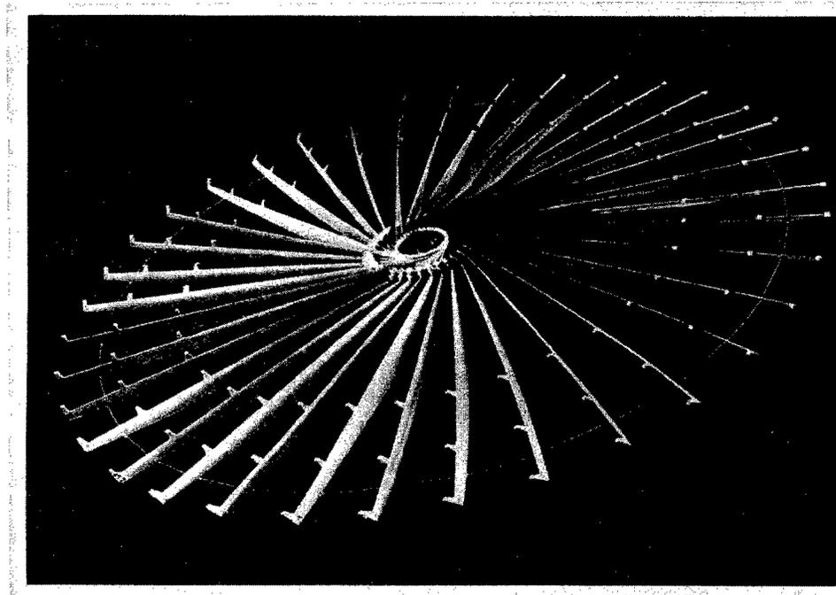
*The Homing Overlay Experiment (HOE) used a warhead that expanded to destroy incoming warheads. In June 1984 it successfully intercepted a non-nuclear reentry vehicle. Credit: US Army Space and Strategic Defense Command*
