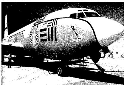
*Airborne laser laboratory. The Air Force conducted considerable number of experiments to support the concept of a laser based on an airborne platform to destroy ballistic missile during the boost phase. Credit: DVIC*
