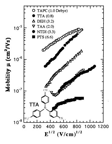
by virtue of their relatively small dipole moments, are insensitive to the dipolar disorder due to the chromophores, thus restoring most of the mobility reduction from addition of 25 wt. % of the highly polar EHDNPB chromophore.
