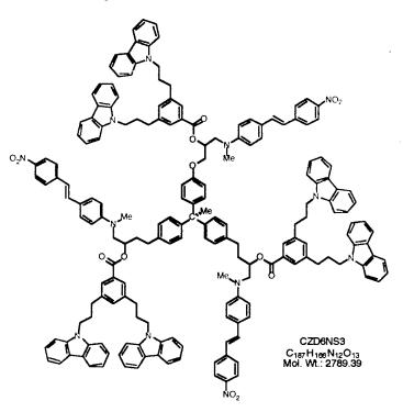
and environment so that redox potentials and photoionization energies can be adjusted without increasing disorder. For example, the electron-withdrawing group of a hole transport agent can be presented to the outside of the dendrimer structure while the remainder of the molecule is "protected" nearer the molecular core.
