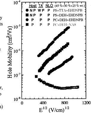
styrene (PS) host and using a weakly polar transport agent tri-p-tolylamine (TTA), even in the presence of the even more polar chromophore 2,5-dimethyl-4-(p-nitrophenylazo)phenol (ENDNPB). This composition shows a 300-fold improvement over the prototypical composi-
