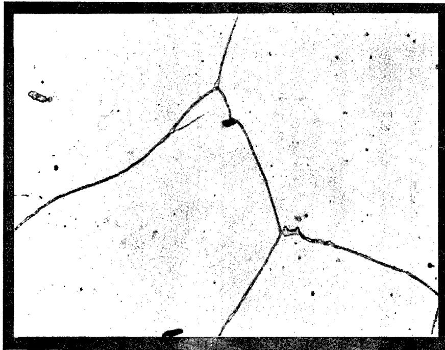
Test 7-1, \Delta\dot{\epsilon}_t = 2.08\% , \dot{\epsilon}_t = 4.2 \times 10^{-3} \text{ sec}^{-1} (Neg. 10138)
