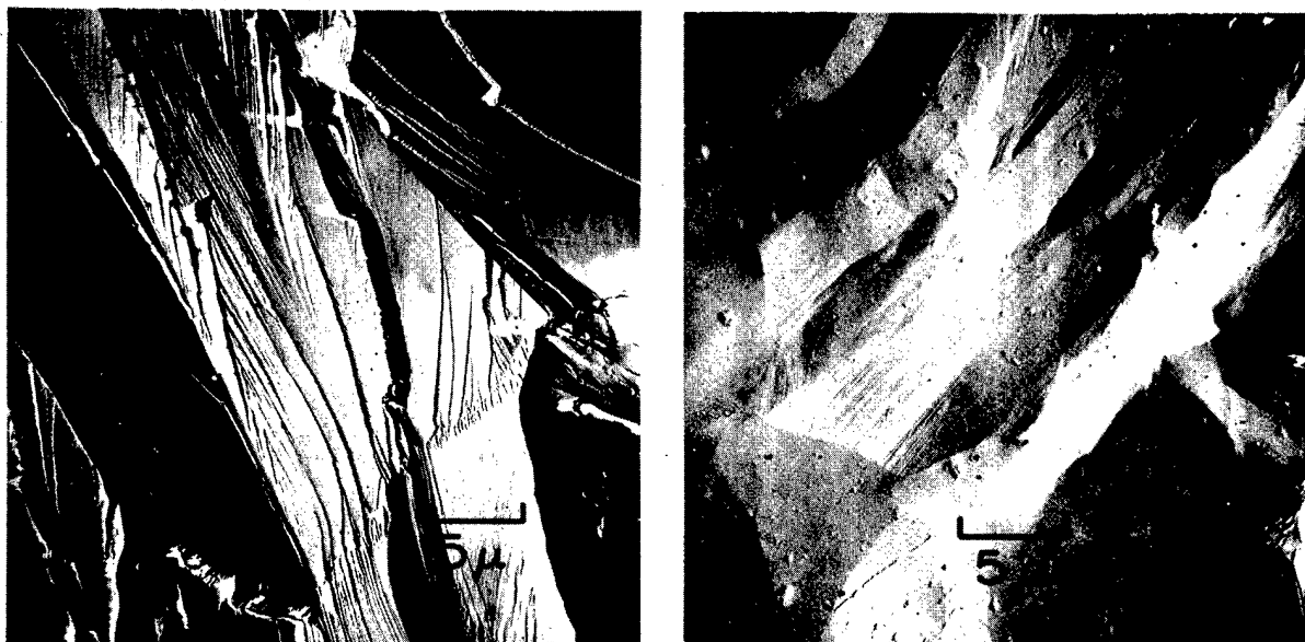
Fig. 1.21 — Electron fractographs of arc-cast tungsten. (a) Transgranular fracture in specimen tested at 2000°C and 2.11 kg/mm 2 . (b) Grain boundary surface in specimen tested at 1600°C and 4.22 kg/mm 2 .
