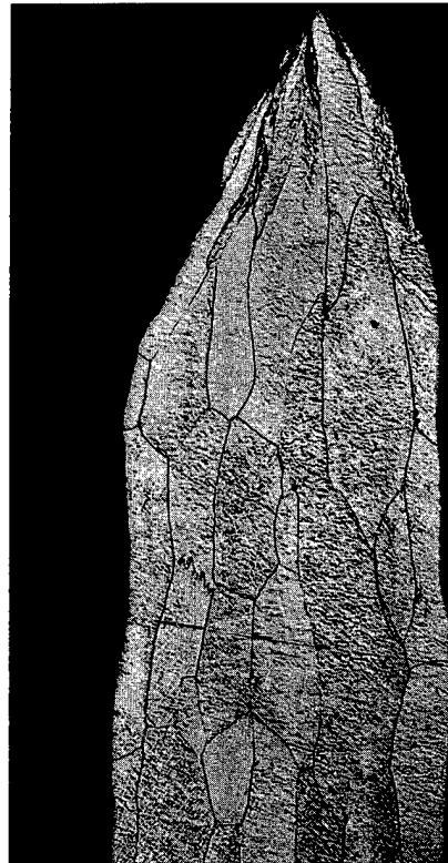
Irradiated ( 1.2 \times 10^{20} n/cm 2 ) plus 1600°C anneal for 1 hour (R-2255)
