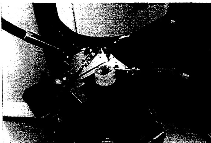
Figure 2. The microelectrochemical cell placed on a sample.
