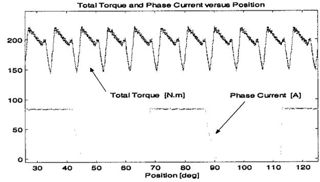
Fig.4 The total torque and flat-top phase current.
