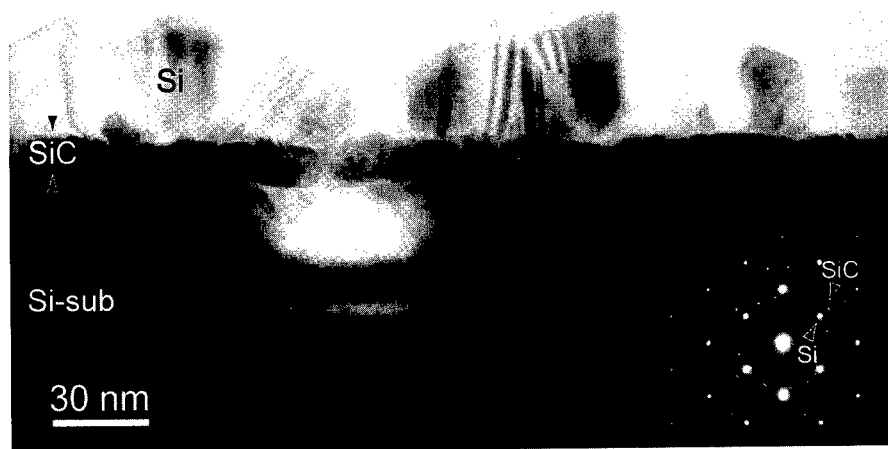
Fig. 1 XTEM bright-field image and diffraction pattern obtained from the sample grown by 3000 pulses of \text{CH}_3\text{SiH}_3 and \text{Si}_3\text{H}_8 .
