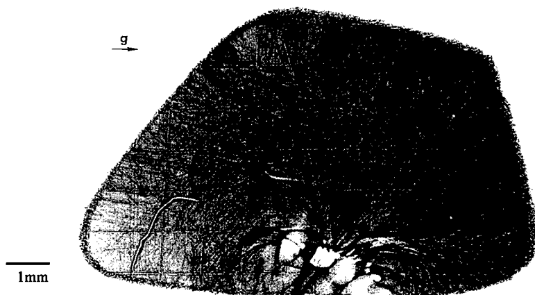
Figure 2. Back reflection topograph recorded from the 540R-SiC crystal ( g=00012960 , \lambda=1.24\text{\AA} ).
