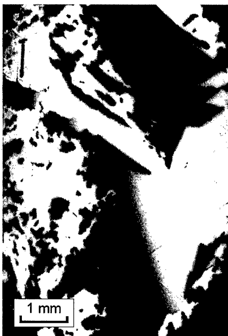
Fig.1. X-ray topograph of the 3C-SiC epilayer (Bragg's reflection (311)_{3C} , \text{CuK}_\alpha - radiation).
