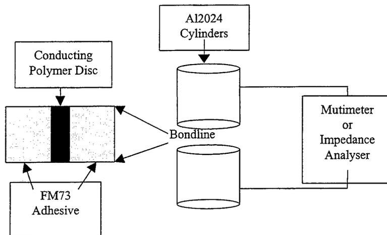
Figure 3a: Set up diagram of impedance and resistance measurements.
