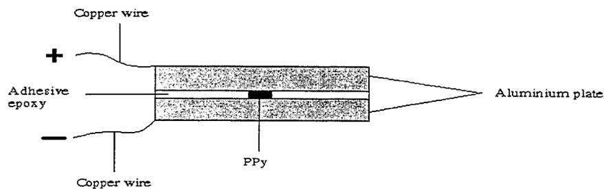
Figure 1: The structure of a cell with compressed PPy powder
