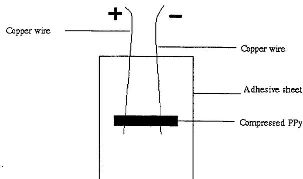
Figure 2: Sample for DC measurement.
