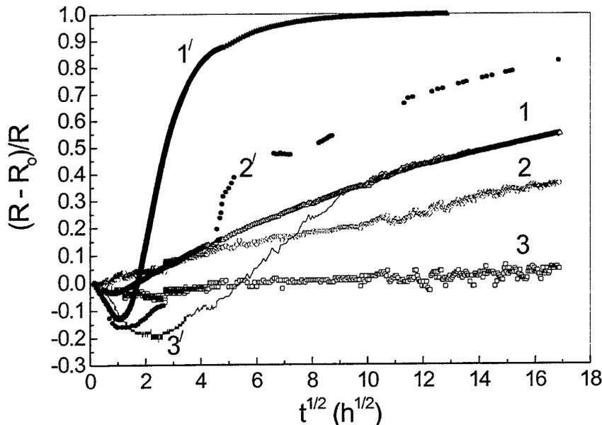
Figure 4: Resistivity increase by oxidative degradation of PPy powder at 50C . In a "dry" environment (7 % humidity): (1) PPy/0; (2) PPy/SSA and (3) PPy/AQ. In an environment of 95 % humidity: (1') PPy/0; (2') PPy/SSA and (3') PPy/AQ
