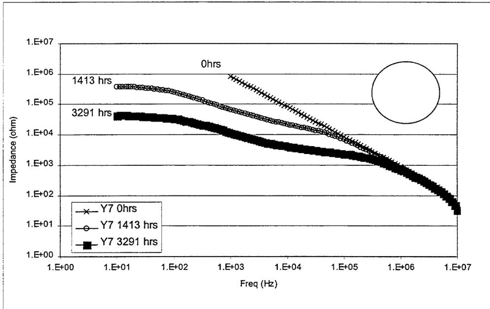
Figure 8a: Impedance plot across the bondline without PPy immersed in 0.001 M NaCl solution (sample Y7).
