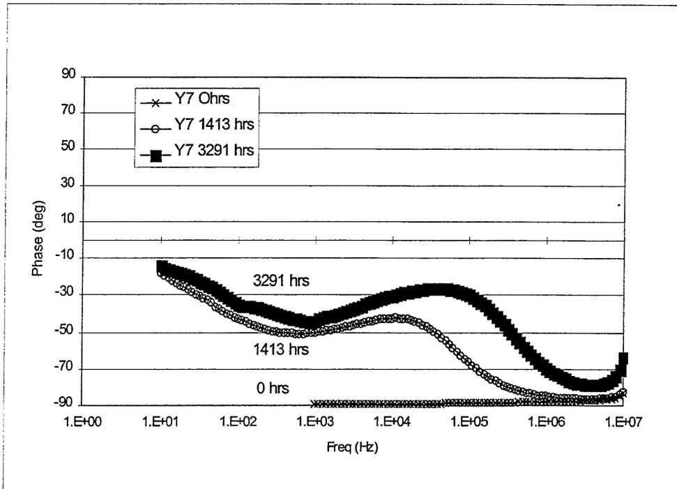
Figure 8b: Phase plot across the bondline without PPy immersed in 0.001 M NaCl solution (sample Y7).
