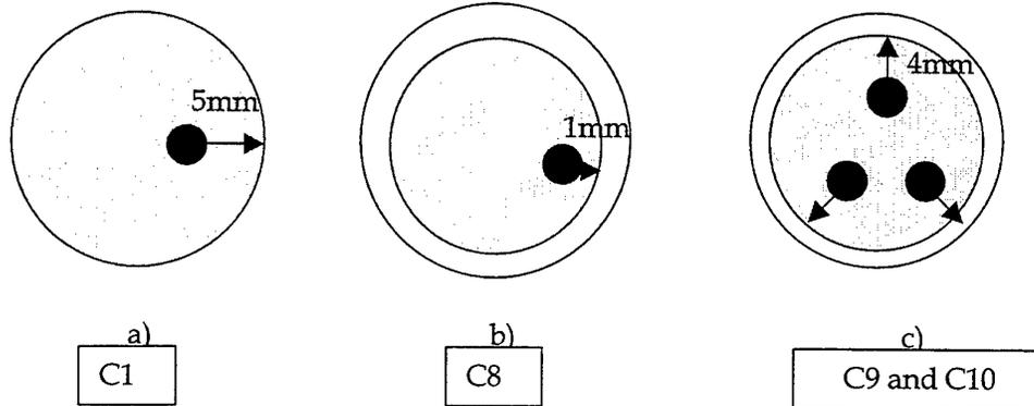
Figure 3b: Positions of the conducting polymer discs in the adhesive bondline, a) C1 with one disc 5mm from edge of adhesive, b) C8 with one disc 1mm from edge of adhesive, c) C9 and C10 with 3 discs at 4mm from edge of adhesive. (Note that in C8-C10 the adhesive was cut 1mm from edge of adherend to prevent overflow of the adhesive across the bondline).
