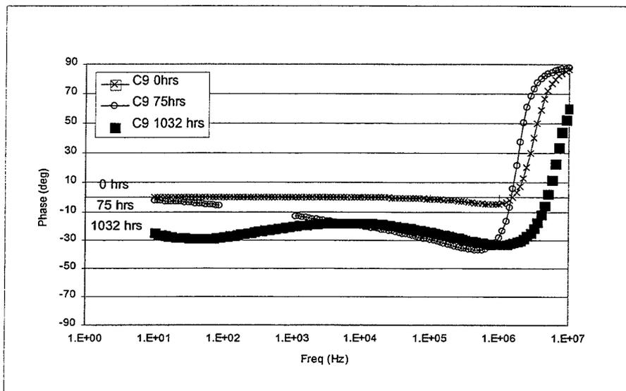
Figure 10b: Phase plot across the bondline with three PPy disc (5 mm diameter) immersed in 0.001 M NaCl solution (sample C9).
