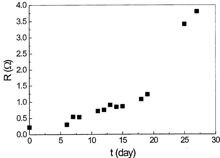
Figure 7: Increase in resistance  $R$  in contact with water of PPy powder.
