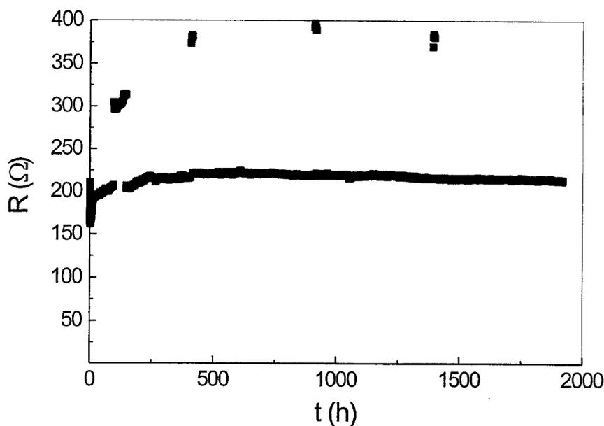
Figure 5: Resistivity of a compressed PPy/SSA powder embedded in the bondline and aged at 100°C
