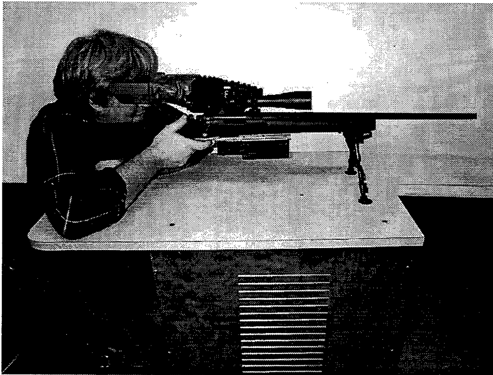
Figure 6. A Remington 700 Sniper Rifle With the IRT Being Fired From a Shoulder Mount.
