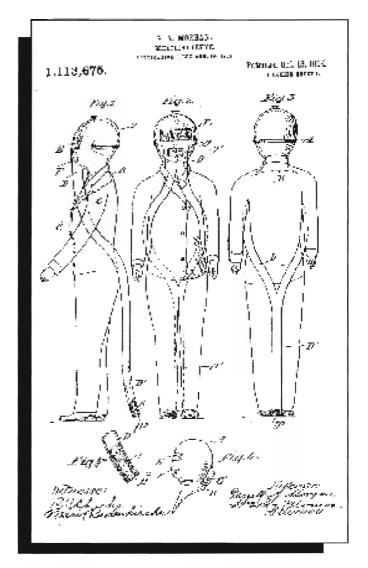
Garrett A. Morgan, of Cleveland, OH, patented a Breathing Device in 1906 designed for fireman, engineers, chemists, and anyone else *obliged to breath noxious fumes or dust*. The hood was made of rubber cloth or asbestos cloth. A long tube provided cleaner floor air to the mask or could be elevated in situations where the noxious fumes were heavier than air. One unique design was the use of *ear trumpets* in the mask to amplify sounds.
