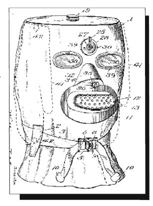
Charles E. Chapin and Arthur A. Sherman patented a Respiratory Apparatus for Firemen or Others in 1904. Two large air cylinders and a smaller emergency cylinder worn on the back provided fresh air to protect against smoke and noxious gases. The backpack included a place to attach an auxiliary mask for a rescued individual.
