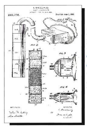
Samuel Danielewicz, of San Francisco, CA, patented a Filtrative Inhaler in 1909 that included a charcoal canister. The canister consisted of raw cotton saturated with glycerin alternating with pulverized charcoal.
