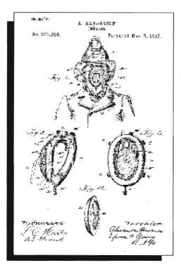
In 1897, Alexander Henderson, of Kansas City, MO, patented a cup mask to protect the wearer from smoke or other impurities in the air, such as arise in cement manufacture, working in acids, or fumes arising from ammonia when working in coldstorage and manufacturing artificial ice. The facepiece was made of rubber and three layers of different materials (wool, silk, and felt) provided the filtering. The silk was treated with glycerin (for smokes), ammonia (for
