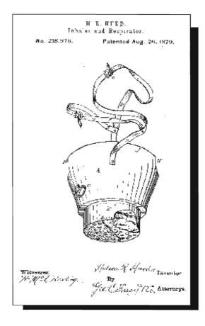
In 1889, Hutson R. Hurd patented a Respirator for Firemen that included a fabric facepiece with windows and an exhaust valve on top of the mask. A long hose drew clean air from the floor level to the facepiece. One unique aspect of the mask was that the gastight seal was around the periphery of the mask and therefore the mask did not require any mouthpieces or nose clips.
