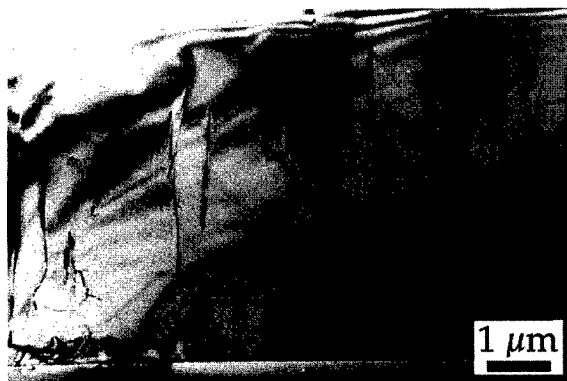
Fig. 1. Representative microstructure of a 5 \mu m thick MOCVD-grown GaN film on a sapphire substrate.
