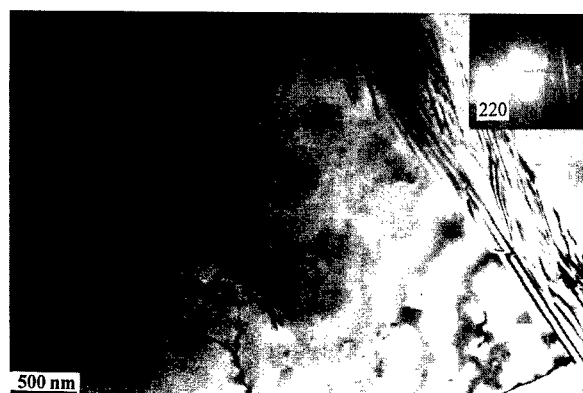
Fig. 6. Electron micrograph showing planar defects and dislocations formed in FZ-Si quenched from a molten state. The defect with a fringe contrast at the left is a stacking fault, and the band at the right is a \{1\ 1\ 1\} twin.
