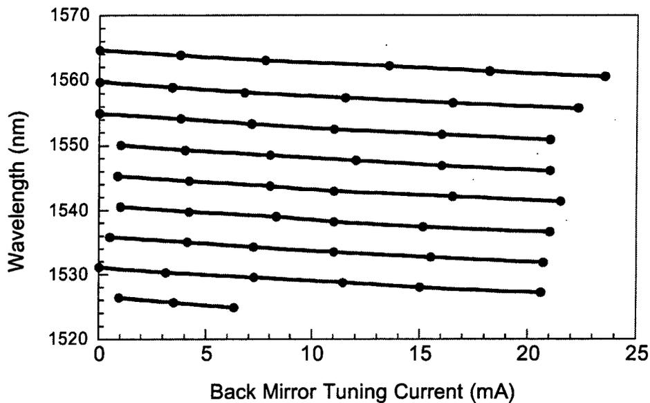
Figure 2-35 Buried Ridge SGDBR Back Mirror Tuning Currents
