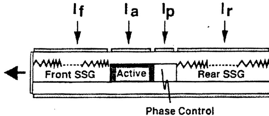
Figure 2-5 SSGDBR schematic cross section.
