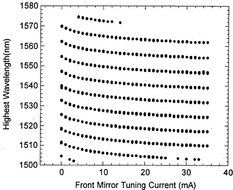
Figure 4a. Front mirror tuning curves for 72 nm quasi-continuous tuning range tested at 0.5 mA intervals from 0 to 35 mA. All points > 30 dB SMSR
