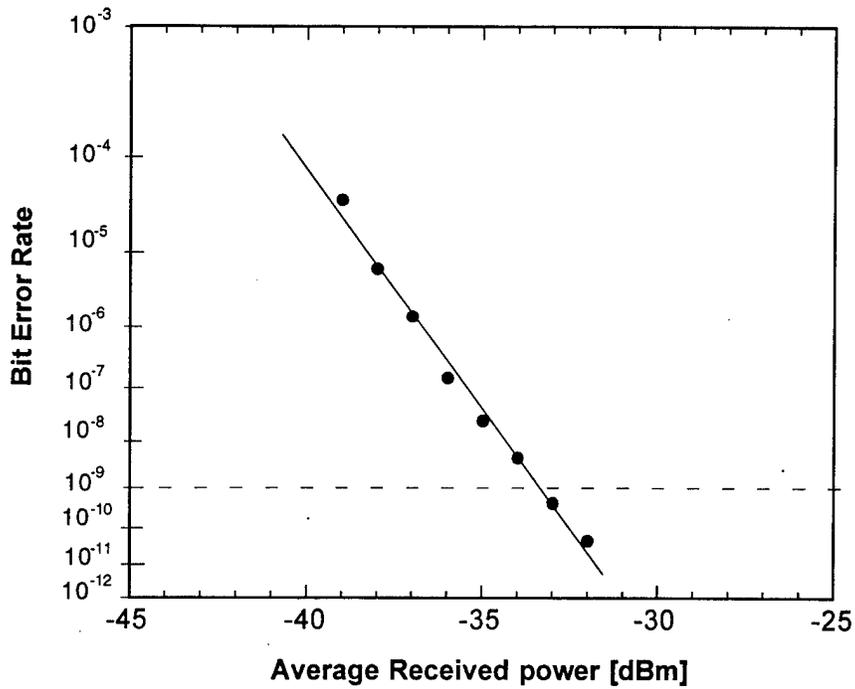
Figure 12. Back to Back Bit Error Rate Curves at 2.5 Gbit/s and  $2^{31}-1$  Pattern Length
