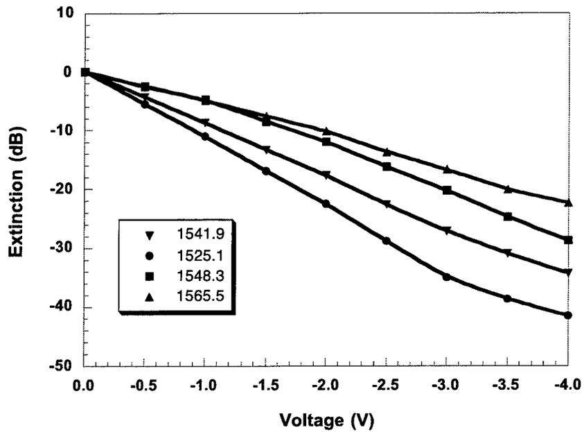
Figure 6-2 Modulator response curves for four wavelengths spanning more than 40 nm.
