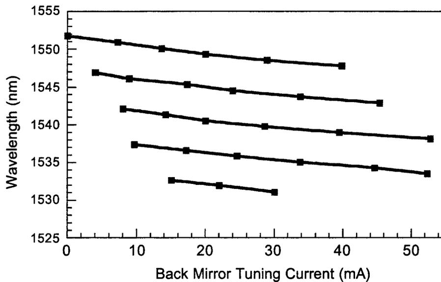
Figure 2-28 Back Mirror Tuning Current For Ridge Waveguide SGDBR
