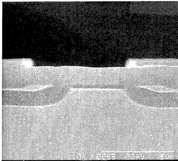
Figure 4-17 Buried heterostructure laser with blocking junction.
