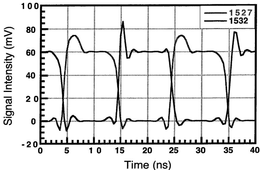
Figure 5-7 High speed wavelength switching waveforms
