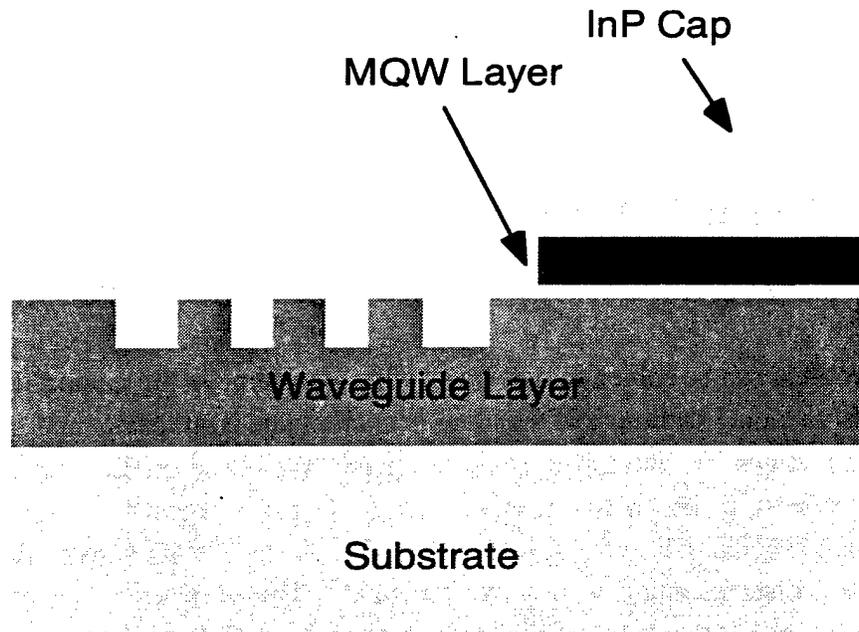
Figure 2-21 Waveguide structure with gratings etched directly into the top of the guide.
