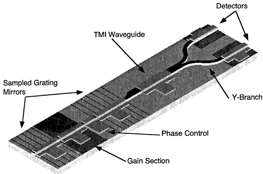
Figure 3-16 Ridge waveguide SGDBR with integrated TMI wavelength monitor.
