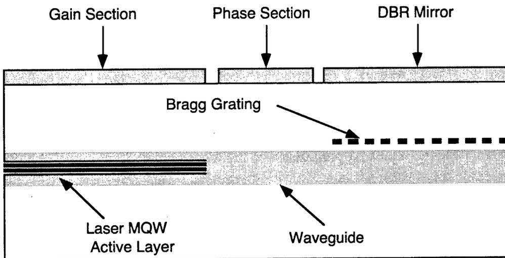
Figure 1-6 Tunable three section distributed Bragg reflector laser
