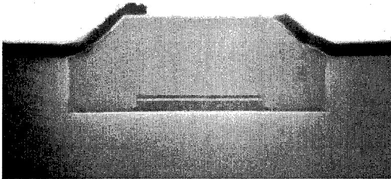
Figure 4-19 Dry etched buried ridge stripe laser.
