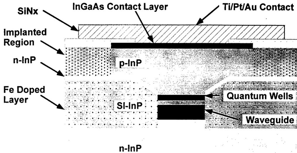
Figure 6. Buried heterostructure laser with Fe doped semi-insulating blocking junction.
