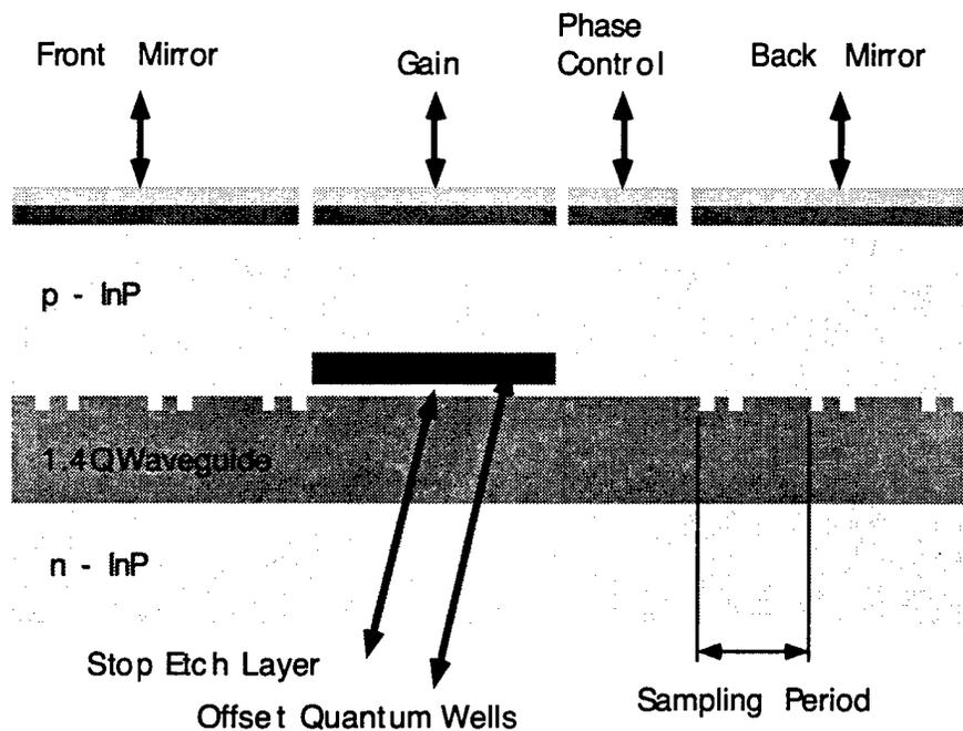
Figure 2-3 Cross section of SGDBR laser
