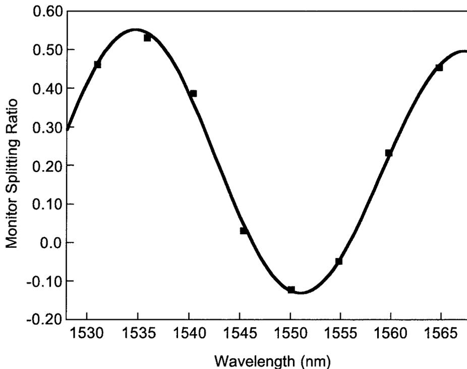
Figure 3-21 Monitor output signal for integrated buried heterostructure device.
