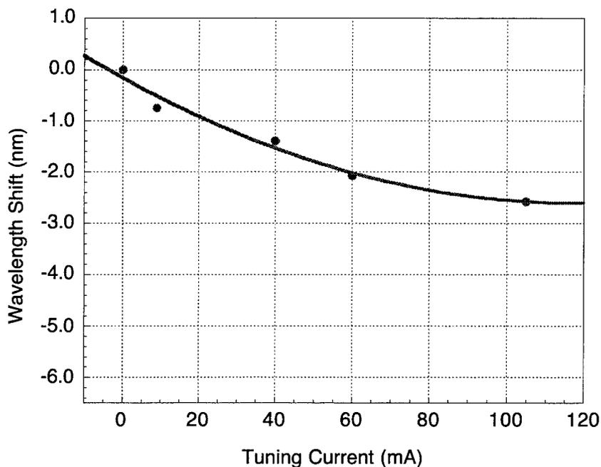
Figure 4-14 Wet etched DBR with 2.8 nm tuning range.
