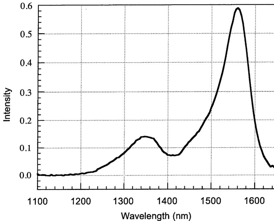
Figure 4-4 Photoluminescence spectrum for SGDBR base structure.
