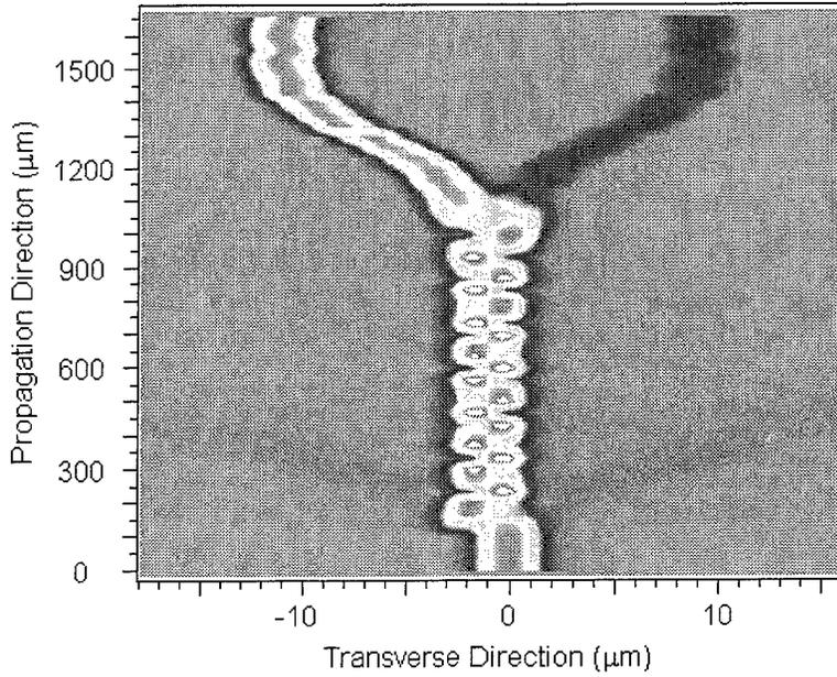
Figure 3-10 Ridge waveguide TMI BPM simulation
