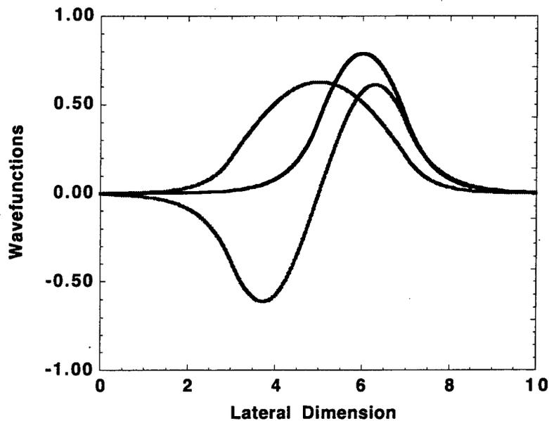
Figure 3-7 Superposition of offset input waveguide mode with the two lowest order TMI waveguide modes
