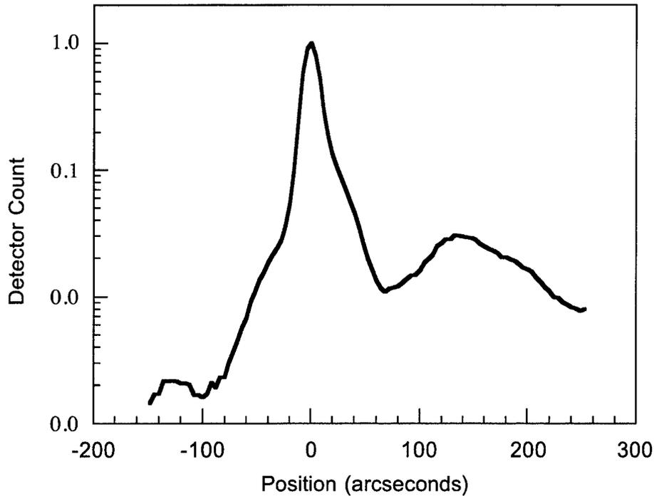
Figure 4-3 X-ray scan for slightly mismatched 1.4Q layer.
