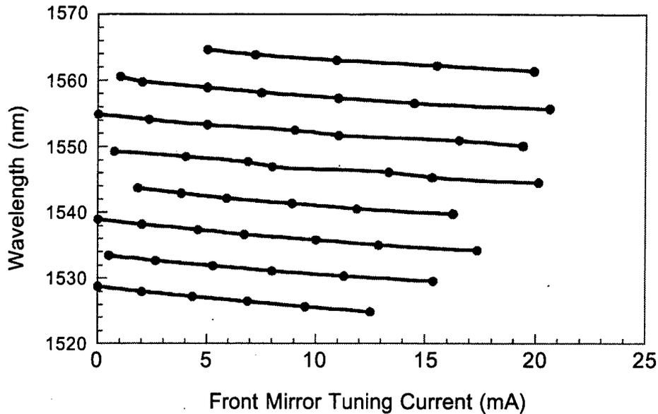
Figure 2-36 Buried Ridge SGDBR Front Mirror Tuning Currents
