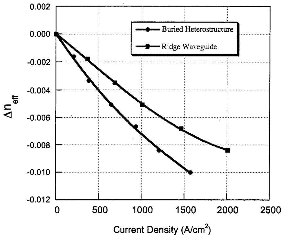
Figure 2-23 Comparison of index change vs. current density for ridge waveguide and buried heterostructure SGDBR mirrors.
