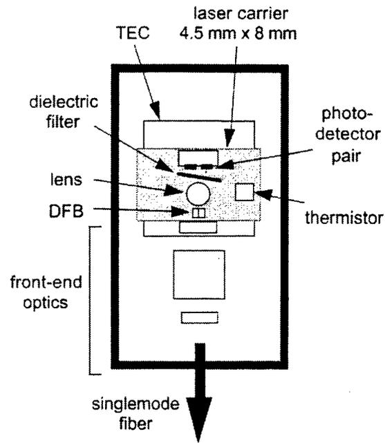
Figure 1-7 Laser with integrated wavelength monitor.
