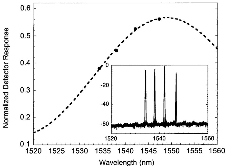
Figure 3-18 Wavelength response for integrated device using calibrated response curve. Laser spectra shown in inset.
