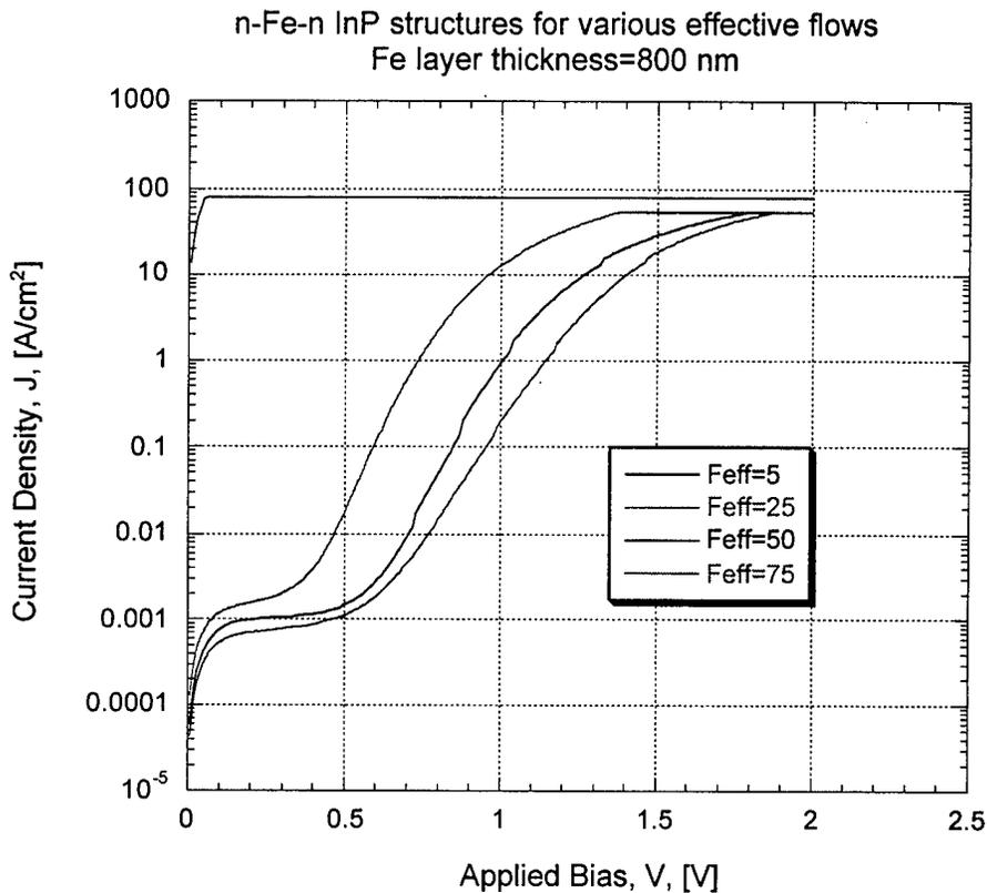
Figure 5. Resistivity for n-Fe-n InP structures grown with a variety of effective dopant flow rates. (3000Å n-type/10000Å Fe-SI/5000Å n-type).
