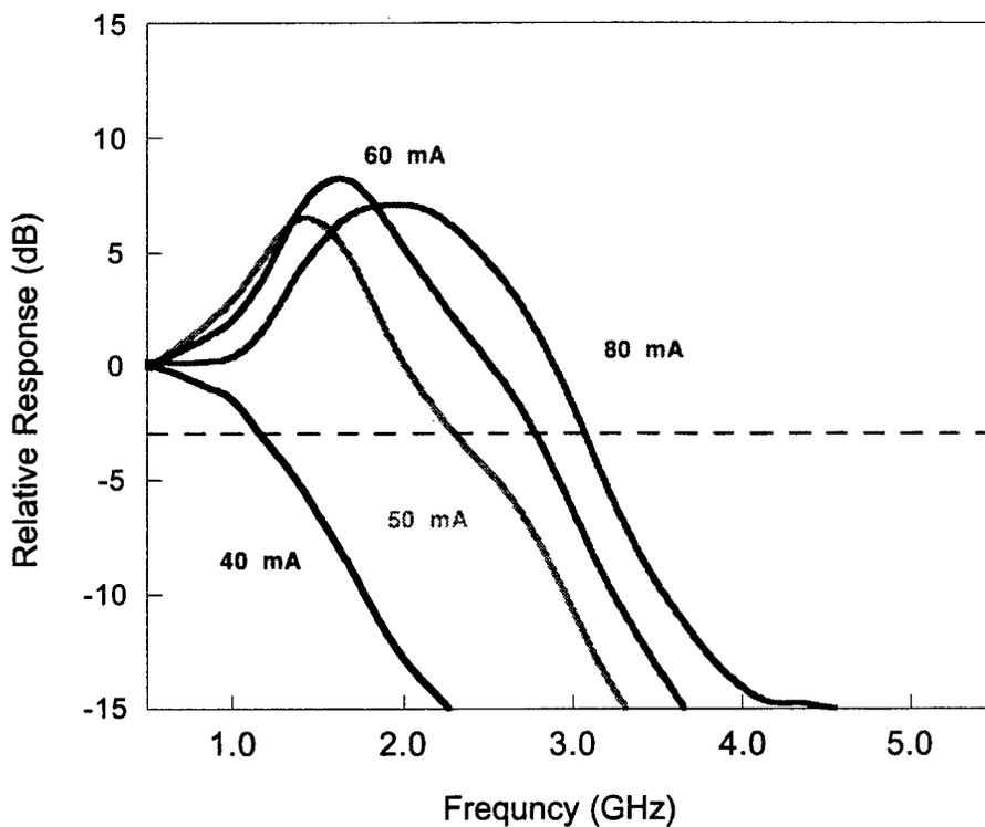
Figure 2-30 Modulation Bandwidth for Ridge Waveguide SGDBR at four different gain current levels.
