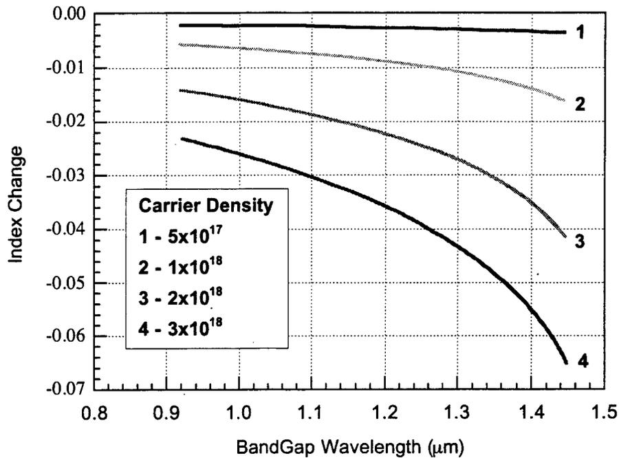
Figure 2-18 Index tuning as a function of bandgap wavelength for four different carrier densities at a wavelength of 1.56  $\mu\text{m}$ .
