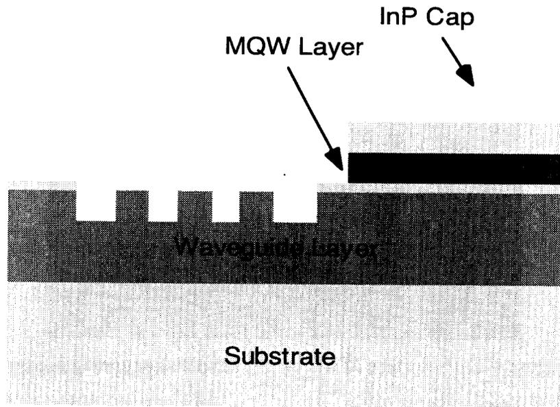
Figure 4-12 Base structure with dry etched gratings
