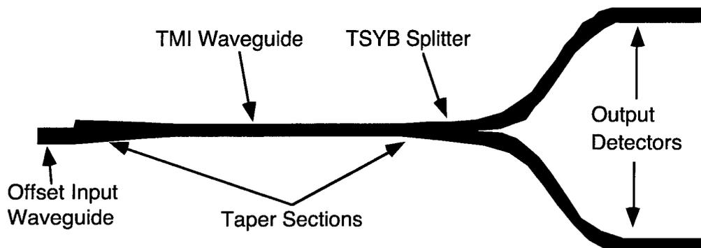
Figure 3-9 Schematic of Two Mode Interference wavelength monitor.
