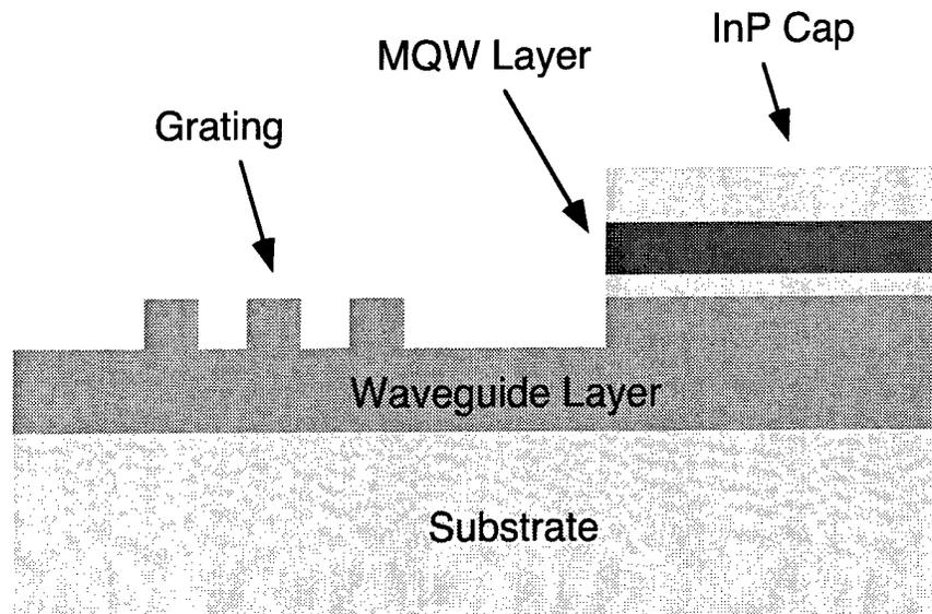
Figure 4-10 Base structure with wet etched gratings.
