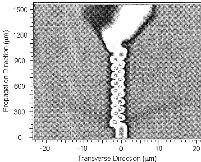
Figure 3-12 Mode beating in wavelength monitor with tapered mode expander and segmented detectors.
