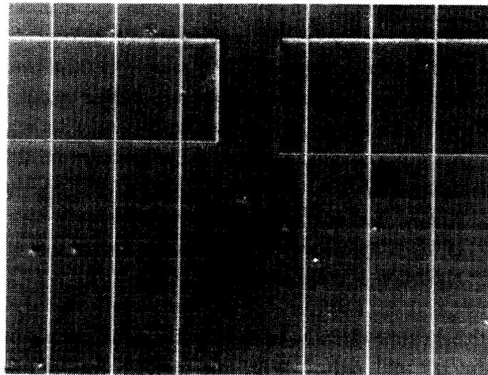
Figure 4-13 Surface of dry etched sample after grating regrowth.
