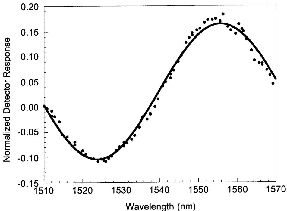
Figure 3-15 Normalized wavelength monitor response.
