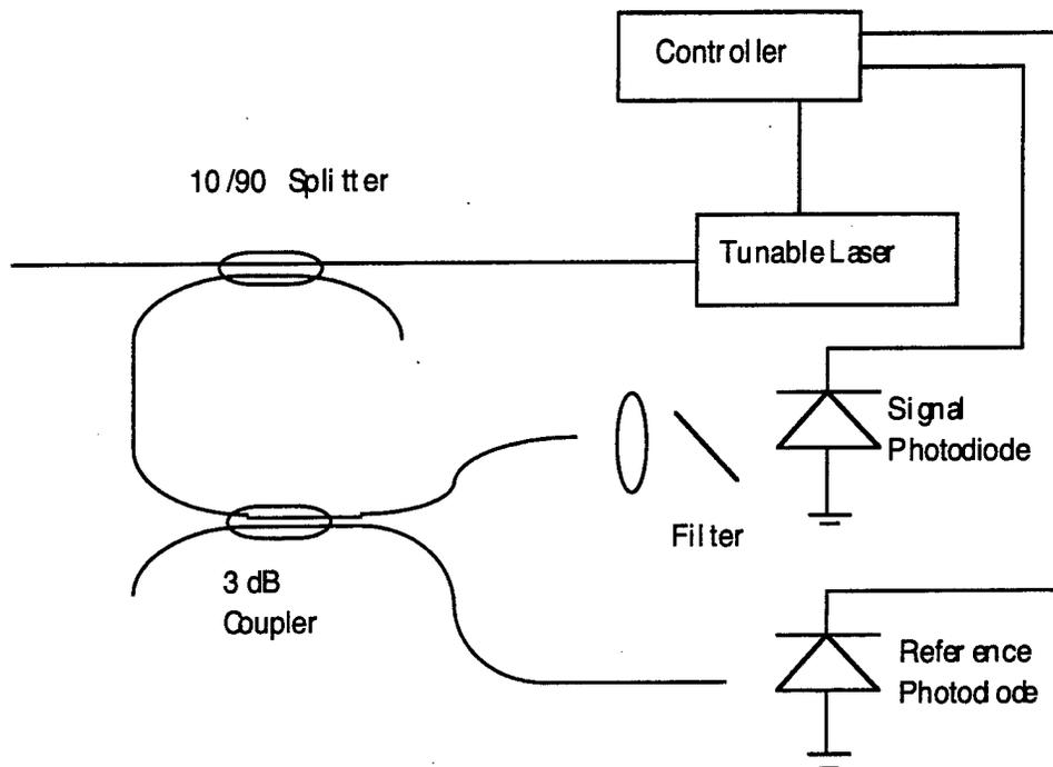
Figure 3-3 Ratiometric Wavelength Monitor and Control System For a Tunable Laser
