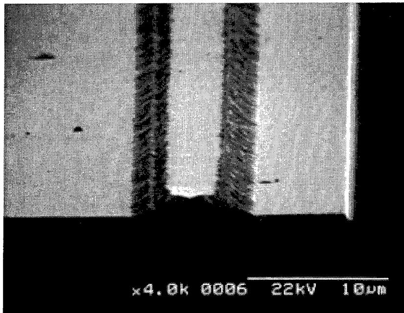
Figure 4-21 Close up of buried ridge with rough side walls.
