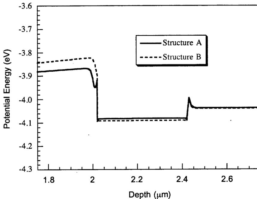
Figure 2-12 Conduction band edge showing barrier height for Structure A with an n doped stop etch layer and Structure B with an undoped stop etch layer.
