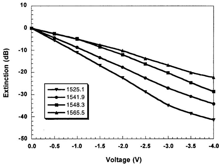
Figure 10. Extinction ratio vs. applied voltage for four different wavelengths.
