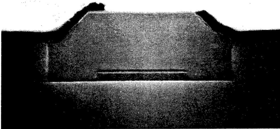
Figure 2-32 Stain etched SEM cross section of buried device.
