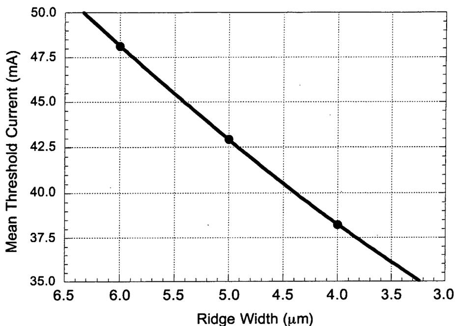
Figure 2-16 Threshold current dependence for SGDBR lasers with 4, 5 and 6  $\mu\text{m}$  ridge widths.
