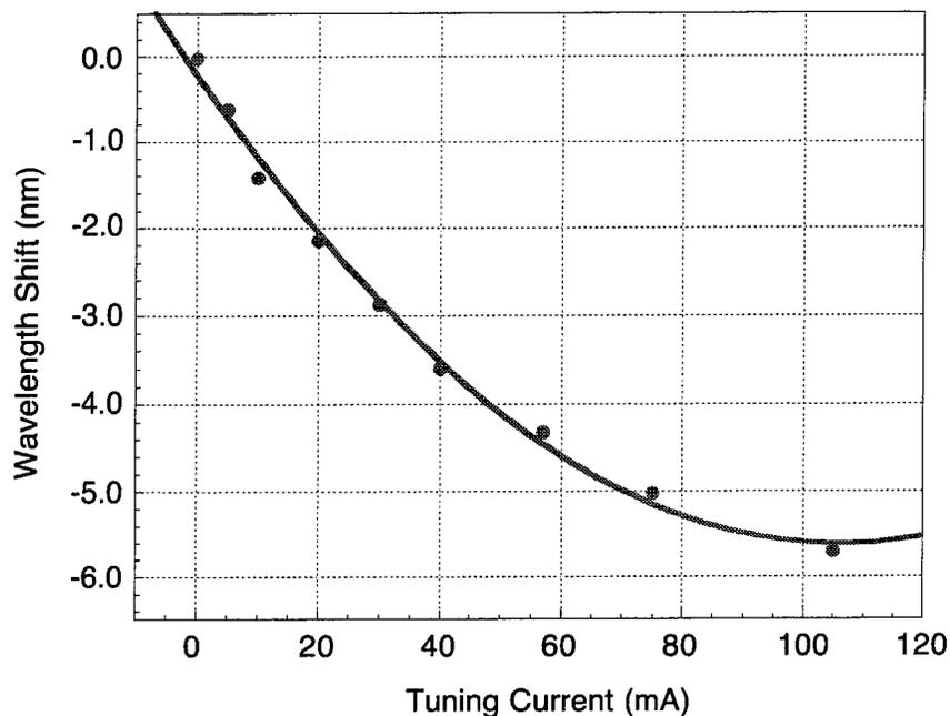
Figure 4-15 Dry etched DBR with 5.8 nm tuning range.
