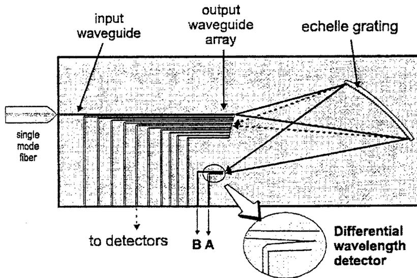
Figure 3-2 Waveguide mux with integrated wavelength locker
