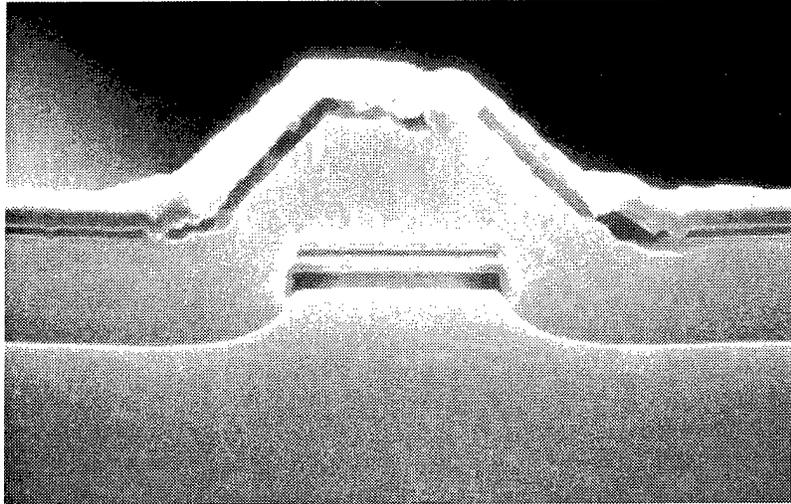
Figure 4-18 Wet etched buried ridge stripe laser.
