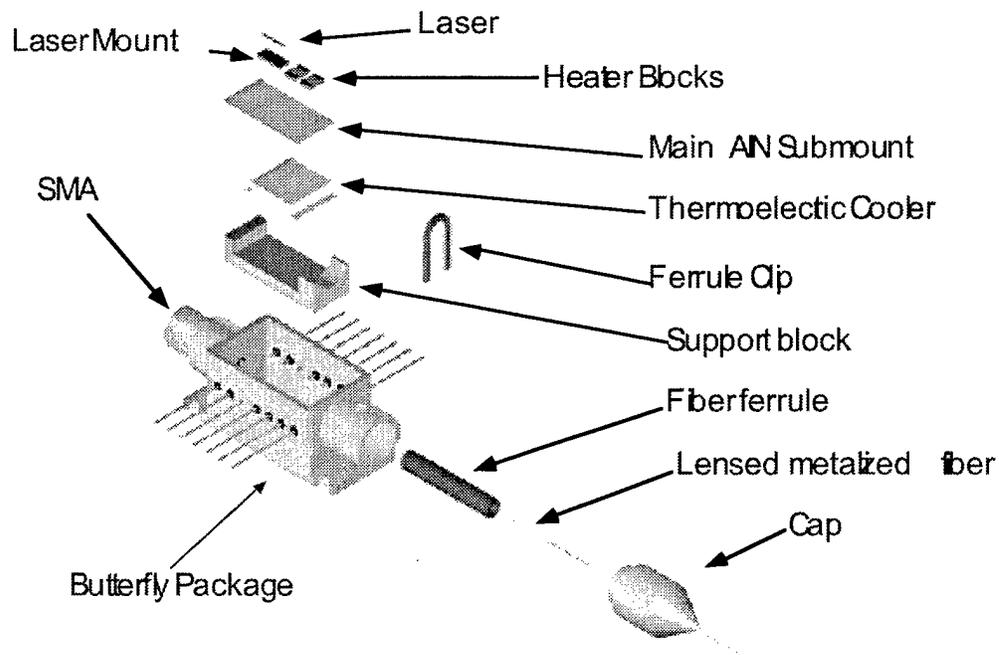
Figure 5-1 Laser package components.
