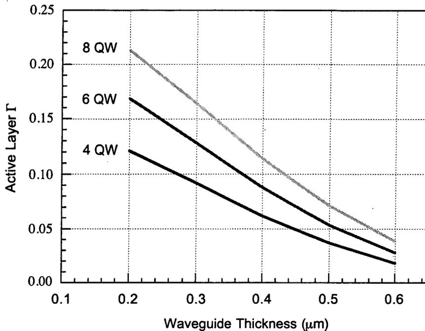
Figure 2-9 Confinement factor vs. waveguide thickness for active layers with 4, 6 and 8 quantum wells.
