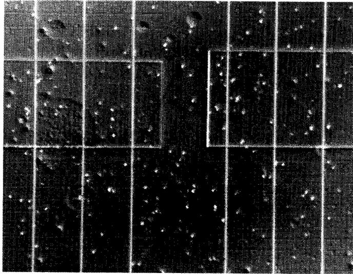
Figure 4-11 Surface of wet etched sample after grating regrowth.
