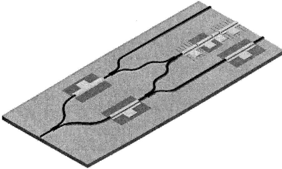
Figure 6-4 Proposed interferometric wavelength converter with integrated tunable laser source.
