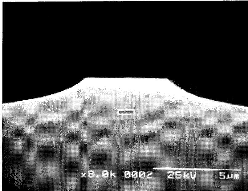
Figure 4-23 SEM cross section of low temperature regrowth showing enhanced lateral growth rate.
