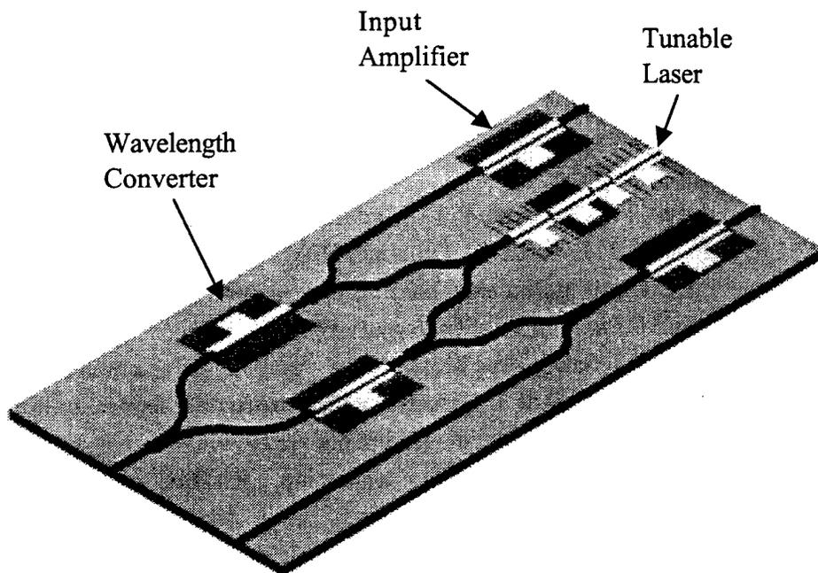
Figure 1-9 Interferometric wavelength converter with integrated tunable laser source.
