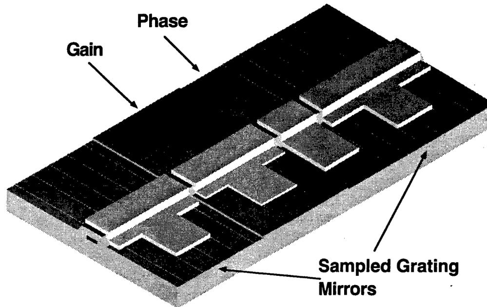
Figure 2-33 Buried heterostructure SGDBR laser schematic
