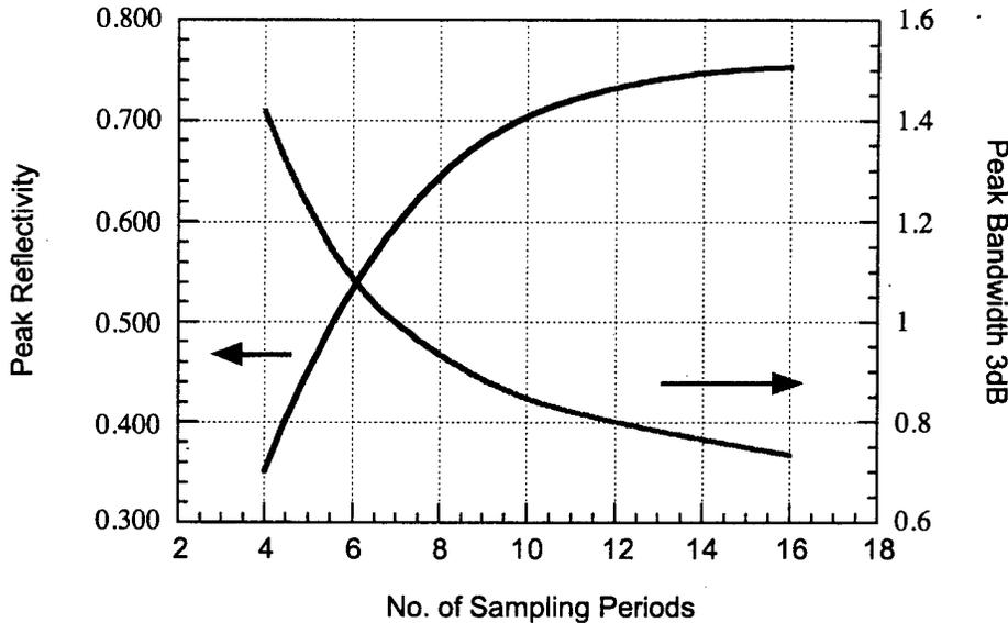
Figure 2-15 Reflectivity and bandwidth for the central peak of a sampled grating mirror vs. number of mirror periods.
