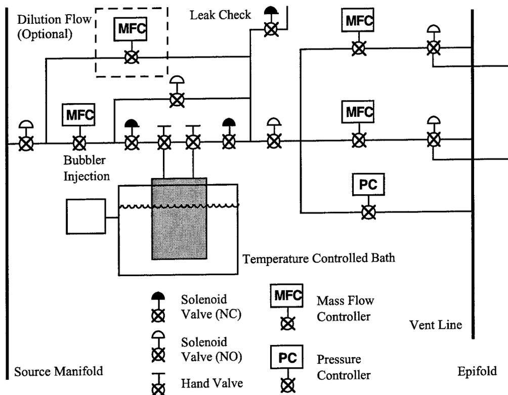
Figure 4-1 Source Bubbler Configuration
