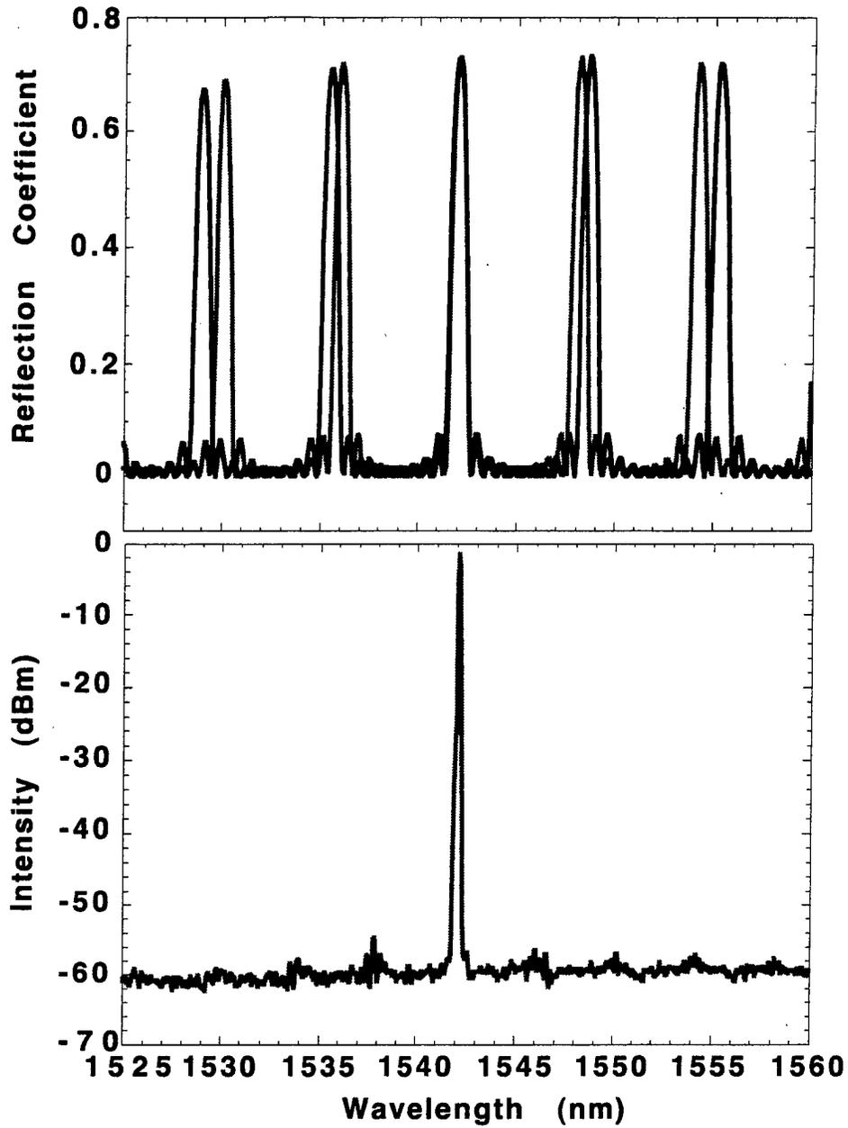
Figure 2-4 Superimposed sampled grating mirror reflection spectra and corresponding laser spectrum.
