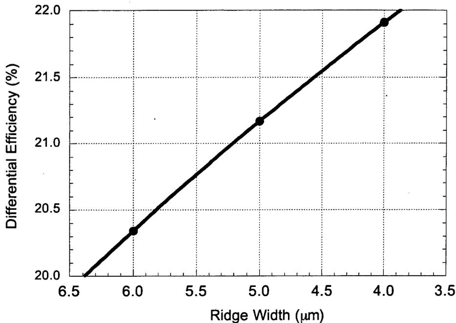
Figure 2-17  $\eta_d$  dependence for SGDBR lasers with 4, 5 and 6  $\mu\text{m}$  ridge widths.
