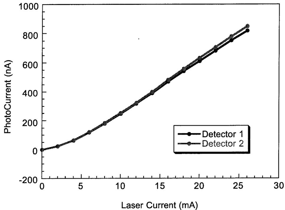
Figure 3-26 Monitor detector response for laser biased below the threshold current of 27 mA.
