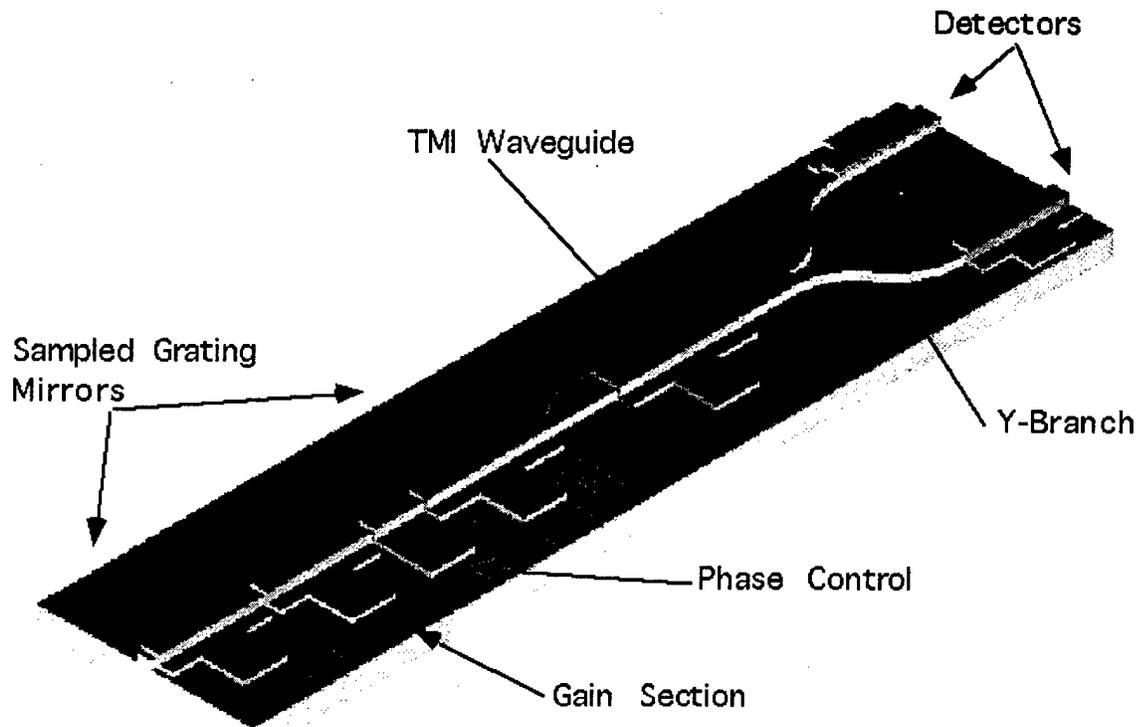
Figure 2. Integrated SGDBR and TMI wavelength Monitor
