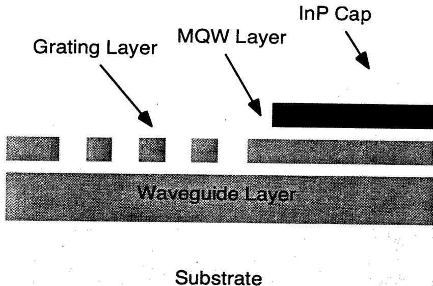
Figure 2-19 Waveguide structure with offset grating layer.
