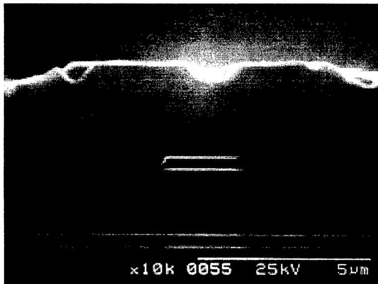
Figure 7. Scanning Electron Microscope cross section of SI-BRS laser.
