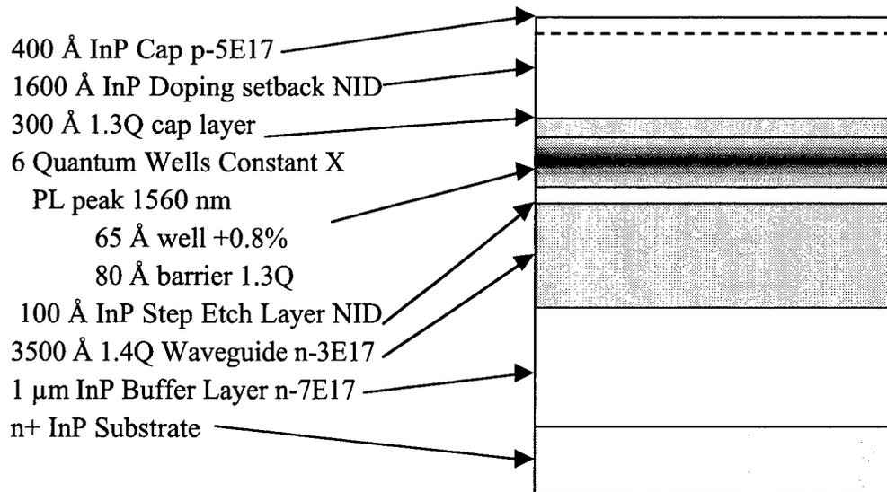
Figure 4-9 SGDBR base structure layer composition and doping
