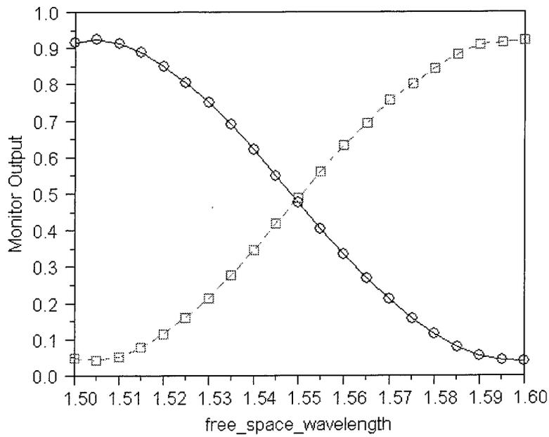
Figure 3-11 BPM simulation of TMI monitor splitting ratio for a wavelength scan from 1500 nm to 1600 nm
