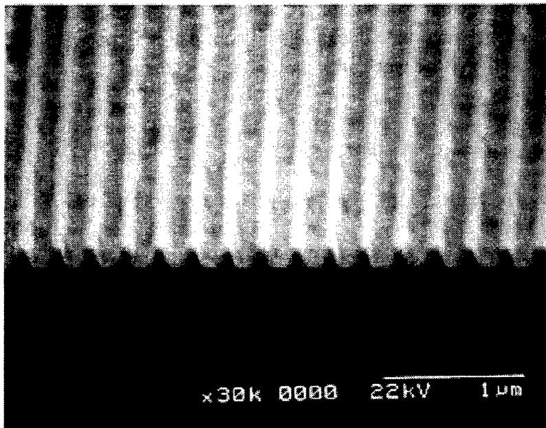
Figure 2-26 SEM Photo of dry etched gratings. Period is 240 nm and the etch depth is approximately  $1260 \text{ \AA}$ .
