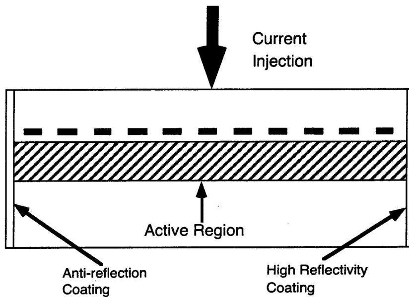
Figure 1-3 Distributed Feedback Laser Diode
