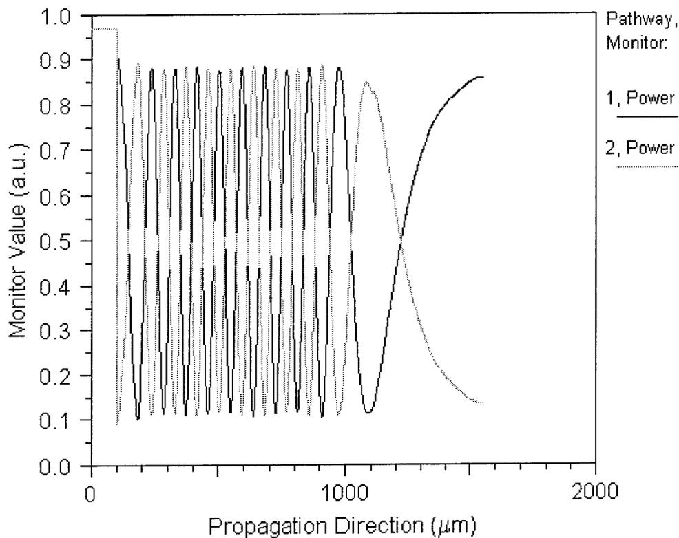
Figure 3-13 Coupled mode power as a function of distance along the TMI waveguide.
