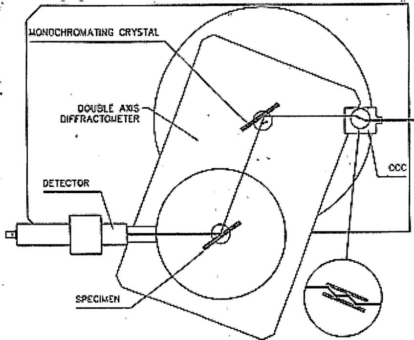
Figure 4-2 Double crystal x-ray diffractometer with channel cut collimator.
