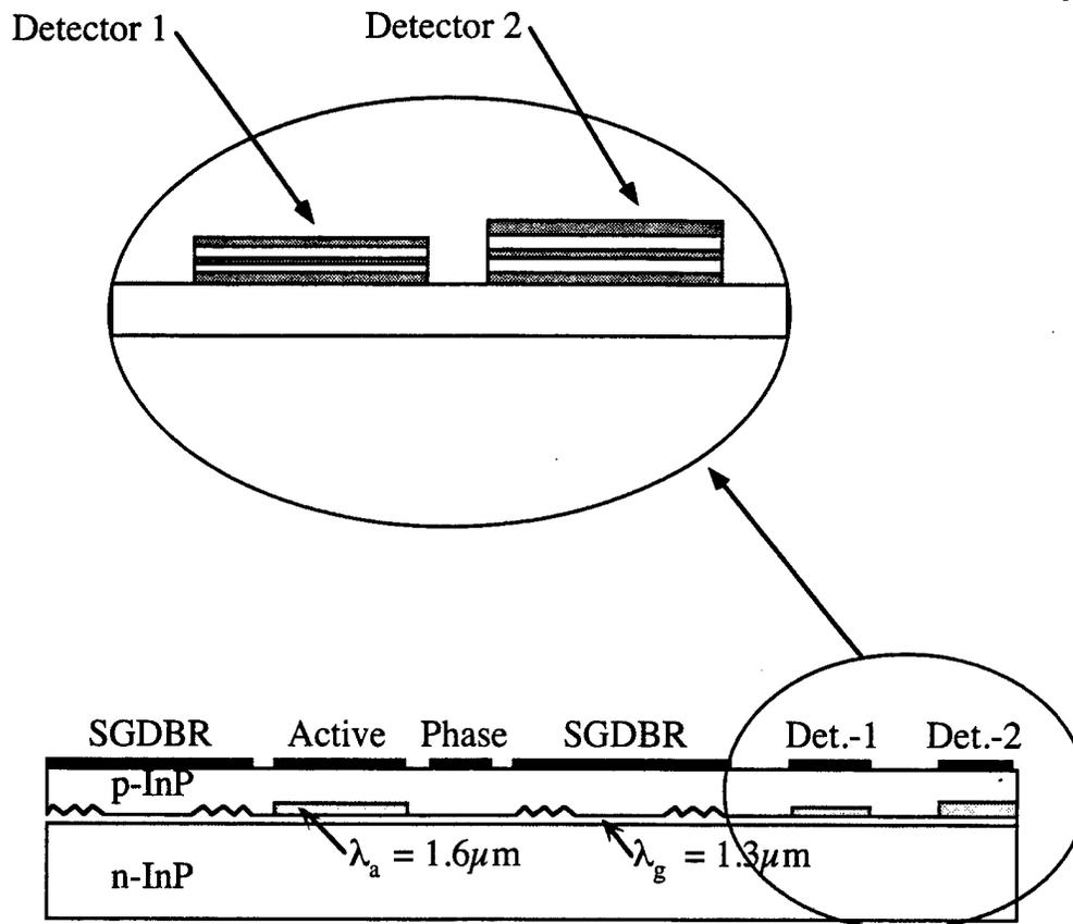
Figure 3-5 Dual Bandgap Detector Wavelength Monitor
