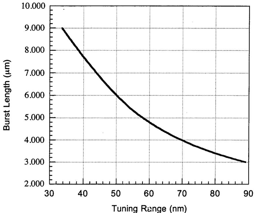
Figure 2-14 Optimum grating burst length vs. tuning range for a mirror with  $9 \text{ cm}^{-1}$  of loss and a coupling coefficient of  $450 \text{ cm}^{-1}$ .
