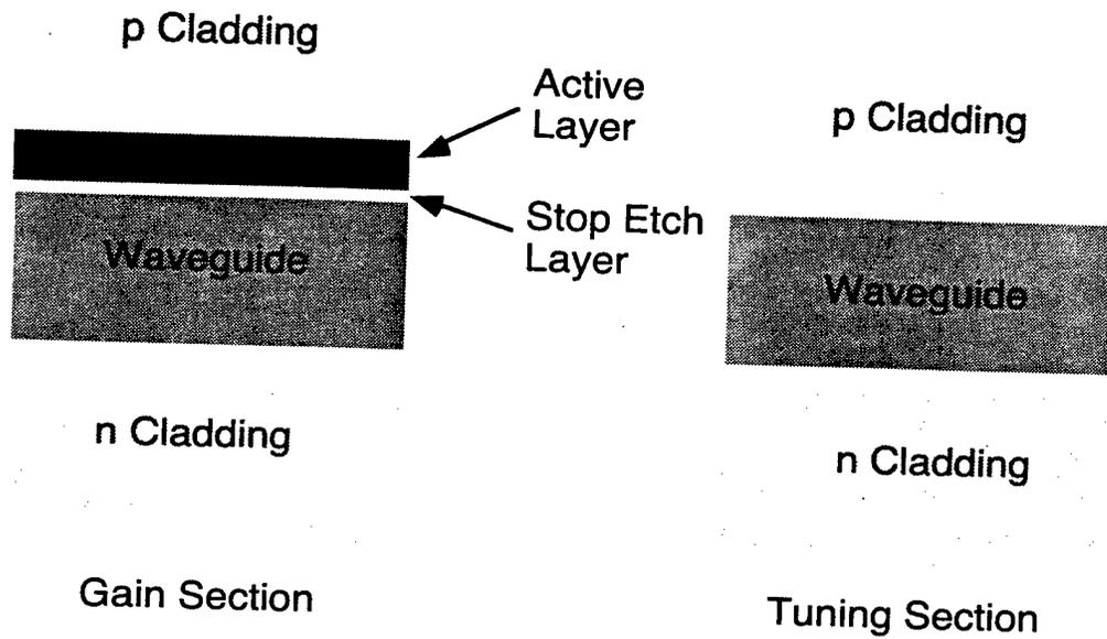
Figure 2-8 Waveguide Structure for Gain and Tuning Sections
