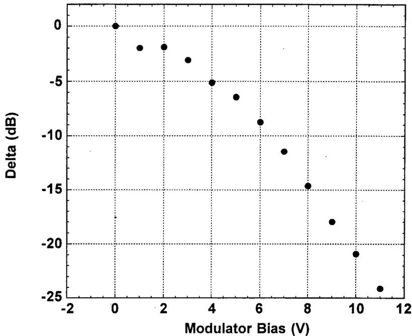
Figure 11. DC extinction curves for EA modulator at 1535 nm
