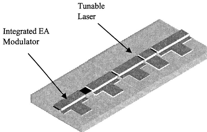
Figure 6-1 Tunable SGDBR laser with integrated modulator.
