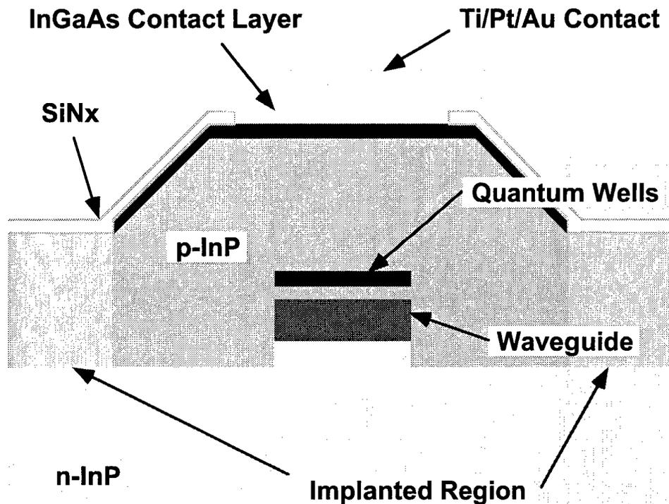
Figure 4-16 Cross section of buried ridge stripe laser.
