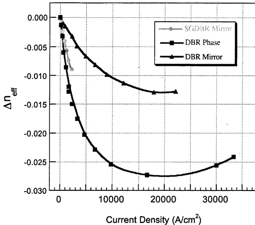
Figure 2-22 Tuning efficiency for ridge waveguide devices without a grating layer.
