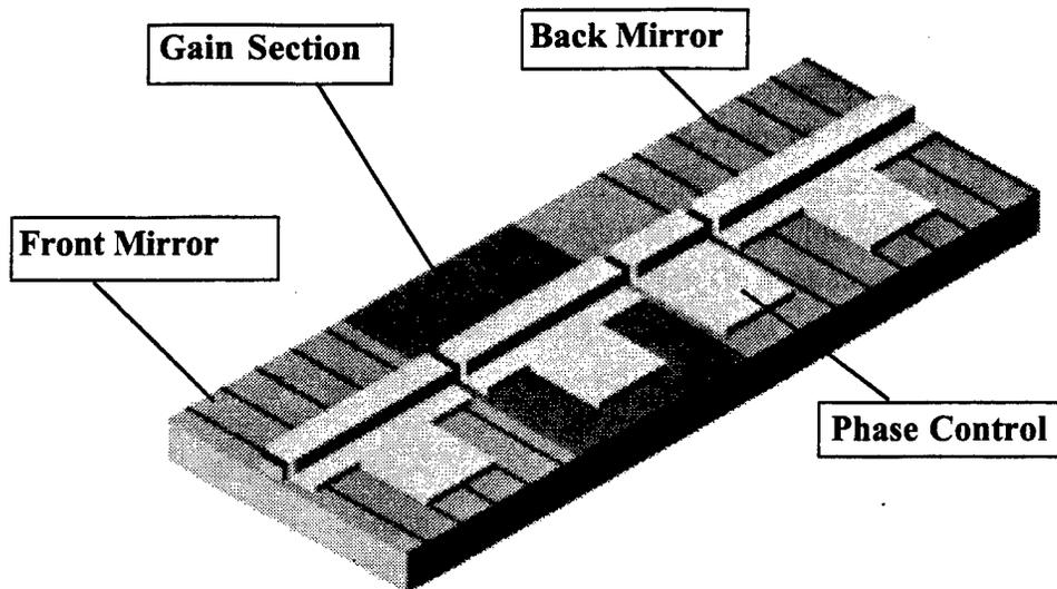
Figure 2-1 Widely tunable SGDBR Laser
