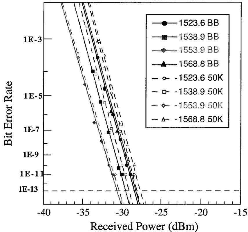
Figure 5-10 Bit error rate curves for back to back and 50 km transmission over standard single mode fiber at four widely spaced wavelengths.
