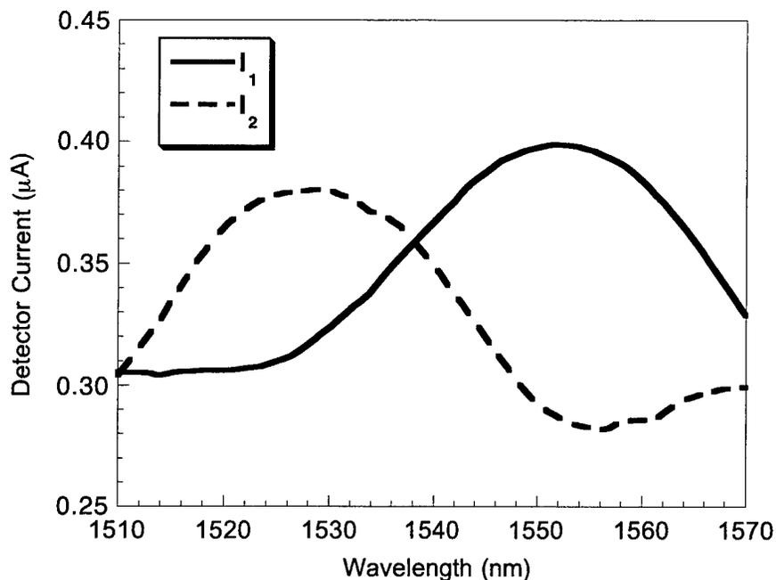
Figure 3-14 Detector response vs. wavelength for ridge waveguide wavelength monitor tested with external cavity tunable laser.
