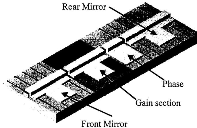
Figure 1 SGDBR Laser schematic
