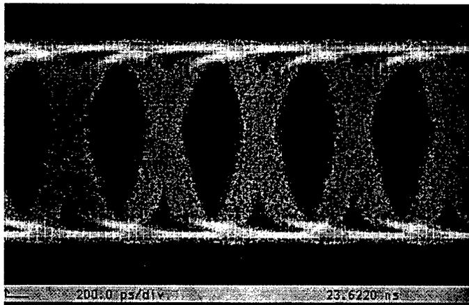
Figure 13. Eye Diagram at 2.488 Gbit/s Data Rate,  $2^{31}-1$  Pattern Length and  $1E-9$  Error Ratio
