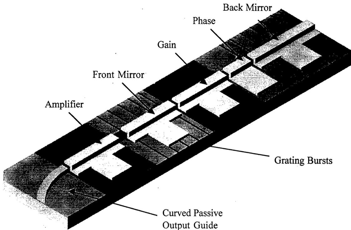
Figure 8. SGDBR laser with integrated semiconductor optical amplifier.
