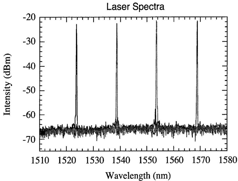
Figure 5-9 Superimposed laser spectra for the four transmission channels which are equally spaced 15 nm apart.
