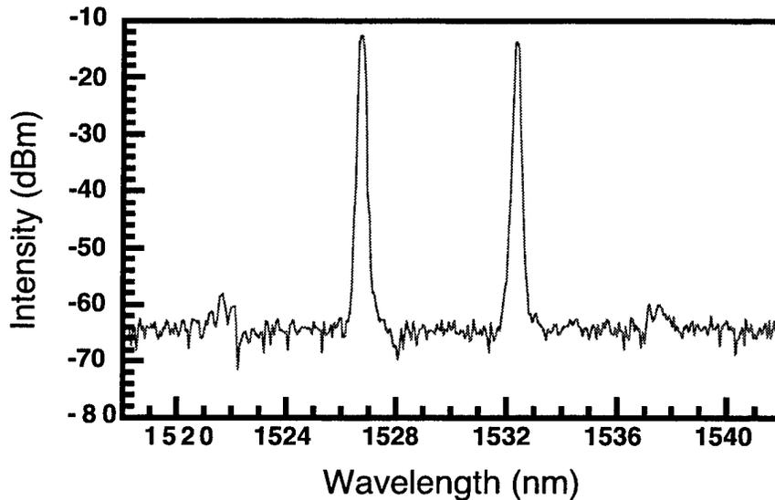
Figure 5-8 Spectrum under periodic wavelength switching
