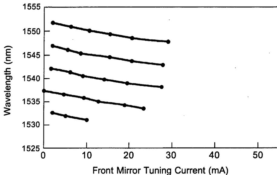
Figure 2-29 Front Mirror Tuning Current For Ridge Waveguide SGDBR
