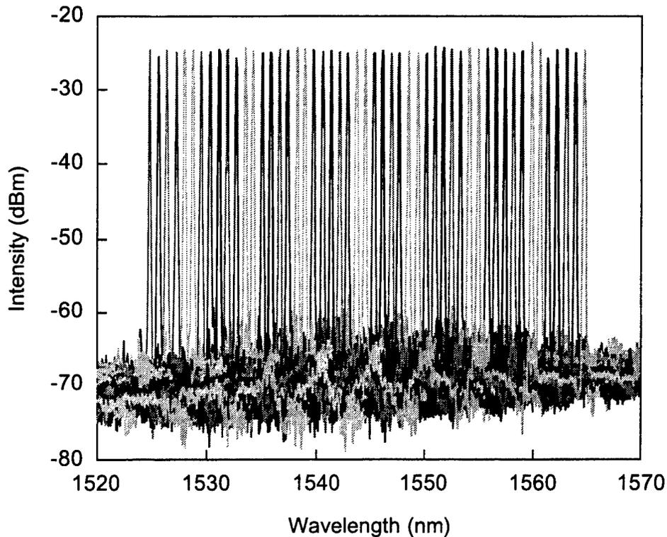
Figure 2-34 Buried heterostructure SGDBR tuning spectra showing 51 channels spaced at 100 GHz over a 40 nm tuning range
