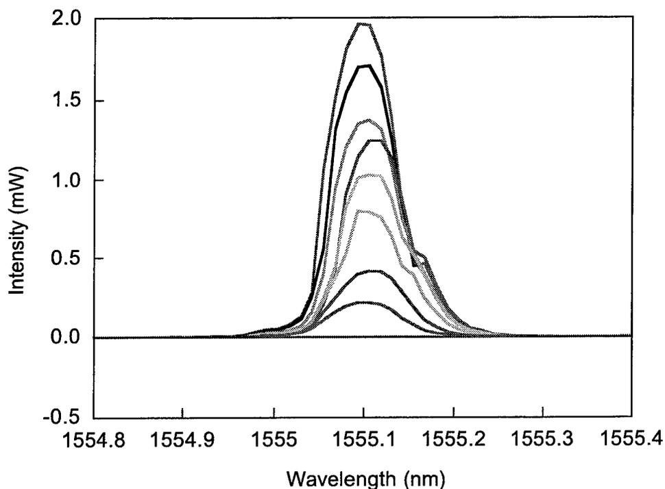
Figure 3-24 Laser spectra for constant wavelength test at 9 different bias levels from threshold to 65 mA.
