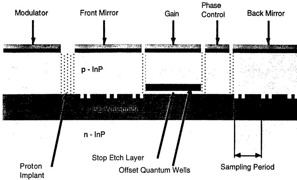
Figure 9. Cross Section of the Integrated Laser Modulator Device
