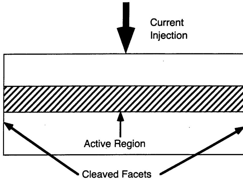
Figure 1-2 Fabry-Perot Laser Diode
