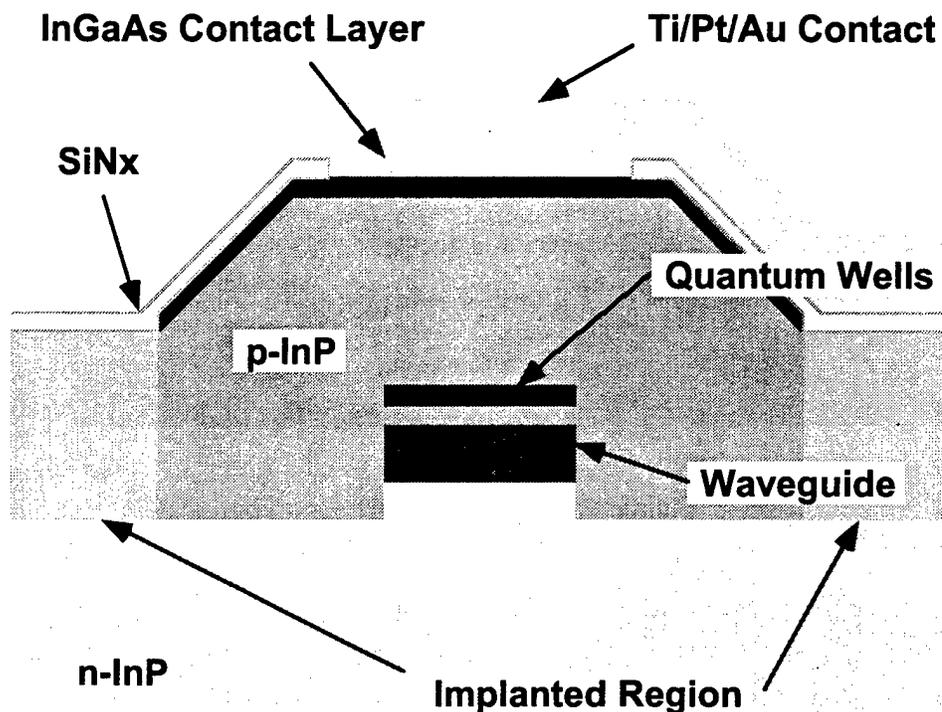
Figure 2-31 Buried Ridge Cross Section With Offset Active Region
