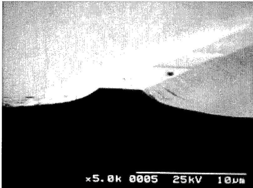
Figure 4-22 SEM of low temperature regrown buried heterostructure laser with smooth side walls.
