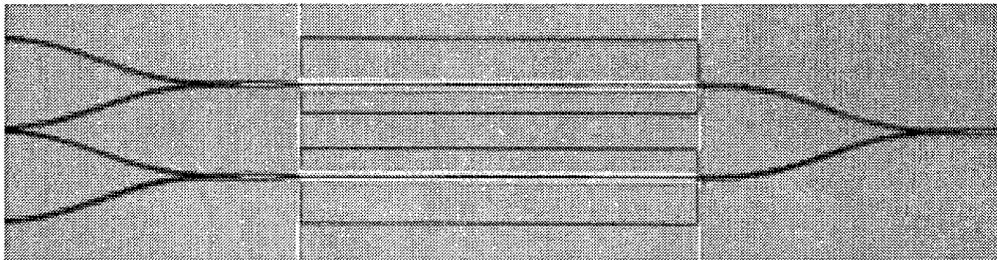
Figure 6-3 Die shot of interferometric wavelength converter with multi-mode interference splitters.
