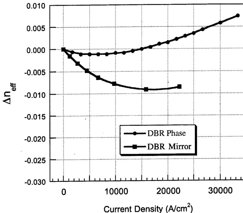
Figure 2-20 Comparison of the tuning efficiency for DBR phase sections and DBR mirror sections.
