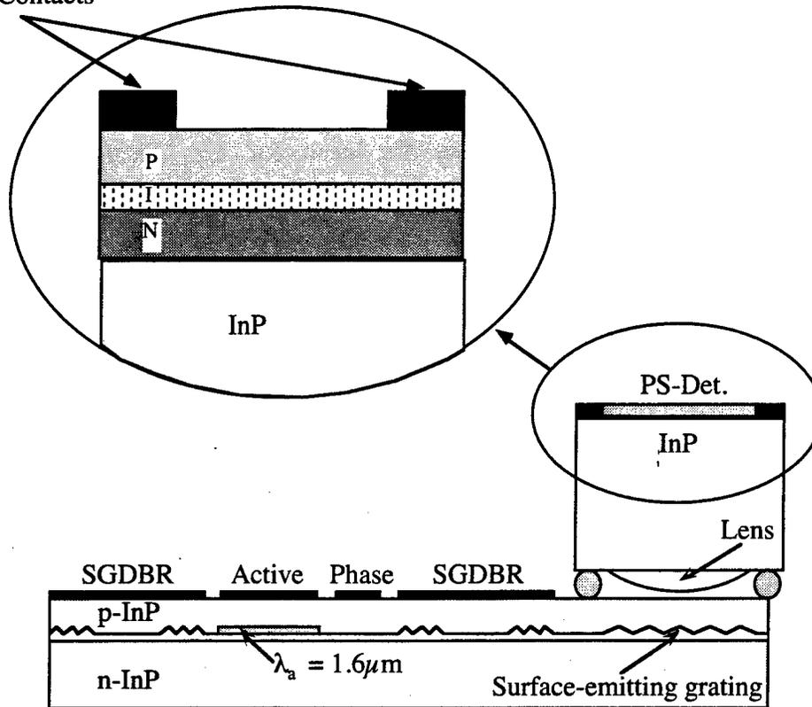
Figure 3-4 Surface Grating Coupled Wavelength Monitor
