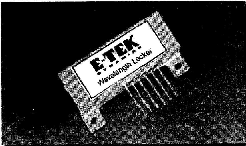
Figure 1-8 Commercial packaged wavelength locker
