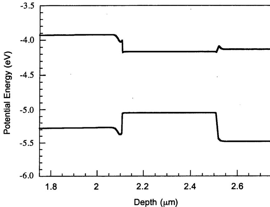
Figure 2-11 Passive section band diagram at a bias of 1.2 V.
