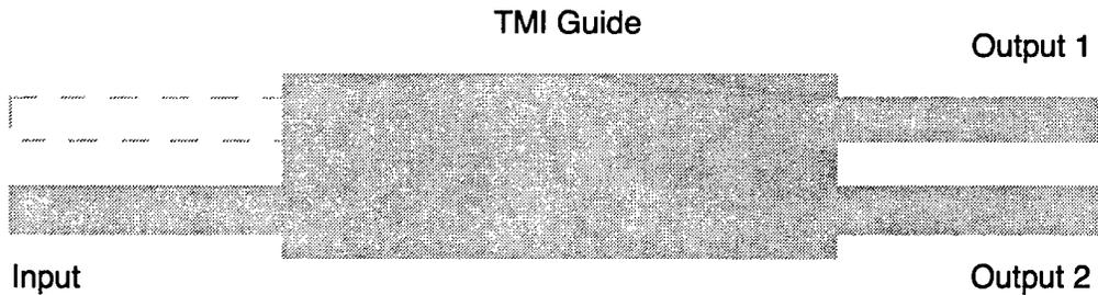
Figure 3-6 Schematic layout of Two Mode Interference splitter
