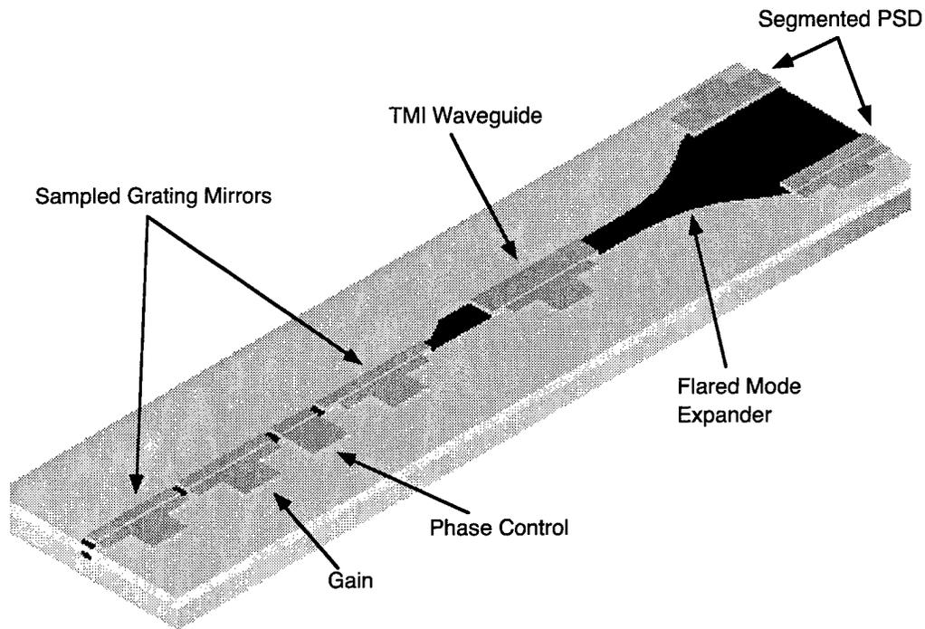
Figure 3-19 Buried SGDBR with integrated wavelength monitor incorporating flared mode expander and segmented detector.
