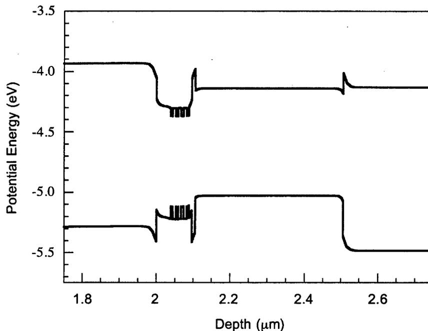
Figure 2-10 Active region band diagram at a bias of 1.2 V.
