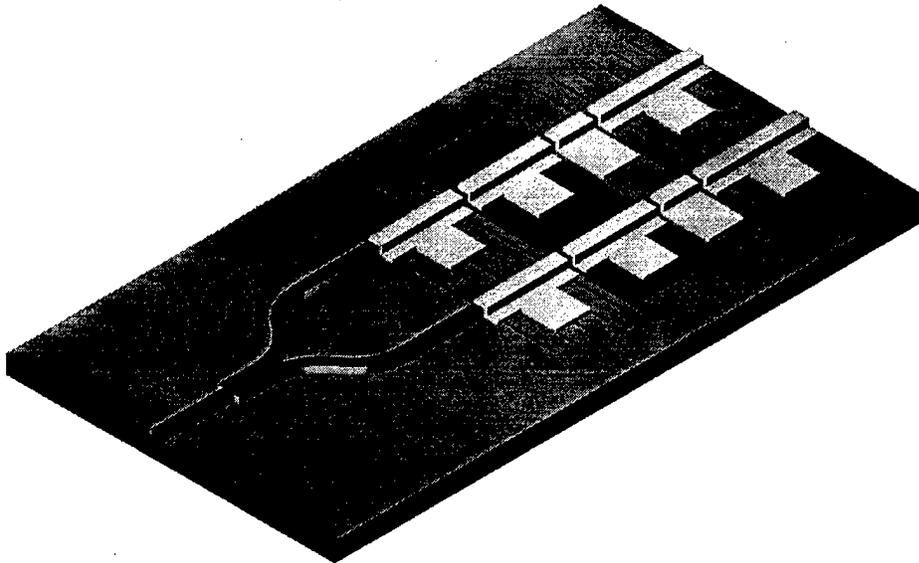
Figure 14. Hetrodyned SGDBR lasers
