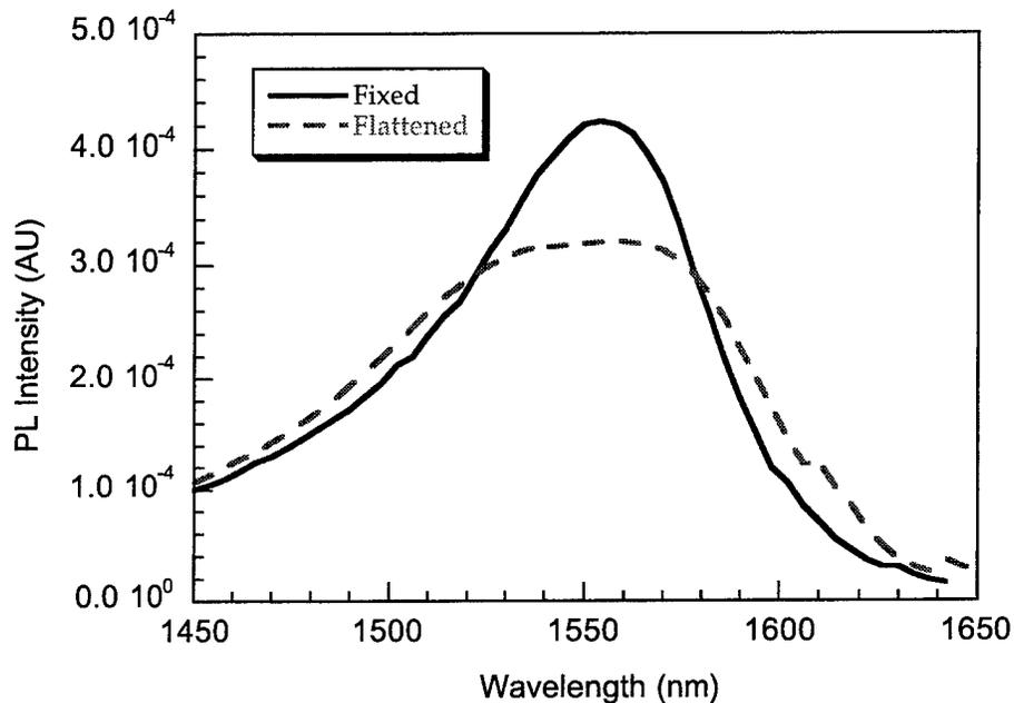
Figure 4-8 Comparison of PL spectrum from standard MQW structure and chirped structure for flattened gain.
