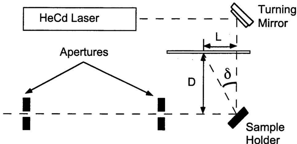
Figure 2-25 Grating period diffraction measurement setup.
