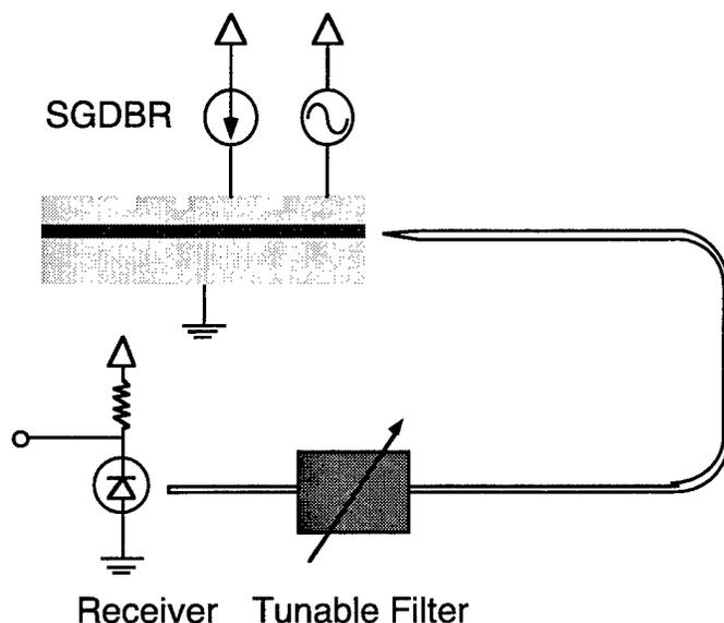
Figure 5-6 Experimental apparatus for wavelength switching tests.
