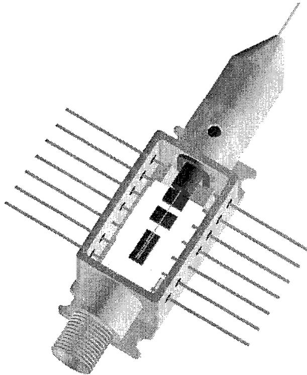
Figure 5-4 Rendering of assembled butterfly package
