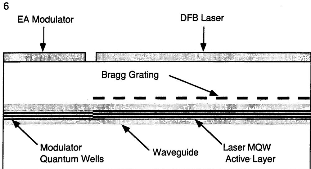
Figure 1-4 DFB Laser with integrated electro-absorption modulator
