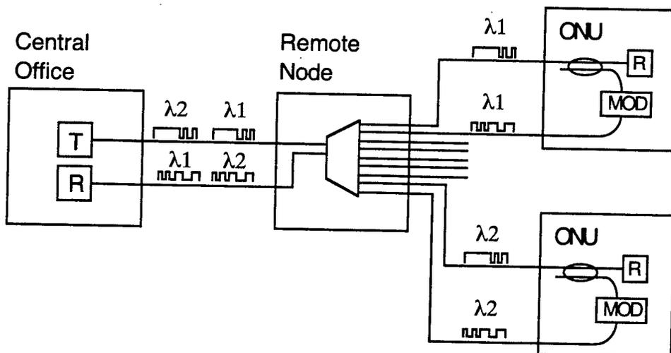
Figure 1-1 Wavelength Routed Passive Optical Network
