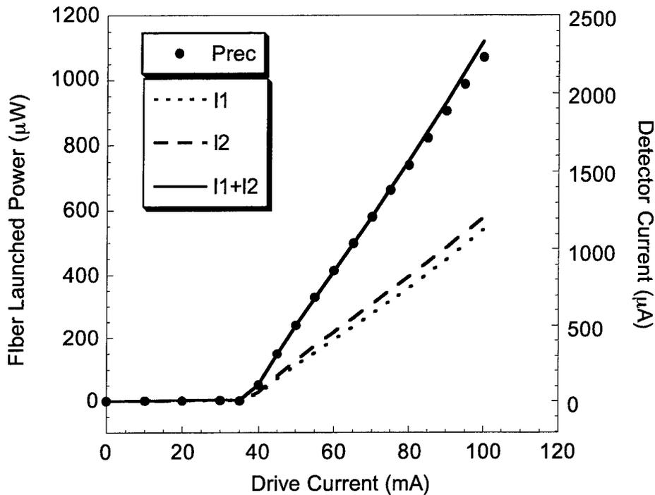
Figure 3-17 Intensity response for wavelength monitor detectors compared with fiber coupled output.
