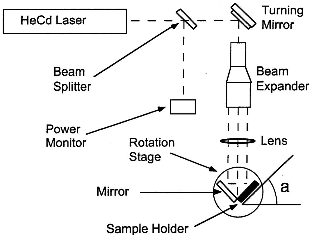
Figure 2-24 Holographic grating patterning system.
