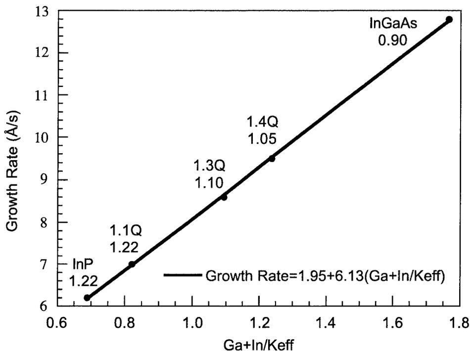
Figure 4-5 Growth rate vs. group III pure component flow for various materials from InP to InGaAs
