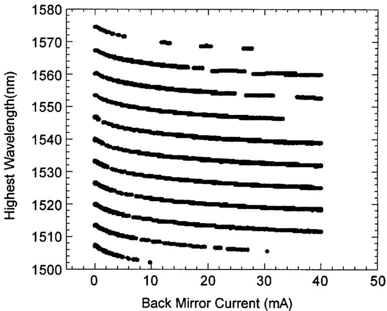
Figure 4b. Back mirror tuning curves for 72 nm quasi-continuous tuning range tested at 0.1 mA intervals from 0 to 40 mA. All points > 30 dB SMSR.
