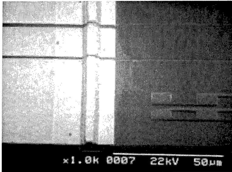
Figure 4-20 SEM of buried heterostructure DBR laser showing sidewall roughness
