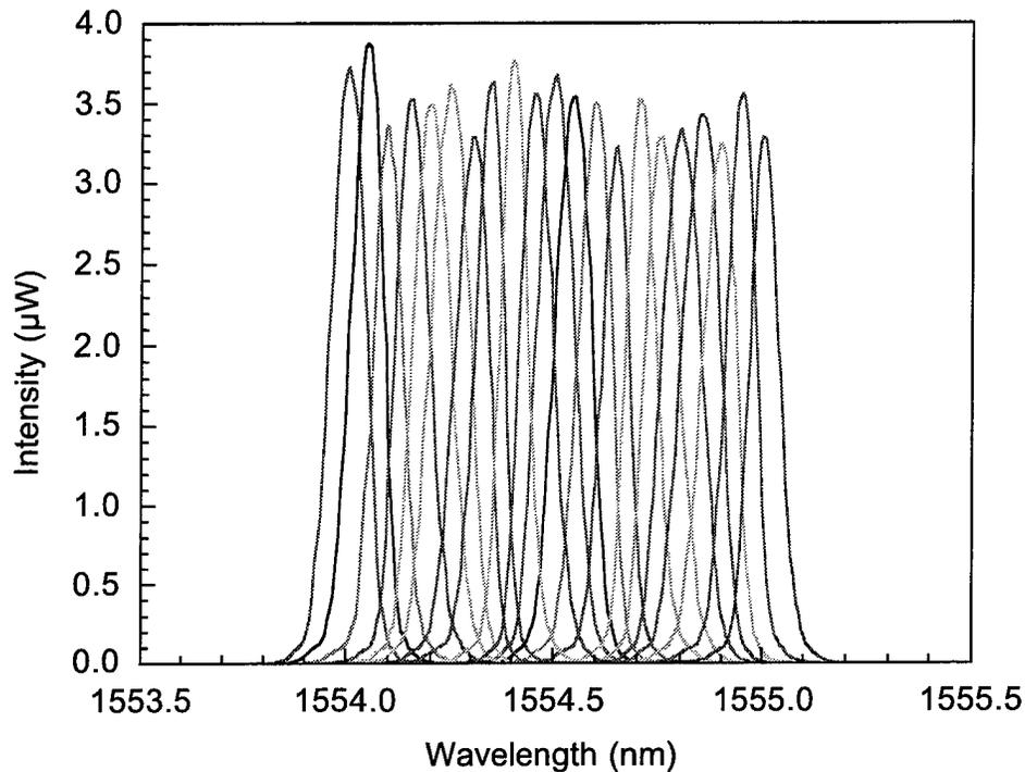
Figure 3-22 Laser spectra for fine wavelength scan in 0.05 nm increments from 1554 nm to 1555 nm..
