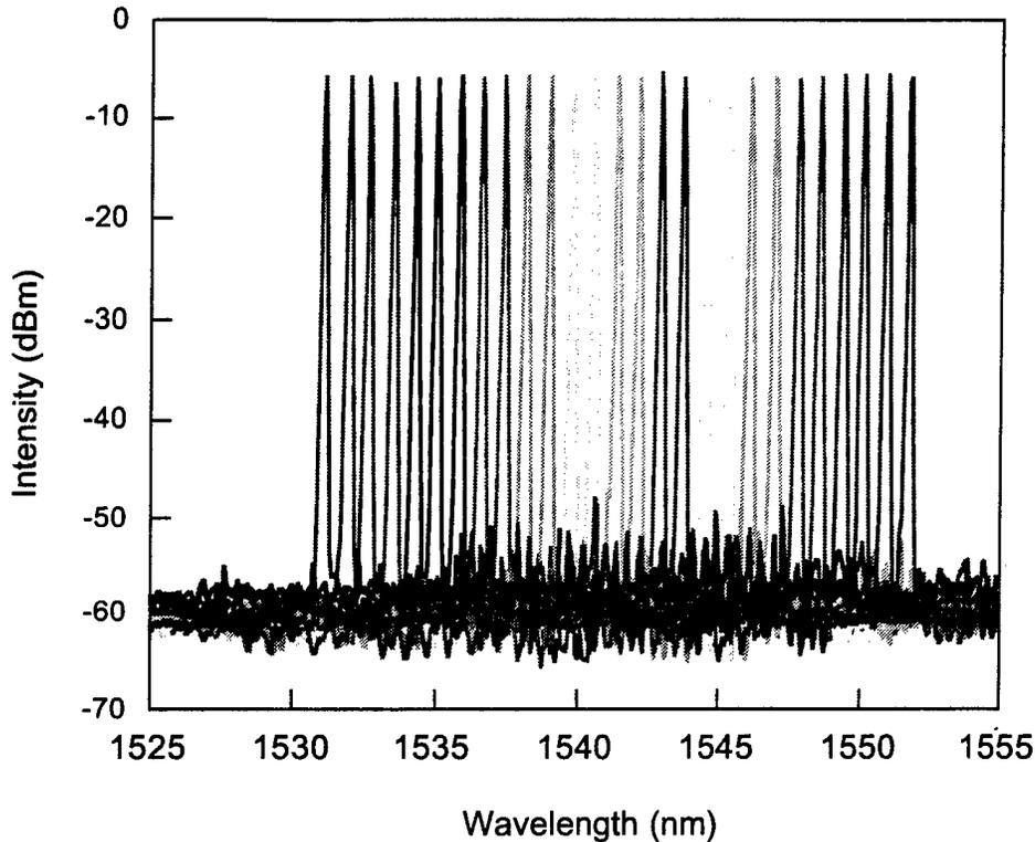
Figure 2-27 Superimposed spectra for ridge waveguide SGDBR showing 27 WDM Channels Spaced at 100 GHz.
