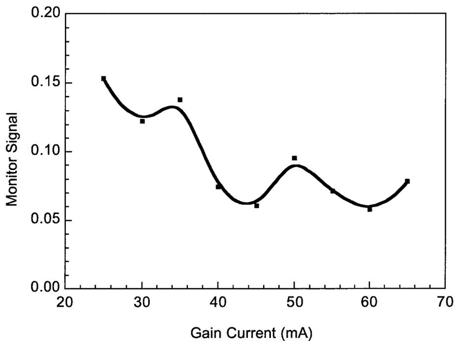
Figure 3-25 Splitting ratio variation with laser gain current for buried wavelength monitor at constant wavelength.
