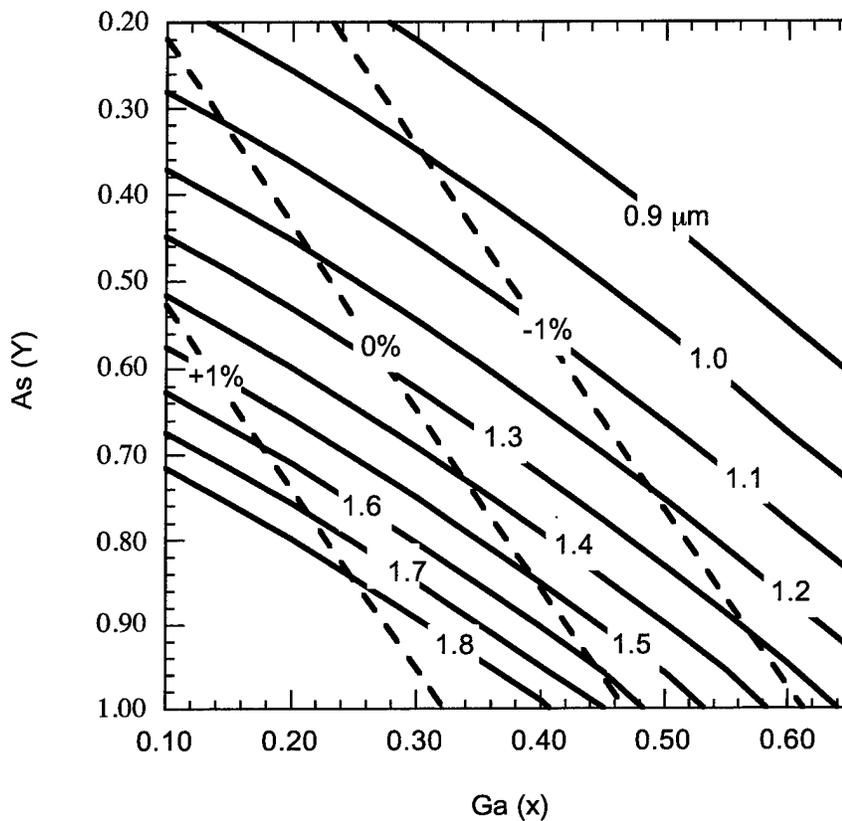
Figure 4-7 Bandgap and strain for  $\text{In}_{1-x}\text{Ga}_x\text{As}_y\text{P}_{1-y}$  quaternary material. Energy contours are plotted in wavelength.
