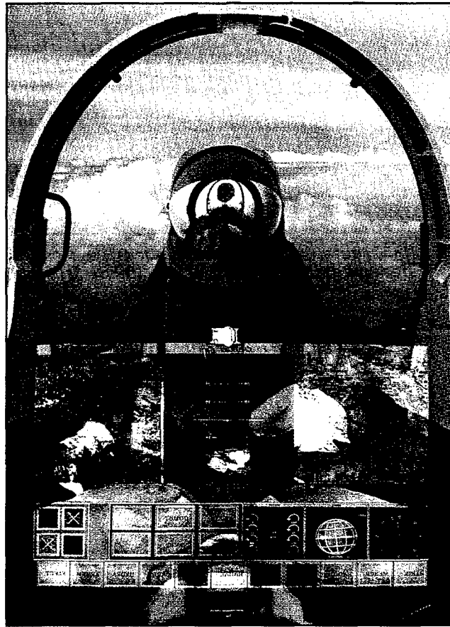
An experimental large interactive display (viewed from behind the display - it has not been printed back to front)
