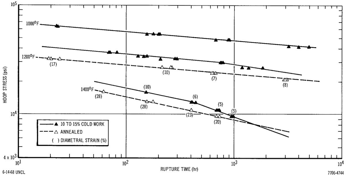
Figure 7. Biaxial Stress-Rupture Properties of Type 316 Stainless Steel in High-Purity Sodium
