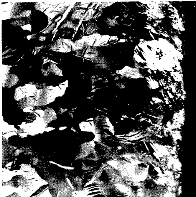
FIGURE 2. Mechanical Deformation as Affected by Band-Saw Sectioning of a Beryllium Specimen. Note the Microcracks, Which Often Occur, in the Upper Portion of the Photomicrograph. Polarized Illumination. Magnification 80X.
