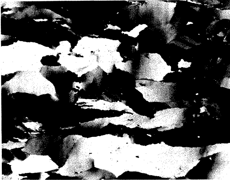
FIGURE 9. Unannealed Vacuum-Cast Ingot Beryllium Sheet. Subgrains are Inherent in Sheet in the Unannealed Condition. Polarized Illumination. Magnification 100X.
