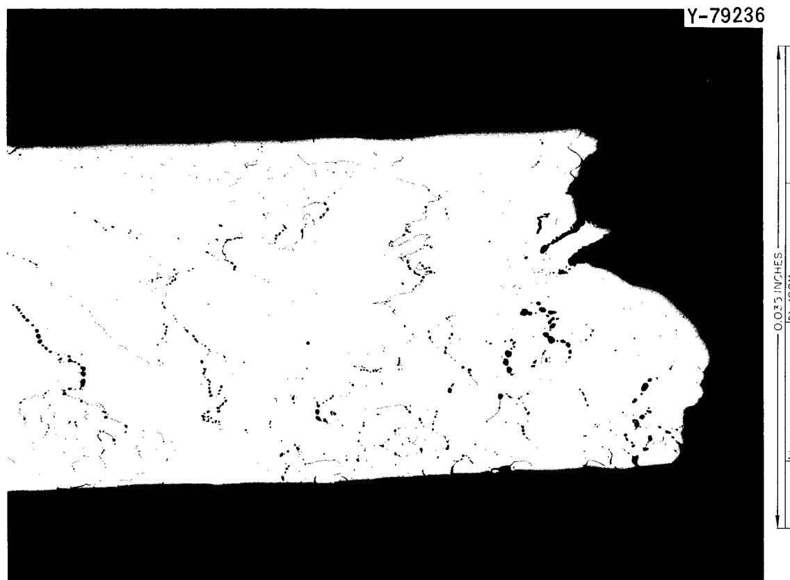
Fig. 14. Fracture of a CVD Tungsten Specimen from Lot PW-69 Tested at 6000 psi and 1650°C. Warm worked 80% and recrystallized at 2200°C prior to testing. Failed in 37 hr with 3.7% strain. Etchant: 50 parts \text{NH}_4\text{OH} and 50 parts \text{H}_2\text{O}_2 .
