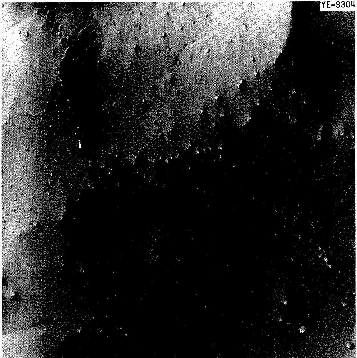
Fig. 10. Fractograph Approximately 10 mm from the Fracture of a CVD Tungsten Specimen Tested at 4000 psi and 1650°C. Ruptured in 413 hr with 3.2% strain. 11,250X.
