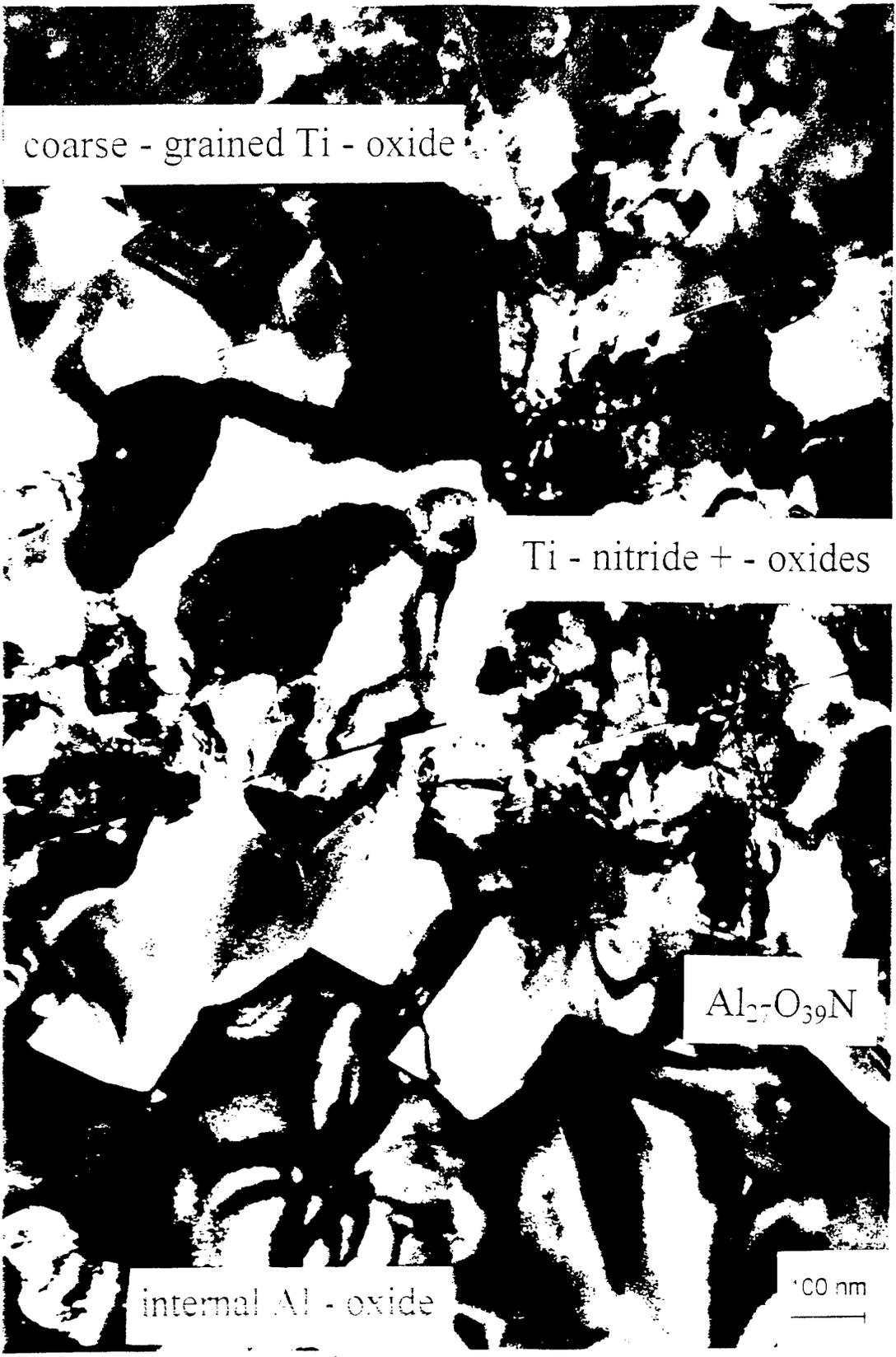
Metal - oxide interface of Ti35Al5Nb after oxidation at 900°C for 4 h in air.
