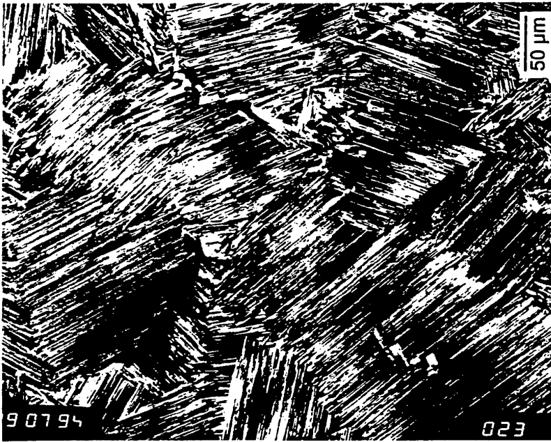
K5SC Alloy TMPL Extrusion LT-Section
