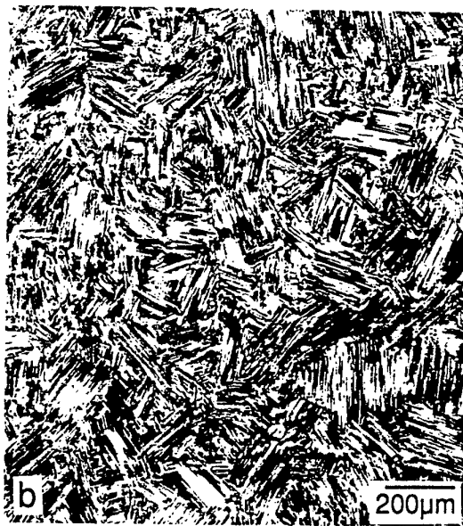
Lamellar Grain Size Control in Wrought Alloy K5
