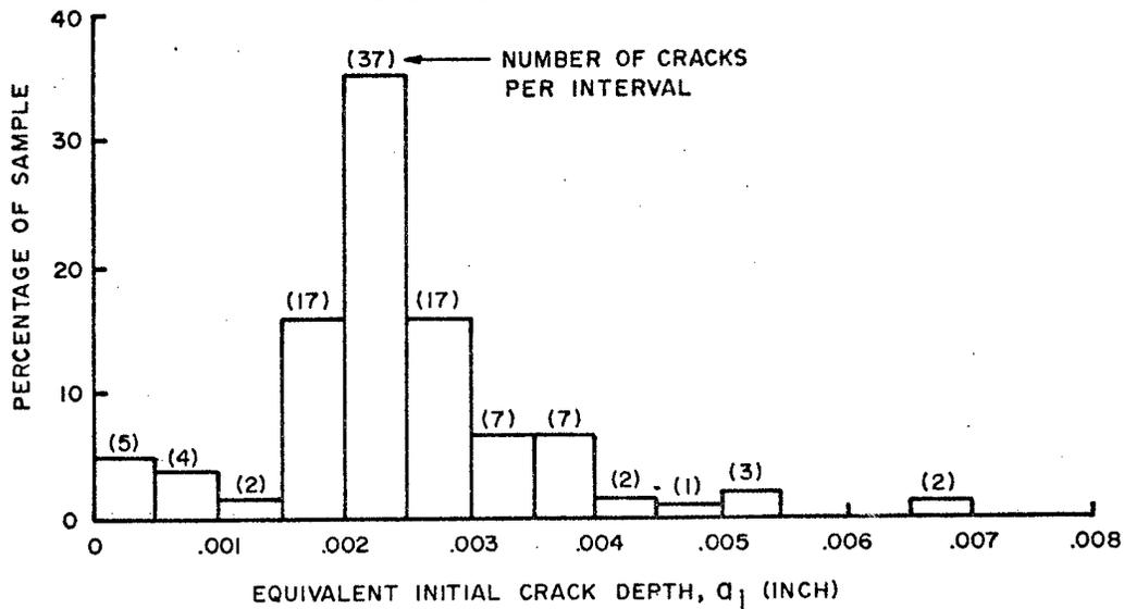
Figure 12. Equivalent Initial Crack Depth Histogram for F/RF-4C/D Aircraft
