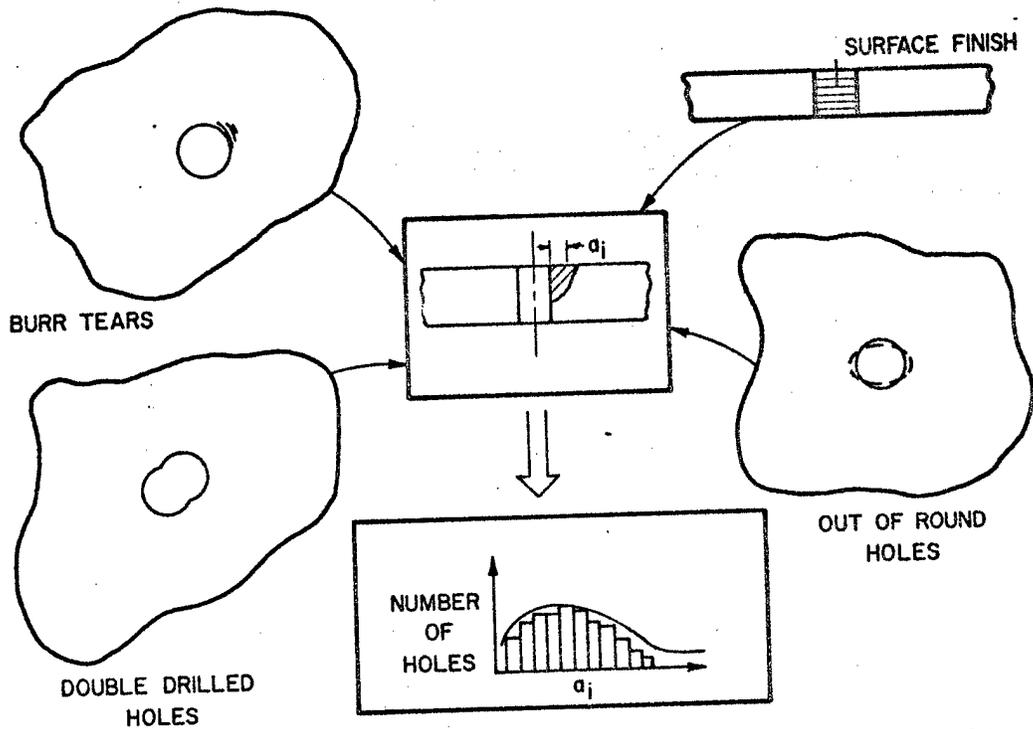
Figure 1. Parameters Which Affect Fastener Hole Initial Quality
