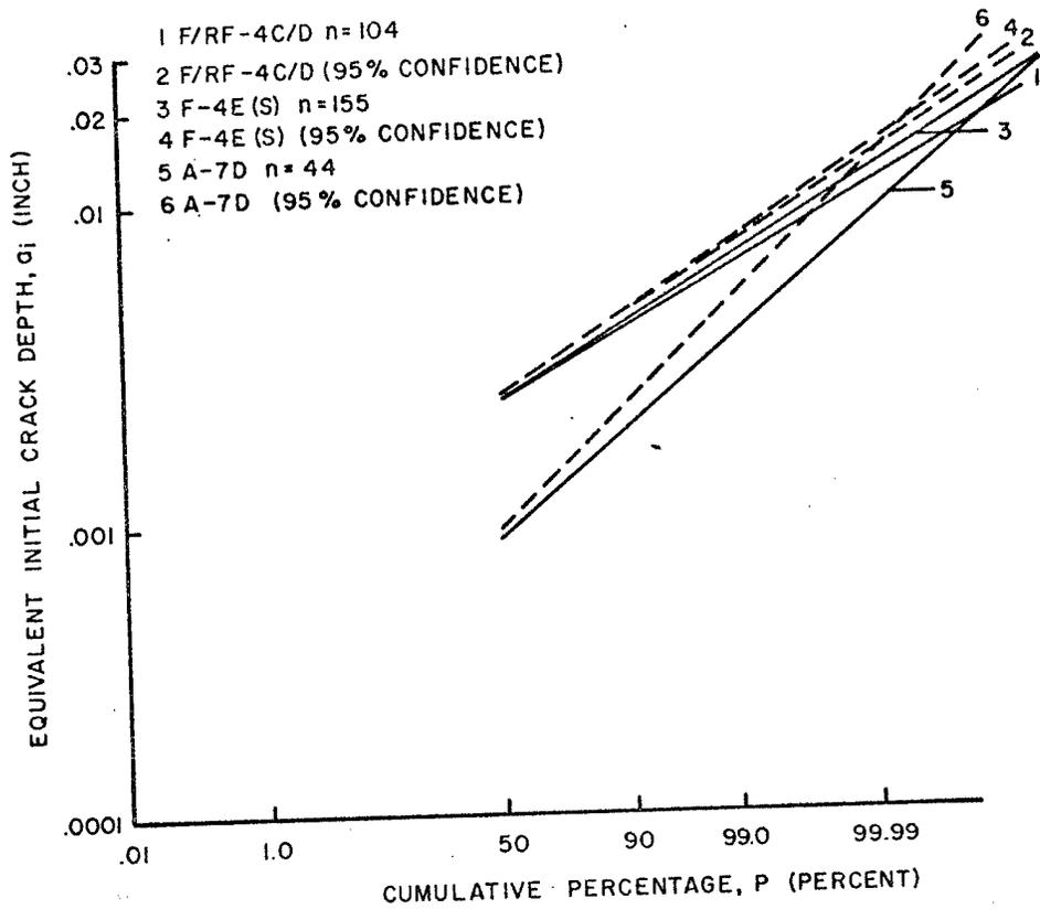
Figure 29. Equivalent Initial Crack Depth Distributions for F/RF-4C/D, F-4E(S) and A-7D Aircraft
