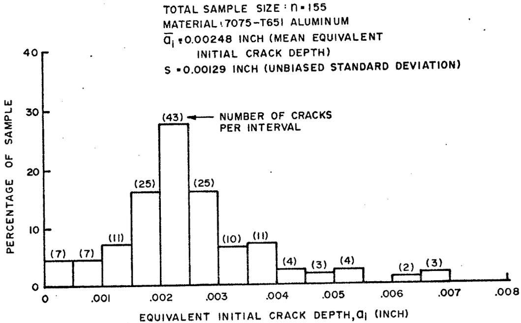
Figure 16. Equivalent Initial Crack Depth Histogram for Reamed Holes for F-4E(S) Aircraft
