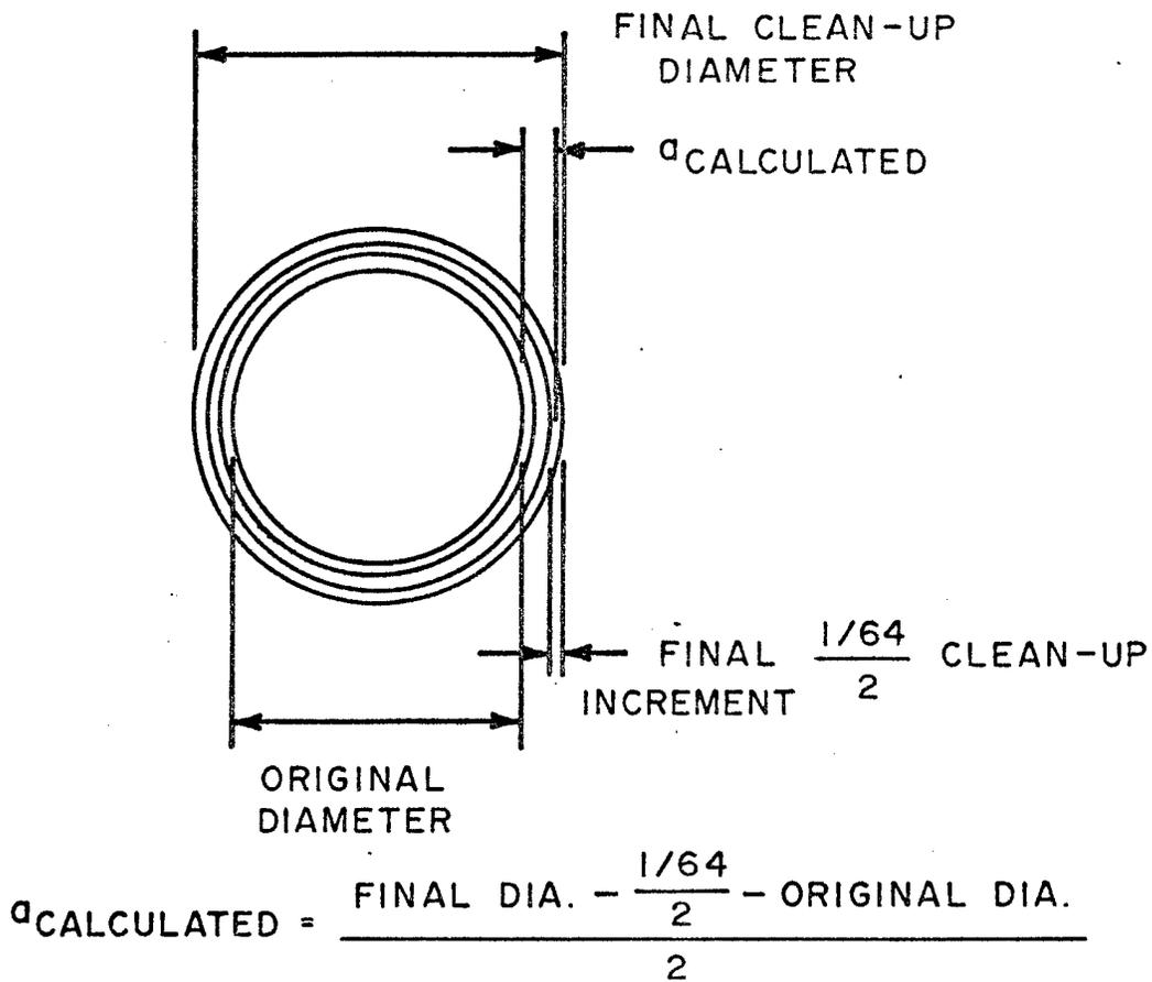
Figure 10. Calculated Crack Depth from Reamed Fastener Hole
