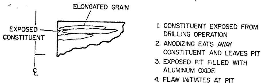
Figure 25. Cause of Flaw Initiation from Anodizing
