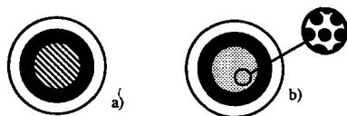
Figure 1: Sketch of the two electroding types of the front surface: the stripes are 200 \mu\text{m} with an interdistance of the same width.
