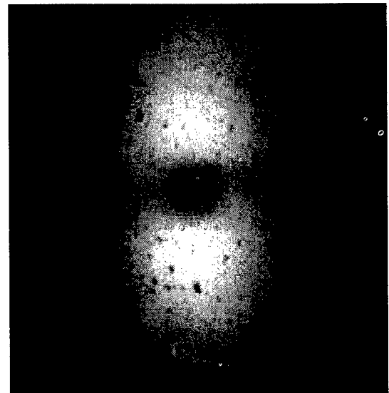
Fig 1 An image of the OTR angular distribution. The difference between horizontal and vertical planes is due to the use of a beam splitter
