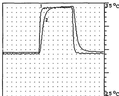
Figure 2: Experimental correlation between temperature of input (1) and output(2) cooling water and time. The scale of horizontal axis – 60 seconds per point. Water flow 0.27 lps
