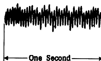
Figure 1 – Typical Field Vibration of 9 mm Shield Wire
