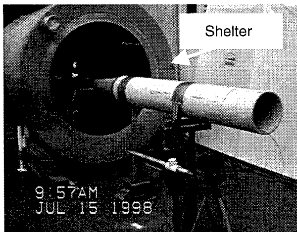
Figure 29. Side and rear view of universal vortex ring generator and extension tube mounted inside a protective shelter.
