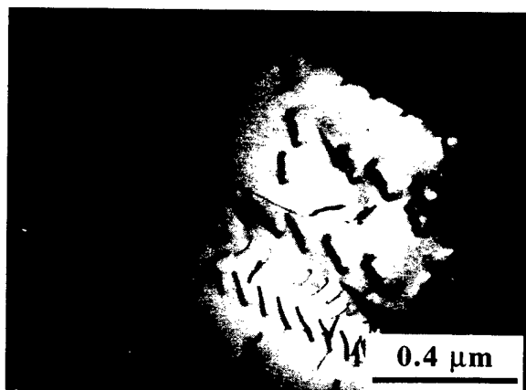
Fig. 4. Typical TEM micrograph after deformation at room temperature. Number and spatial extent of dislocation arrays is greatly increased compared to the undeformed samples.
