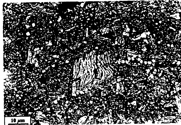
Fig. 5. Optical micrograph of etched cross section of a sample deformed at 1300 ^{\circ}\text{C} in compression. Grain denoted by the arrow buckled and delaminated into the void that formed to its right. Compression direction is vertical.
