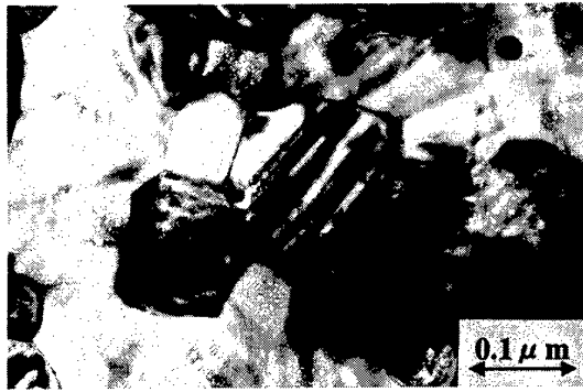
Fig.1. TEM image of the doped BaTiO 3 ceramics of grain size 150nm.
