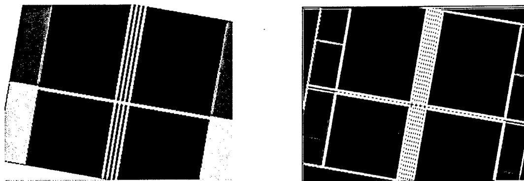
Figure 22. Tilted test pattern before (left) and after (right) Sober edge detection.
