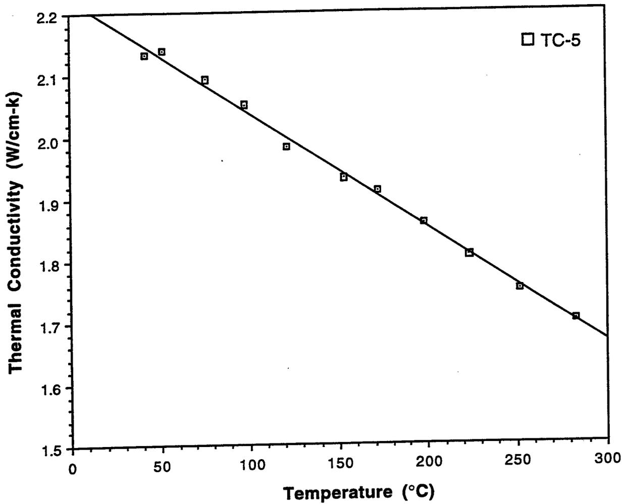
Figure 1. [90°] Thermal Conductivity vs. Temperature Plot of P30X/C (EO-1) Specimen.
