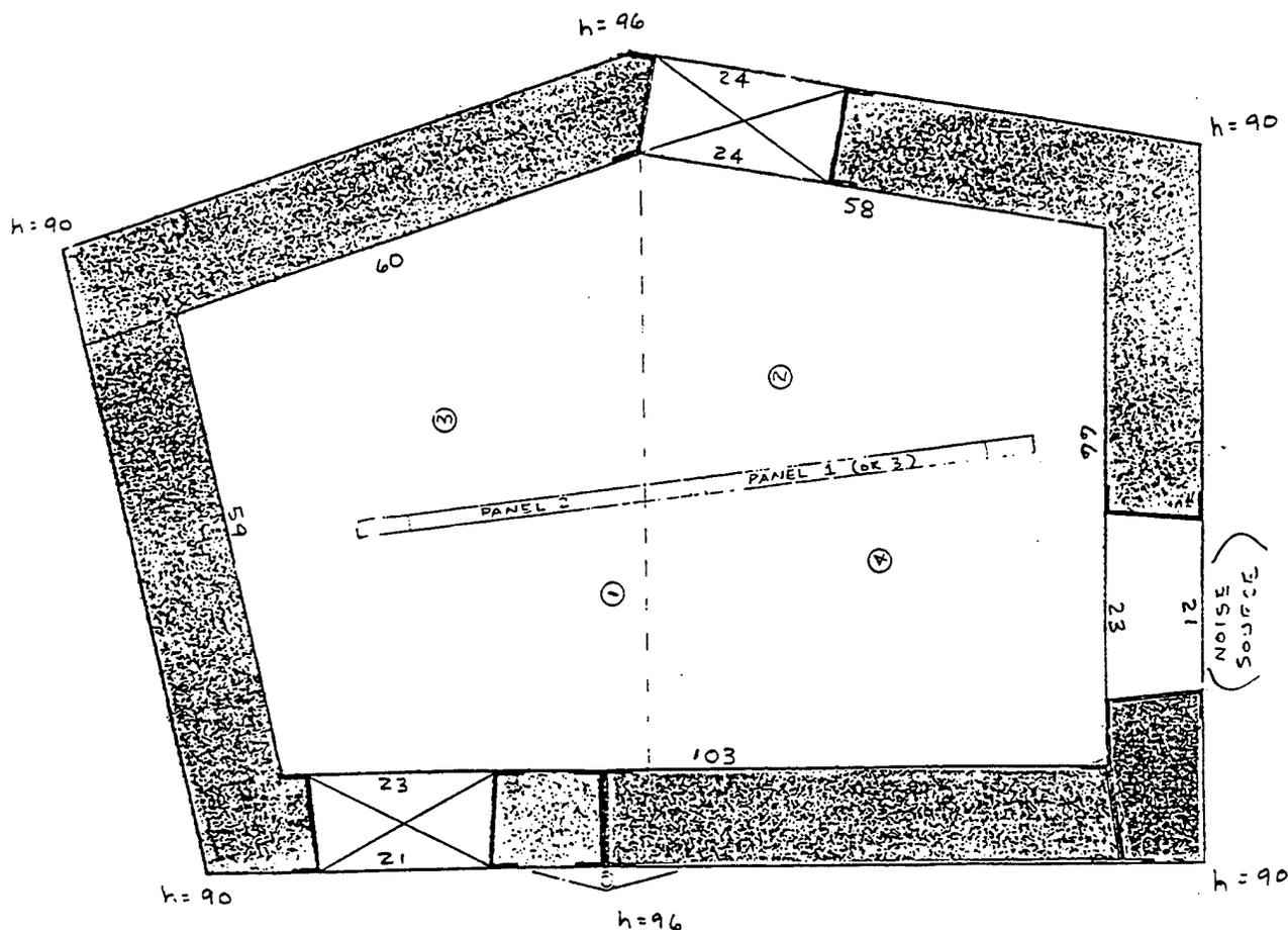
**Figure 3.1.1** 400 ft<sup>3</sup> Reverberant Chamber of the Acoustics Laboratory
