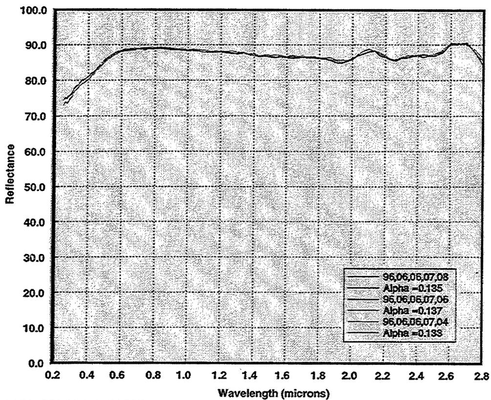
Figure 9 Solar Absorptance Measurements of Panel 3
