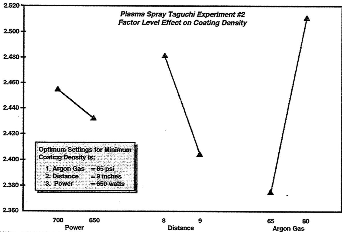
Figure 21 Factor Level Effect on Coating Density
