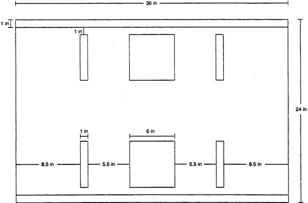
Figure 2.2 Configuration of Panel 3 with Edges Reinforced and Test Coupons Attached
