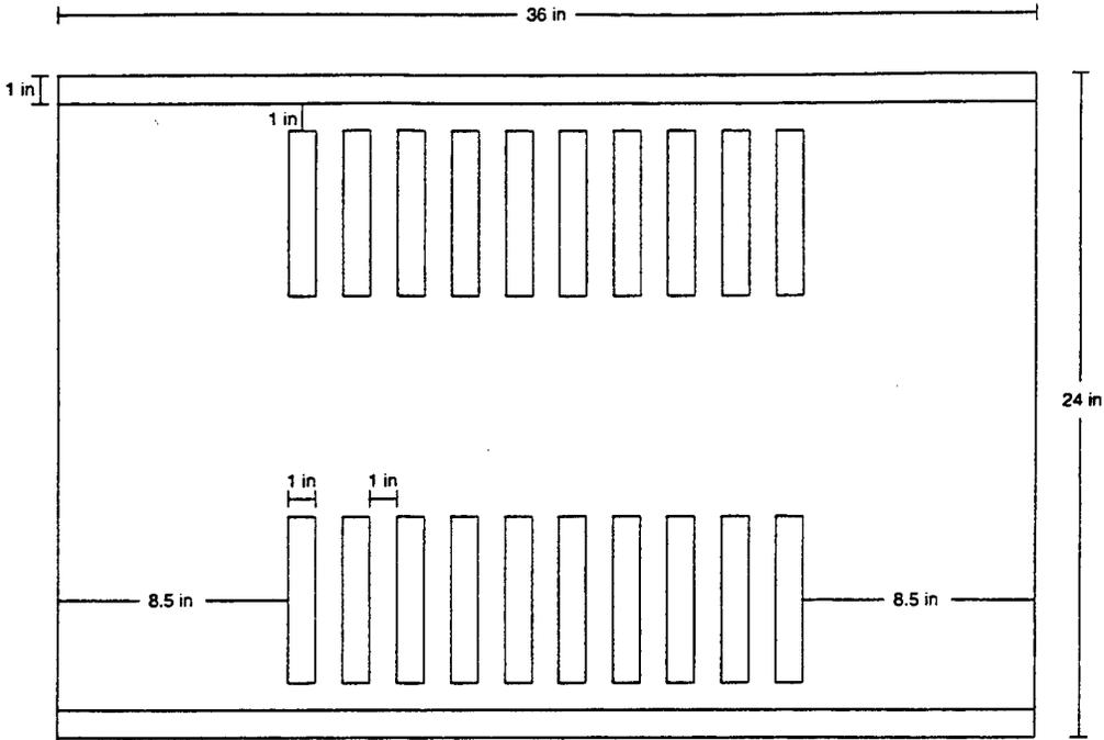
Figure 2.1 Configuration of Panels 1 and 2 with Edges Reinforced and Test Coupons Attached
