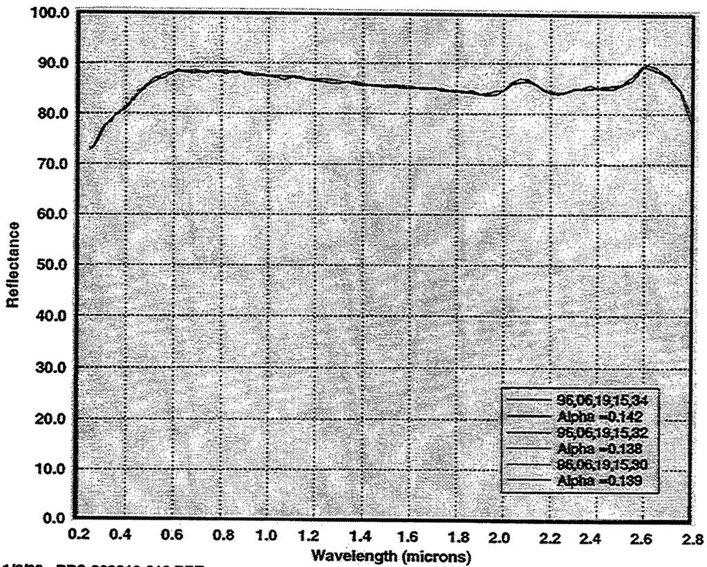
Figure 15 Solar Absorptance Measurements of Panel 9
