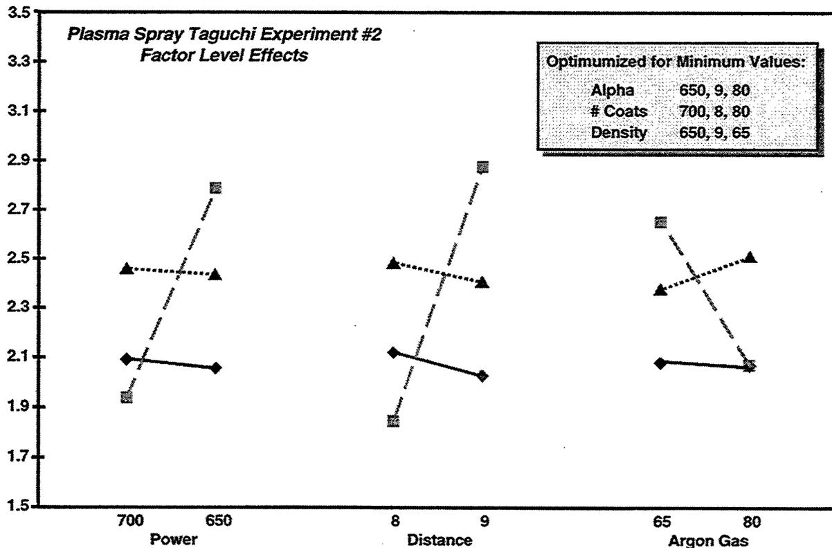
**Figure 23 Verification Experiment Factor Level Effects**
