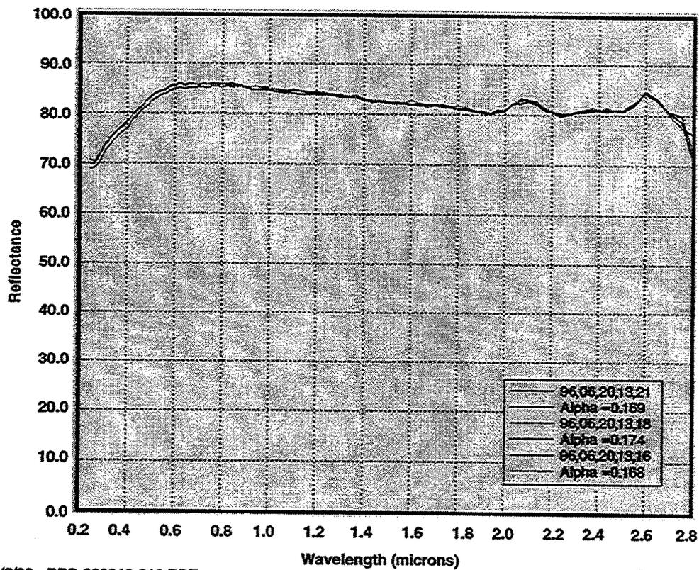
Figure 16 Solar Absorptance Measurements of Panel 10
