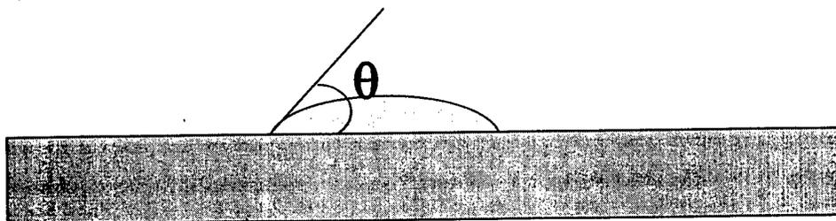
Figure 2. Contact angle of a liquid drop on a solid surface.
