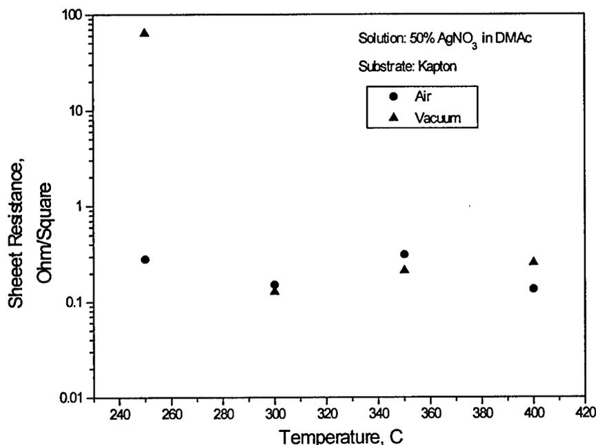
Figure 6. Effects of heat-treatment conditions on conductivity of Ag conductor patterns on Kapton® films. Resistance of the Ag patterns was measured with the 2-probe method.
