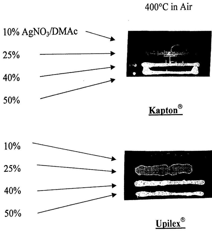
Figure 4. Ag conductor patterns formed from AgNO<sub>3</sub>/DMAc precursor solutions of different concentrations on Kapton<sup>®</sup> and Upilex<sup>®</sup> substrates after heat treatment at 400°C in air for 30 min.
