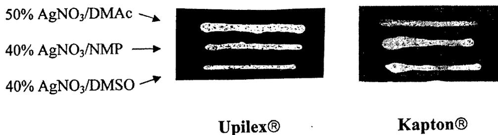
Figure 5. Ag conductor patterns derived from AgNO<sub>3</sub> solutions in different solvents. The patterns were printed on the substrate with a drawing pen and heat treated at 300 °C in air for 30 min.
