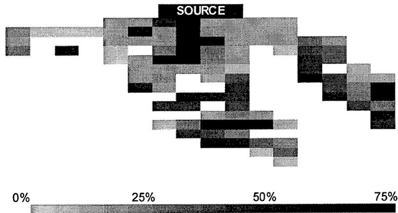
**Figure 2.** Experiment 1, NAPL saturation after 7 days.
