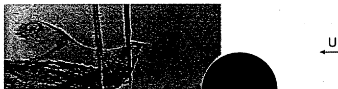
Figure 1: The upwelling of near-wall fluid at the edge of the wake area ( x/D \approx 1.5 ) downstream of the hemisphere (side view, flow direction to the left).
