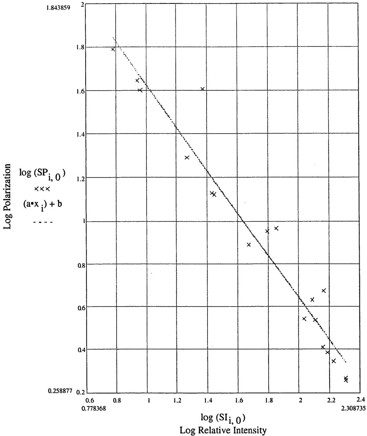
**Figure 4.** Log of the polarization of recorded radiance in the NIR band plotted against the log of the scene radiance for uniformly illuminated artificial gray targets shown in Figure 1.
