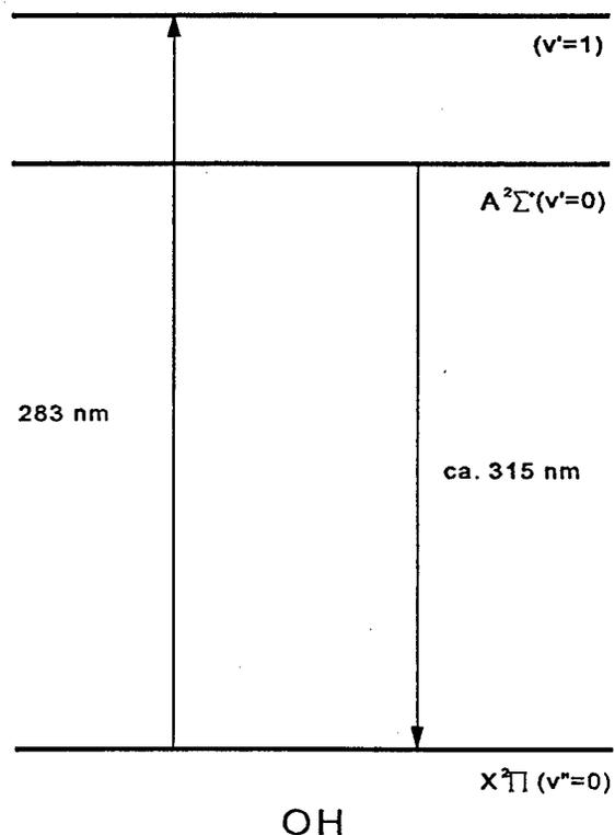
Figure 1. Energy Level Diagram for OH radical.
