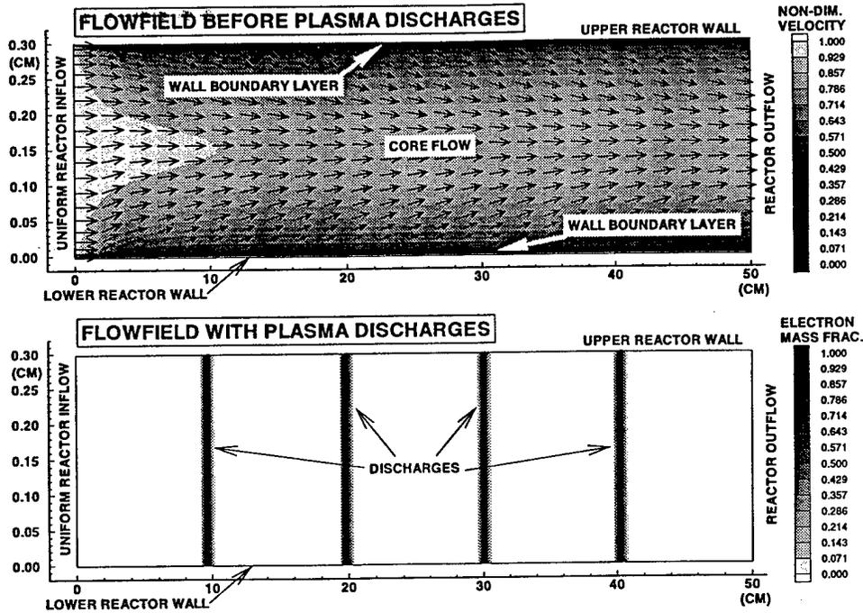
Figure 5. Computed Flowfields with and without Plasma Discharges.
