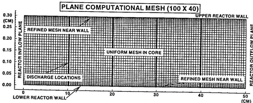
Figure 4. Problem Setup and Computational Mesh.
