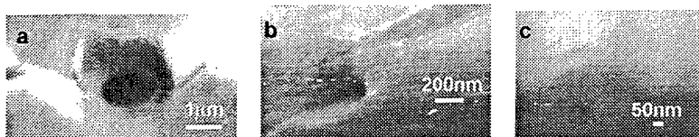
Fig.3. SEM cross-sectional images of epitaxially overgrown micro- and nanotubes: a- initial overgrowth stage of tubes of large diameter (1 \mu\text{m} ); b- fully overgrown tube of 200 nm diameter, the tube is inclined at an angle to the cleavage; c- an overgrown tube of a \sim 10 nm inner diameter, outside diameter \sim 60 nm (tube was self-scrolled from a 2ML GaAs+1ML InGaAs film and consisted of 20 turns).
