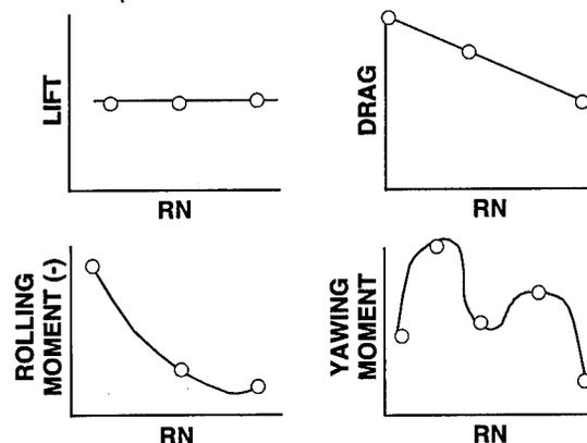
Fig. 2. Example of RN effects on a low observable aircraft.
