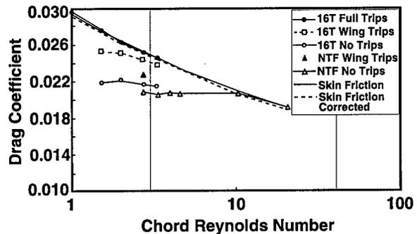
Fig. 6. Drag as a function of Reynolds number for  $M = 0.6$ ,  $\alpha = 2.0$  deg.
