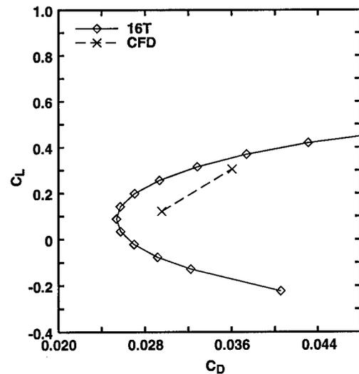
Fig. 16. Measured and computed forces and moments,  $M = 0.835$ ,  $Re_c = 2.7 \times 10^6$ , full trips.
