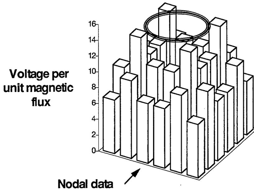
**Figure 6. Columnar Plot of Equation (2) for the Output of the Planar Grid Model's Computer Code. Each Column Represents the Voltage Between Plies for a Planar Grid Node in the Plane of the Laminate. The Relative Position of the Coil Is Shown.**
