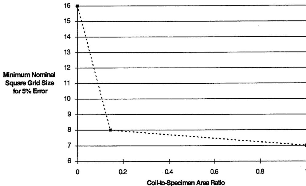
**Figure 16. The “Accuracy Zone” for Coil-to-Specimen Size Ratio as It Relates to the Grid Density Used in the Planar Grid Model. Note That a Minimum Grid Size of  $8 \times 8$  is Accurate for All Coil-to-Specimen Area Ratios.**
