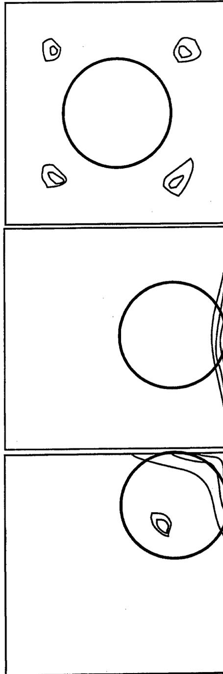
**Figure 19. Results of Liquid-Crystal Thermal Measurement Observations for a 10-cm Helmholtz Coil on a 20-cm-square [0/90] Cross-Ply Laminate. The Ring Indicates the Placement of the Coil. The Contours Represent the Progression (From Inside To Outside) of Heating as Witnessed From the Liquid Crystal in the 40–45°C Range. Note the Points of Highest Heating, as Predicted in Figure 15.**
