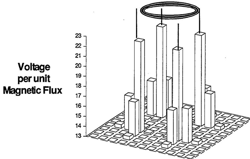
**Figure 18. The Predicted Nondimensional Voltage Profile From the Planar Grid Model for the  $10 \times 10$  Grid Representation Used to Model the Tape Segments of Figure 17. Only the First Two Sets of Highest Heating (Those in Excess of 13) Are Shown. All Lower Voltages Are Omitted Here for Clarity. The Ring Above the Graph Indicates the Placement of the Helmholtz Coil on the Specimen.**
