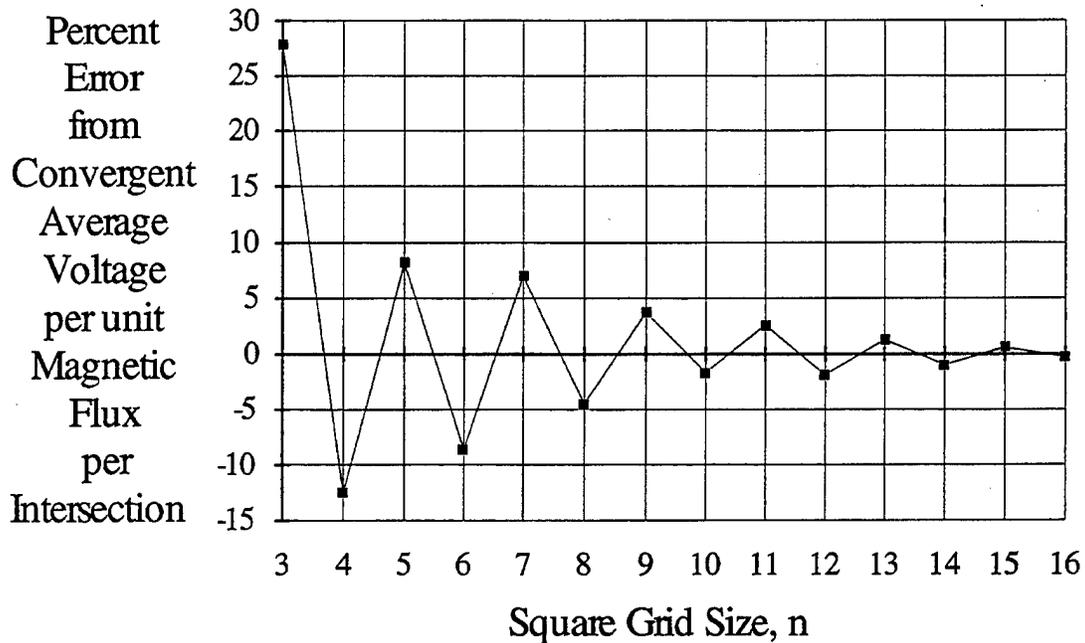
**Figure 11. Plot of Percent Error of Average Nondimensional Voltage for Various Grid Sizes From the Convergent Solution at Infinite Grid Fineness. Note That an  $8 \times 8$  Grid Size Is Within a 5% Error Limit From the Convergent Value Determined From Figure 10.**
