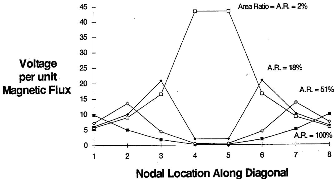
**Figure 13. Predictions of the Effects of Changing the Size of the Helmholtz-Type Coil With Respect to the Size of the Laminate Specimen for Centered-Coil Experiments.**
