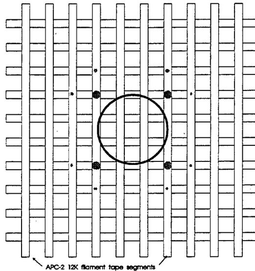
**Figure 17. A  $10 \times 10$  APC-2 Tape Grid. The Large Circle Represents the Placement of the Helmholtz Coil. The Small Circles Represent the Points of Heating as Indicated by Liquid Crystal Sheet ( $40\text{--}45^\circ\text{C}$  Range). The Intensity of Heating Is Thus Indicated by the Size of the Dots. Note the Four Points of Highest Heating and the Eight Points of Second-Highest Heating.**
