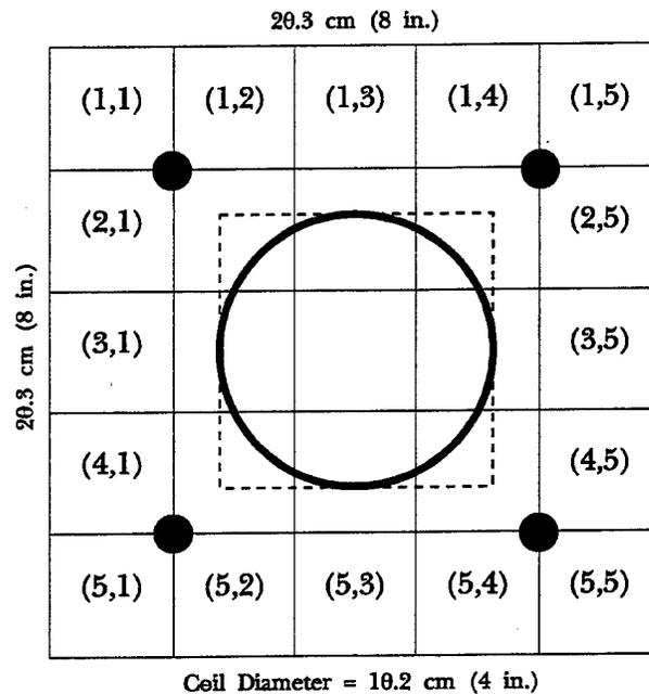
**Figure 8. Prediction of the Points of Highest Heating for a 5 × 5 Grid Size Representation (Darkened Circles). In a Test Specimen, the Points of Highest Heating Fall at the Points of Intersection of the Tangents (Dashed Lines) to the Flux Region (Bold Circle) Due to the Nearly Infinitely Fine Grid.**
