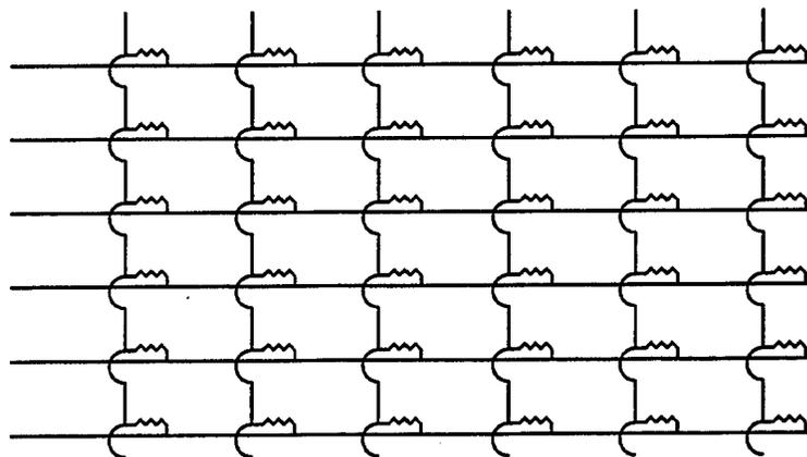
**Figure 2. An Electrical Network Analog to a [0/90] Cross-Ply With a  $5 \times 5$  Grid Size Representation in the Plane. Note That Fiber-Fiber Intersection Resistances Are Considered to Be Equivalent in the Ply-Ply Interaction Submodel.**
