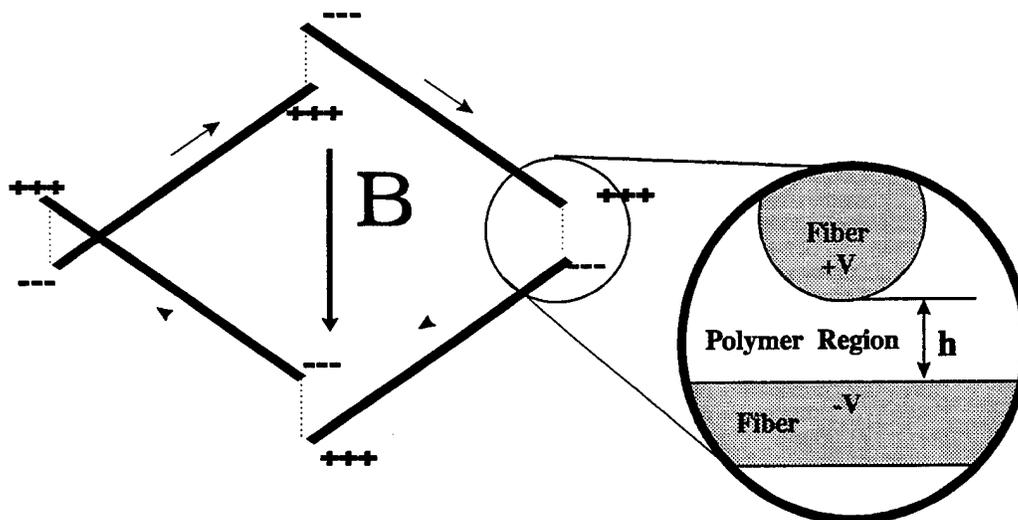
**Figure 1. Induced Current Due to a Transverse (Normal to the Plane) Magnetic Field in a  $[0/90]_s$  Cross-Ply. A Matrix-Rich Region of Thickness  $h$  Exists Between the orthogonal plies in such a laminate.**
