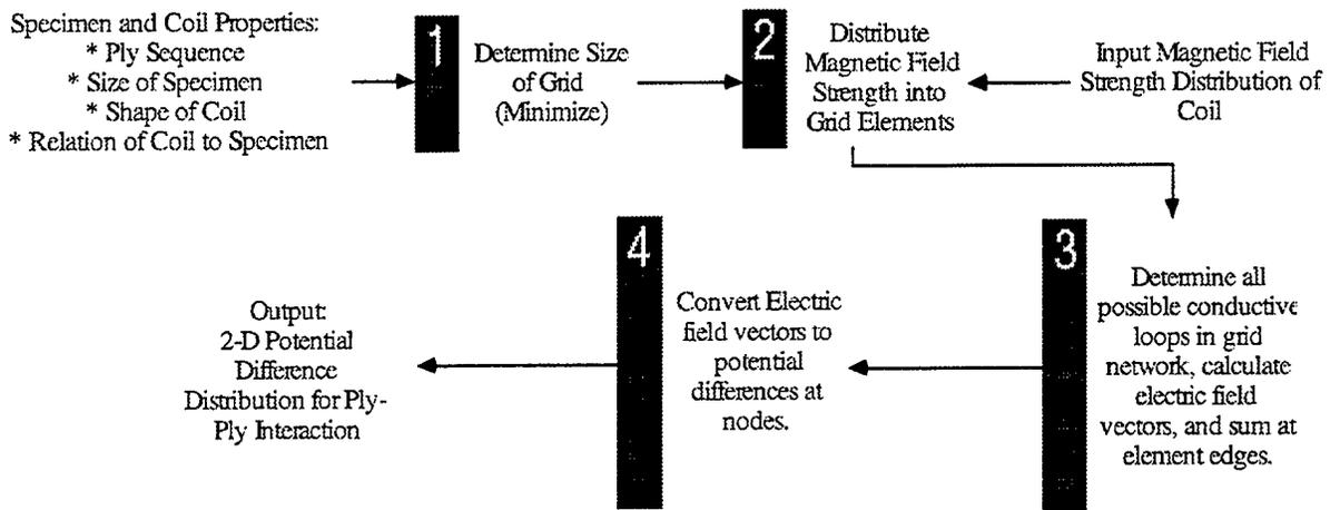
**Figure 4. Process Flow Diagram for Planar Grid Model.**
