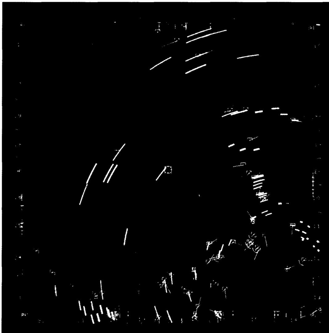
**Figure 2.15:** *Typical Airborne Early Warning radar display showing radar detection data, radar tracks, map overlays and supplemental alpha-numeric data.*
