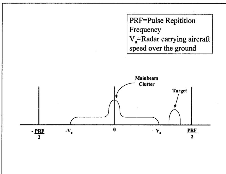
**Figure 2.8:** Clutter spectrum of a radar with a pulse repetition frequency high enough, such that the clutter is unambiguous at the radial component of the radar platform groundspeed along the clutter patch angle.
