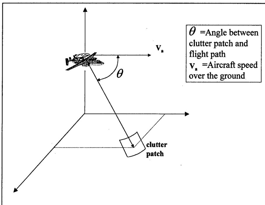
**Figure 2.7:** Clutter has an apparent doppler component due to the relative motion of the radar carrying aircraft over the ground. The nature of the clutter is defined by the angle between the aircraft velocity vector and the clutter patch, and the groundspeed of the aircraft.
