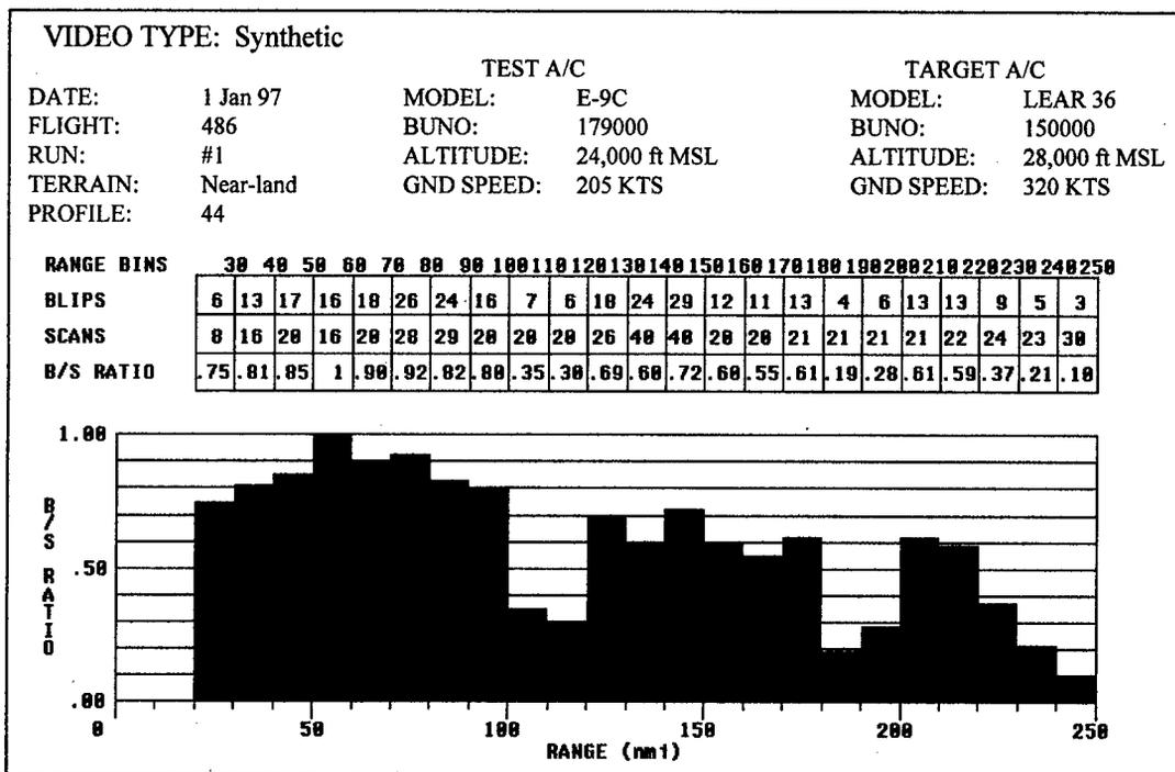
Figure 4.1: Sample Blip-Scan (B/S) ratio plot for target flying a radial inbound track in near-land environment with the land-sea interface at 110 nm and the clutter line at 190 nm.
