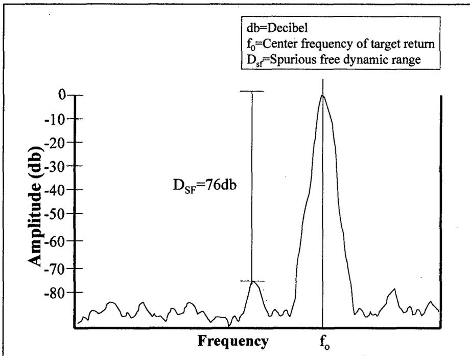
**Figure 2.4:** Spurious free dynamic range shown as the difference between the amplitude of the full scale input and the peak, or largest, spurious response.
