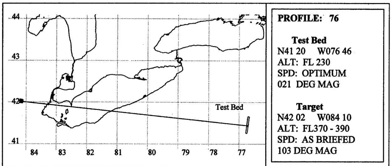
Figure 4.5: Over-land maximum detection range test scenario.
