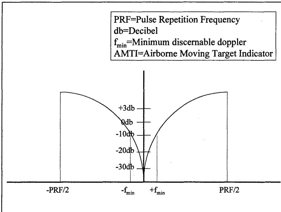
**Figure 2.12:** The transfer function of the Airborne Moving Target Indicator (AMTI) filter, showing the maximum output when the doppler shift of the target approaches half of the Pulse Repetition Frequency (PRF) and a zero output when the doppler shift approaches zero.  $f_{min}$  is the minimum doppler shift at which the radar can discriminate between real moving targets and the clutter return signal.
