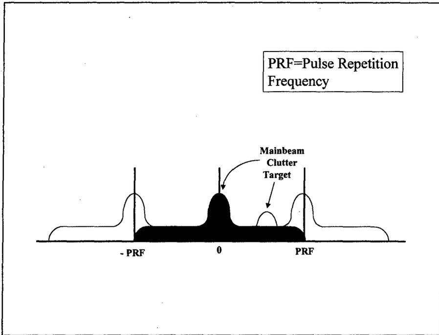
**Figure 2.9:** Clutter spectrum of a radar with a pulse repetition frequency, such that the clutter is ambiguous at the radial component of the radar platform groundspeed along the clutter patch angle.
