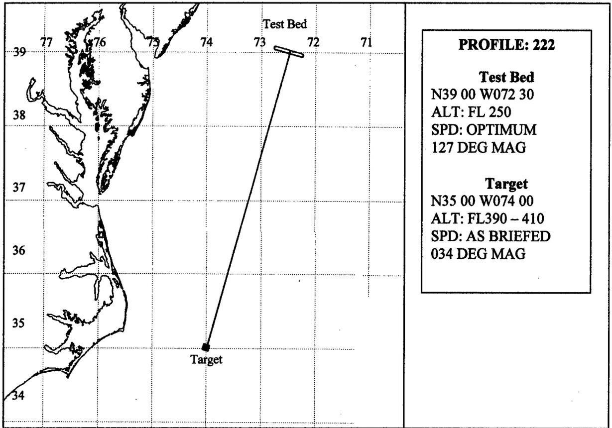
Figure 4.4: Over-water maximum detection range test scenario.
