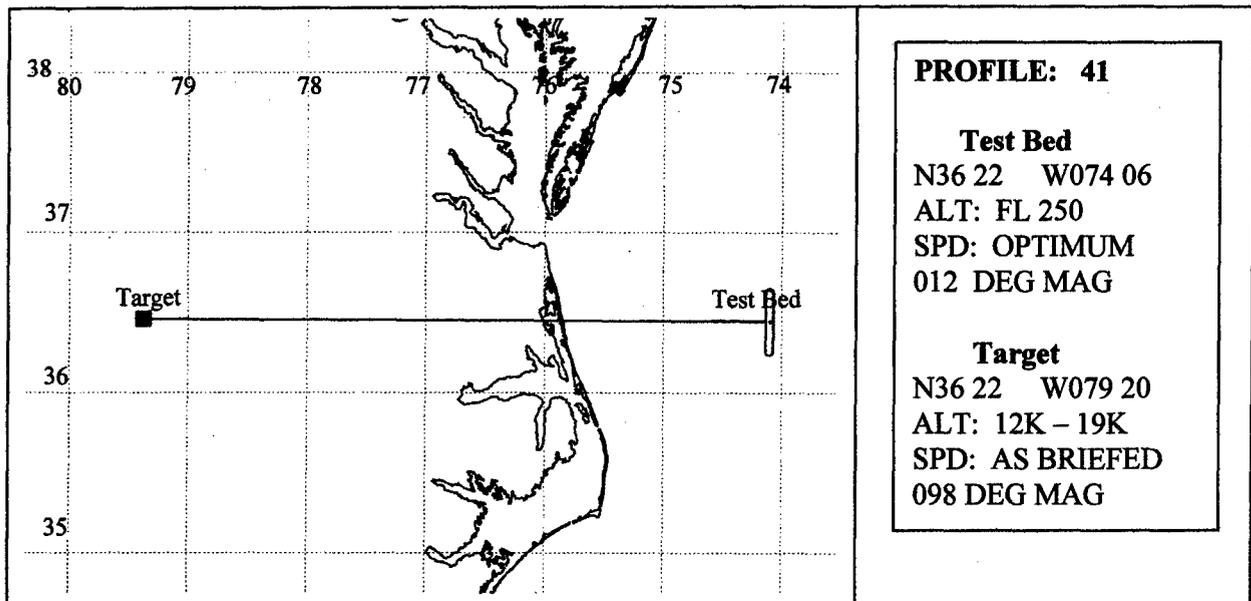
**Figure 4.6:** *Near-land maximum detection range test scenario.*
