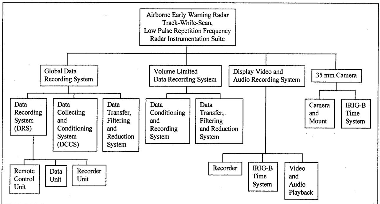
**Figure 3.3:** *Taxonomy of the complete sample instrumentation system.*
