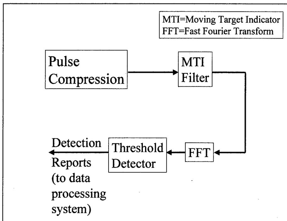
**Figure 2.6:** Typical Airborne Early Warning radar signal processor.
