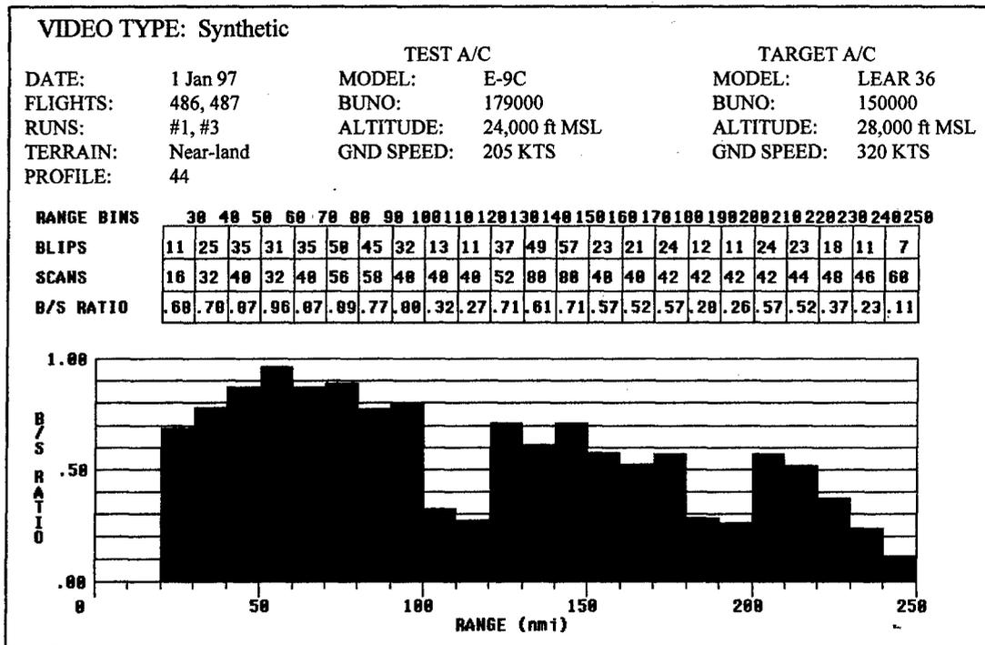
Figure 4.2: Sample composite Blip-Scan (B/S) ratio plot for two target runs where the targets are flying a radial inbound track in a near-land environment with the land-sea interface at 110 nm and the clutter line at 190 nm.
