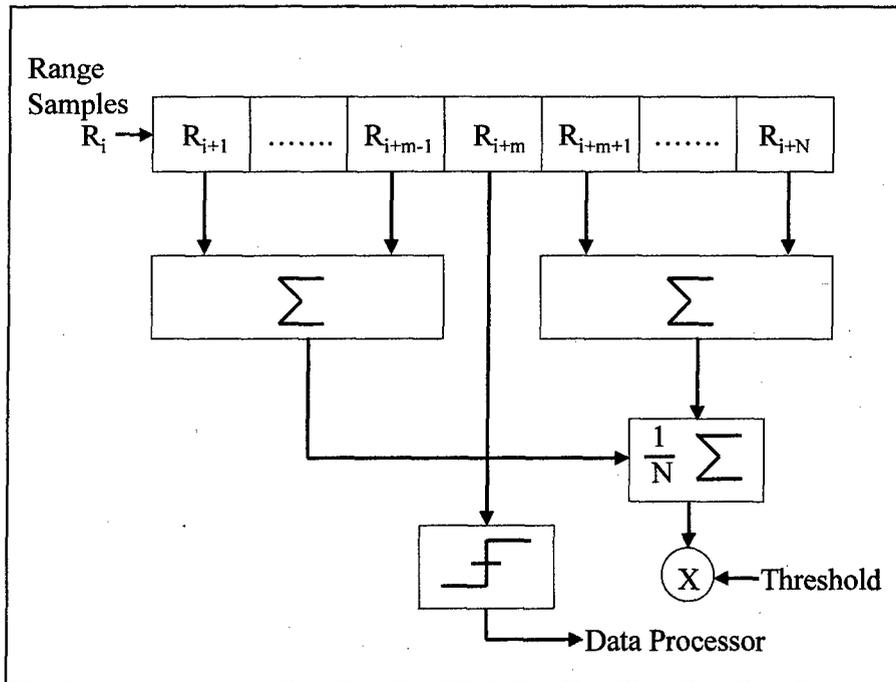
**Figure 2.13:** Cell Averaging Constant False Alarm Rate (CA-CFAR) system which approximates the average of the range cells before and after the test cell by summing samples and then setting the threshold to the greater of these two sums.
