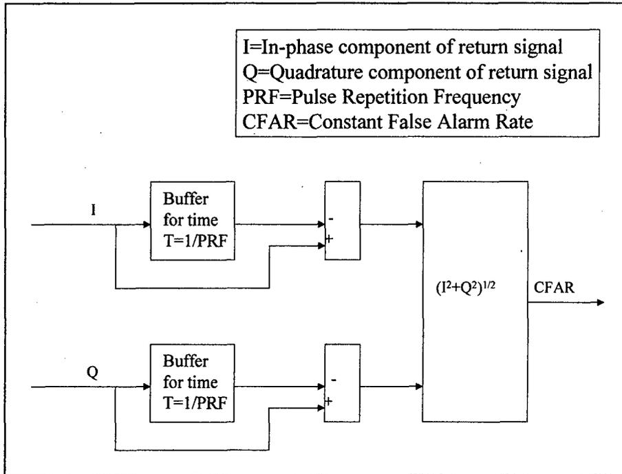
**Figure 2.11:** A digital delay line canceller, which uses the In-phase (I) and Quadrature (Q) output of a synchronous detector to cancel out the effects of stationary clutter and to highlight the presence of targets with motion over the ground.
