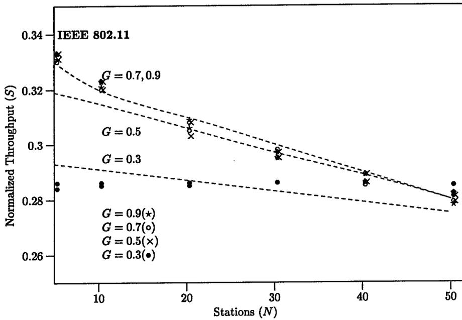
Figure 7.33: IEEE 802.11 Telemetry Throughput Model and Simulation Data
