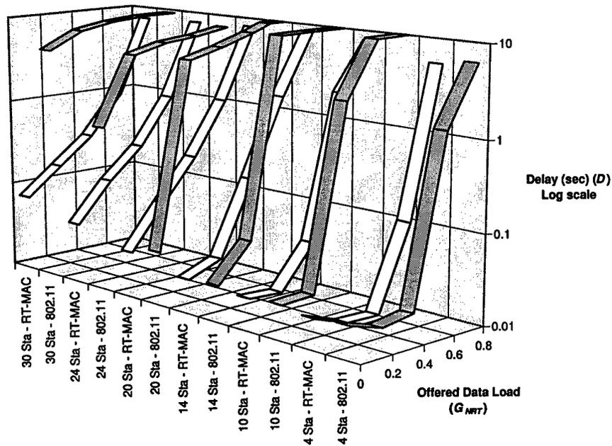
Figure 6.35: Voice Mean Delay - Bursty Error Channel (1 Mbps)
