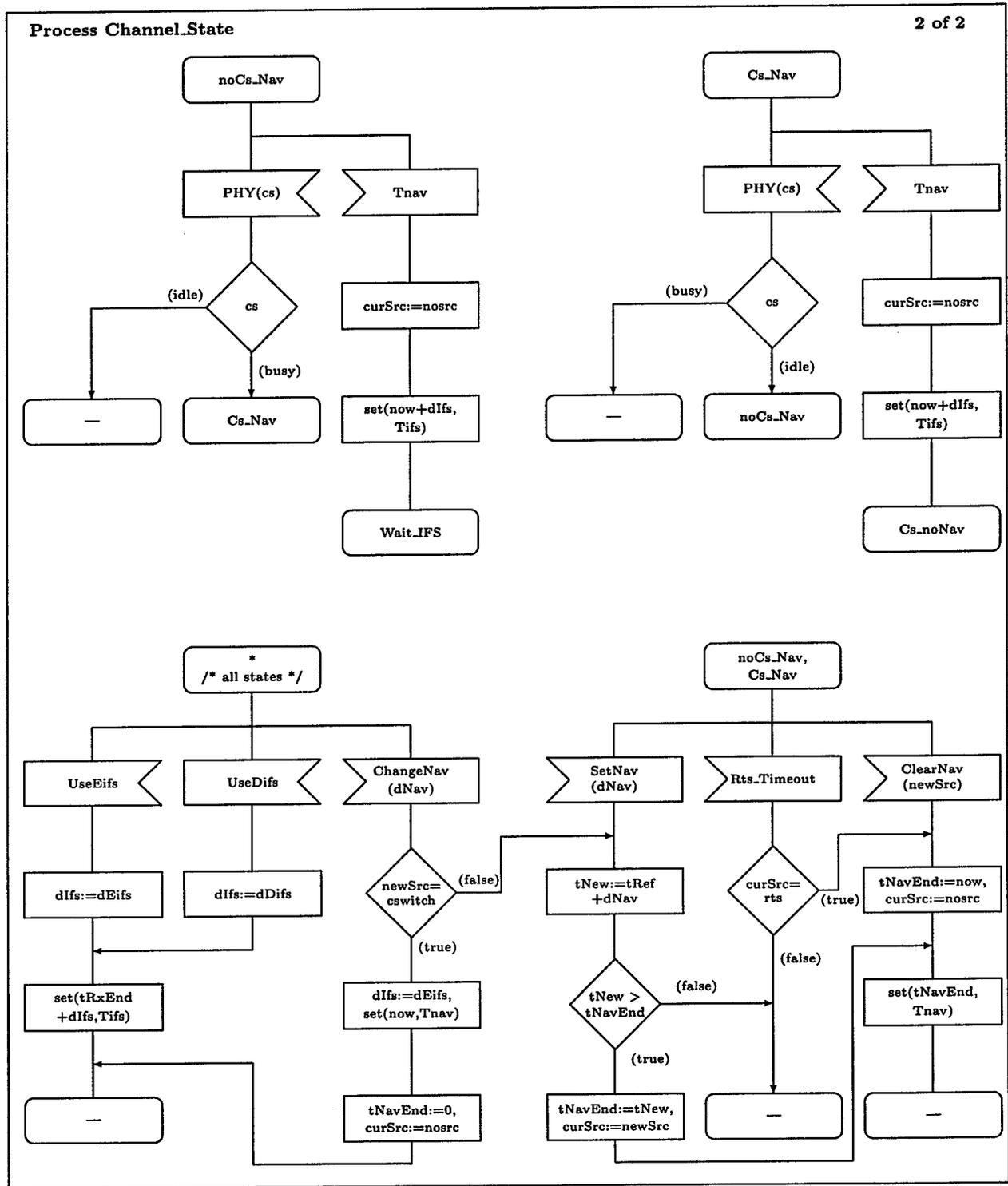
Figure A.23: Channel\_State – SDL Description (2 of 2)
