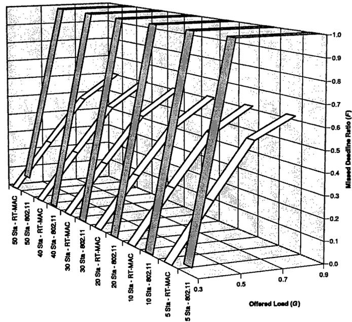
Figure 6.8: Telemetry Missed Deadline Ratio - Ideal Channel
