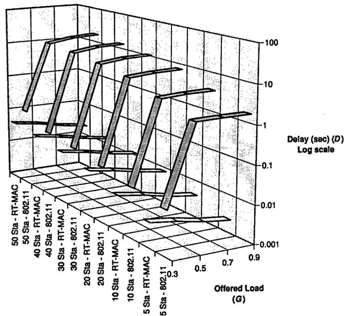
Figure 6.7: Telemetry Mean Delay - Bursty Error Channel
