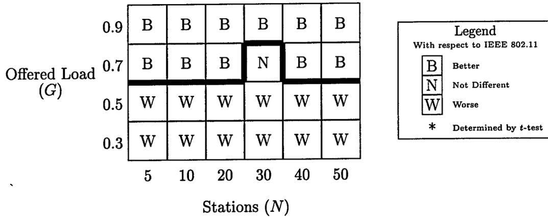
Figure 6.21: Avionics Mean Delay Performance Comparison - Ideal Channel
