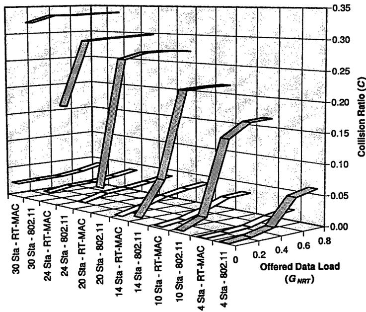
Figure 6.45: Voice Collision Ratio - Bursty Error Channel (1 Mbps)
