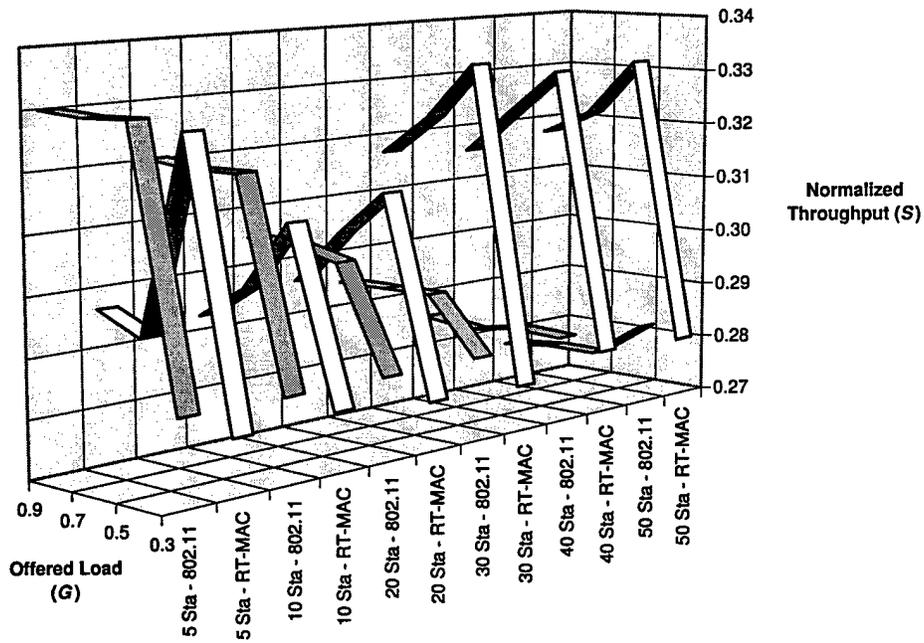
Figure 6.2: Telemetry Throughput - Bursty Error Channel
