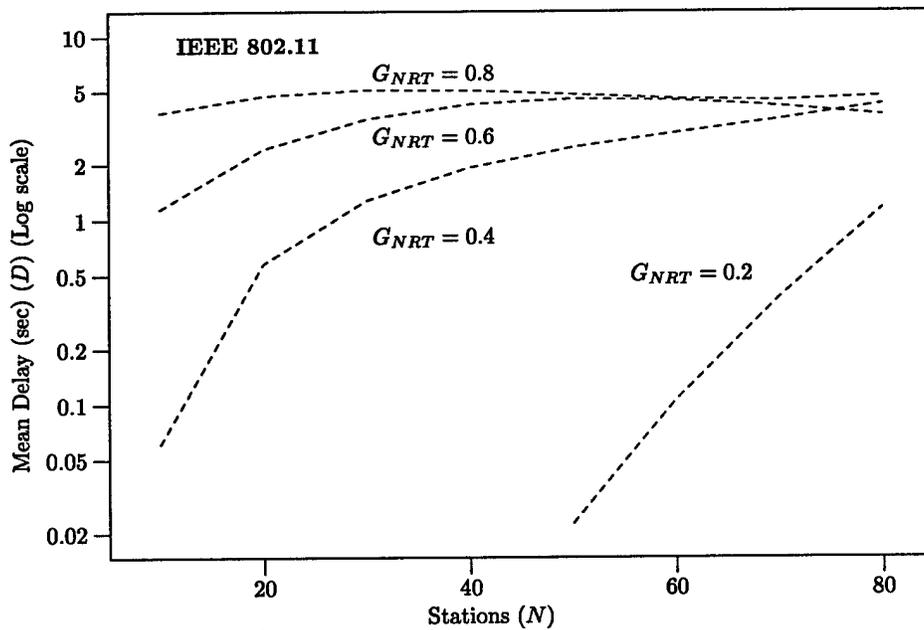
Figure 7.28: Mean Delay - Voice Traffic Model (10 Mbps) (2 of 3)
