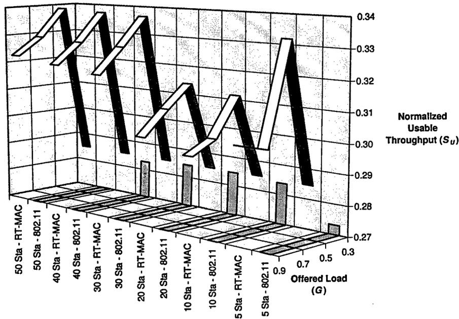
Figure 6.5: Usable Telemetry Throughput - Ideal Channel
