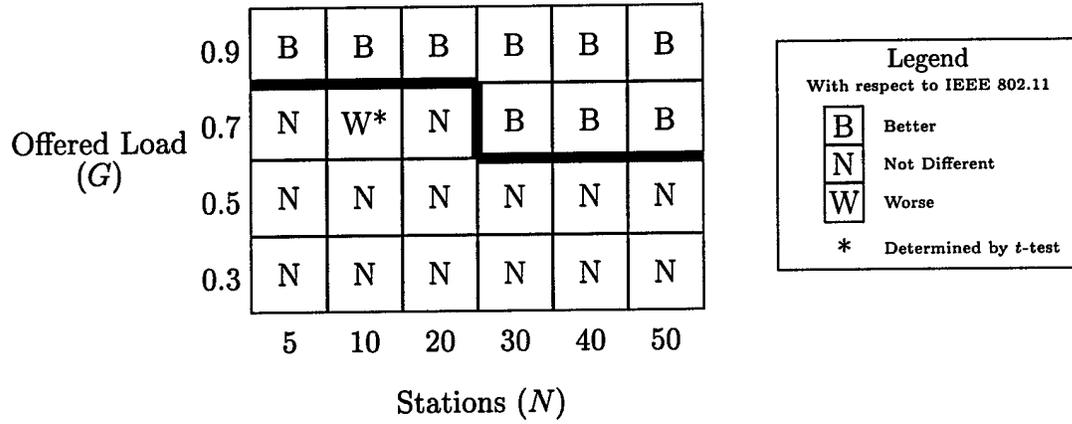
Figure 6.17: Avionics Throughput Performance Comparison - Bursty Error Channel
