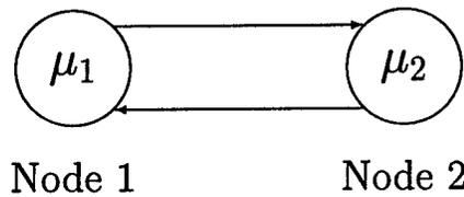
Figure 3.5: Closed Tandem Queueing Network –  $M = 2, N = 3$
