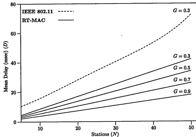
Figure 7.6: Mean Delay – Telemetry Traffic Model (2 of 2)
