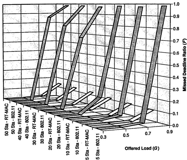
Figure 6.24: Avionics Missed Deadline Ratio - Bursty Error Channel
