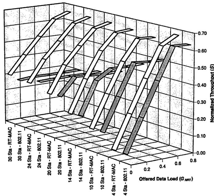
Figure 6.30: Voice Throughput - Bursty Error Channel (1 Mbps)
