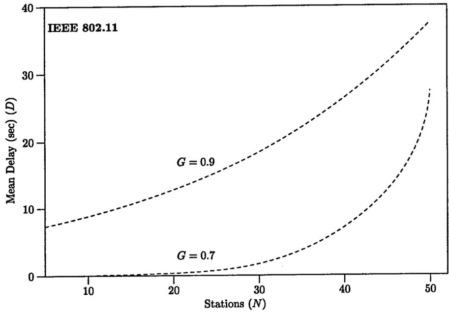
Figure 7.10: Mean Delay - Avionics Traffic Model (1 of 3)
