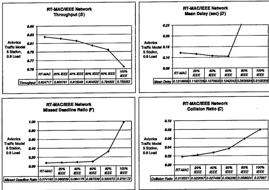
Figure 6.74: Mixed RT-MAC/IEEE 802.11 Network, Avionics Traffic Model, 5 Stations
