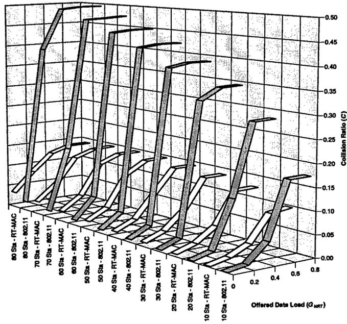
Figure 6.60: Voice Collision Ratio - Ideal Channel (10 Mbps)
