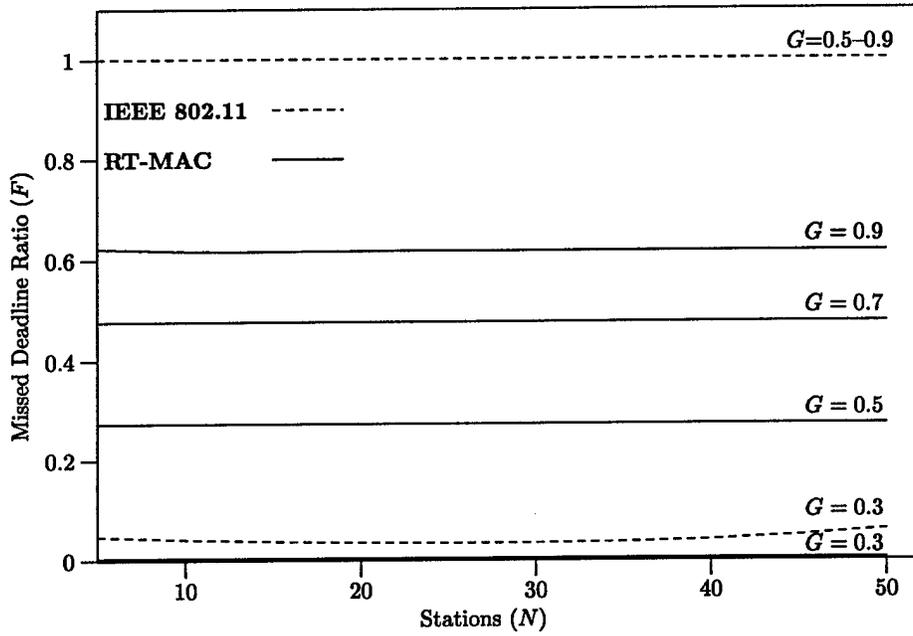
Figure 7.7: Missed Deadlines – Telemetry Traffic Model
