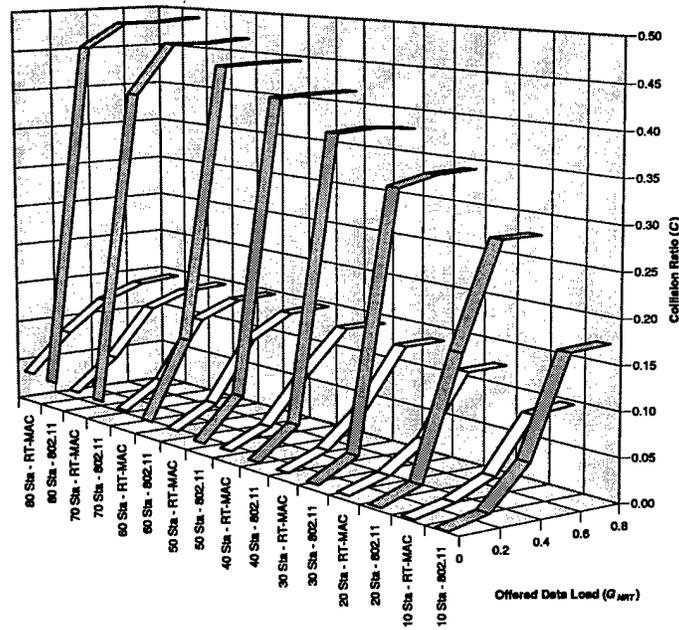
Figure 6.61: Voice Collision Ratio - Bursty Error Channel (10 Mbps)
