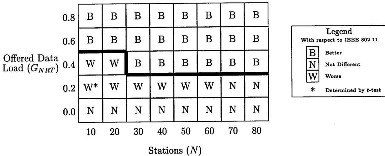
Figure 6.48: Voice Throughput Performance Comparison - Ideal Channel (10 Mbps)
