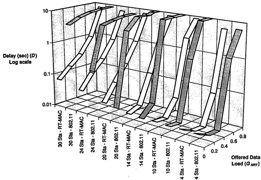
Figure 6.34: Voice Mean Delay - Ideal Channel (1 Mbps)
