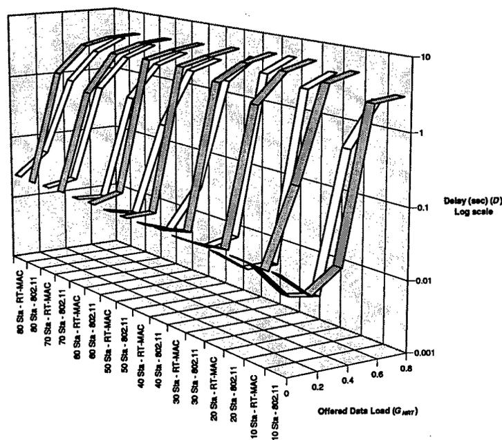
Figure 6.51: Voice Mean Delay - Bursty Error Channel (10 Mbps)
