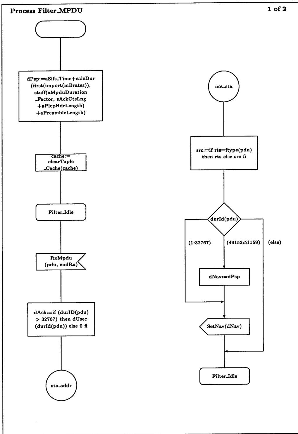
Figure A.19: Filter\_MPDU – SDL Description (1 of 2)
