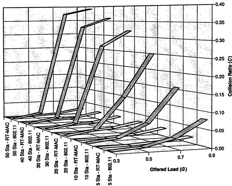
Figure 6.28: Avionics Collision Ratio - Bursty Error Channel
