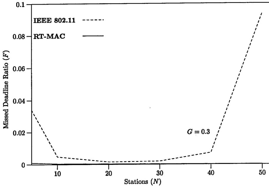
Figure 6.10: Telemetry Missed Deadline Ratio (5-50 Stations) - Ideal Channel
