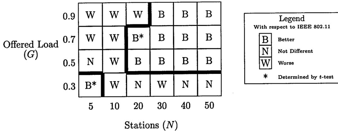
Figure 6.3: Telemetry Throughput Performance Comparison - Ideal Channel
