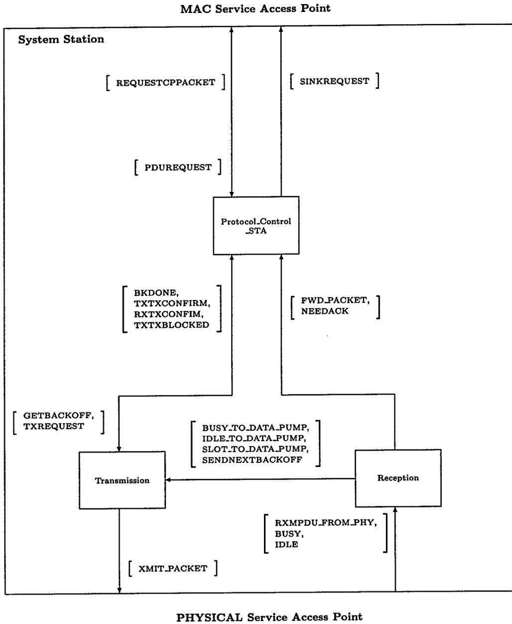
Figure A.7: SDL – System Station
