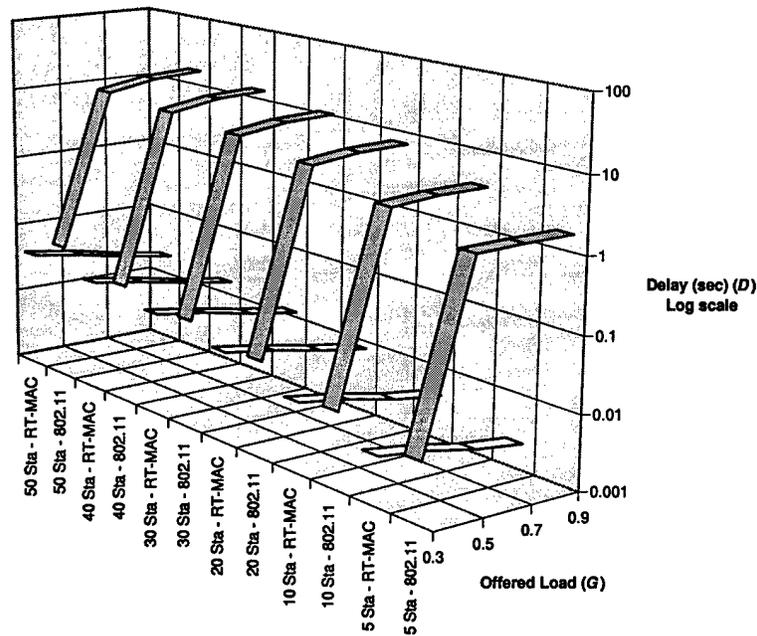
Figure 6.6: Telemetry Mean Delay - Ideal Channel
