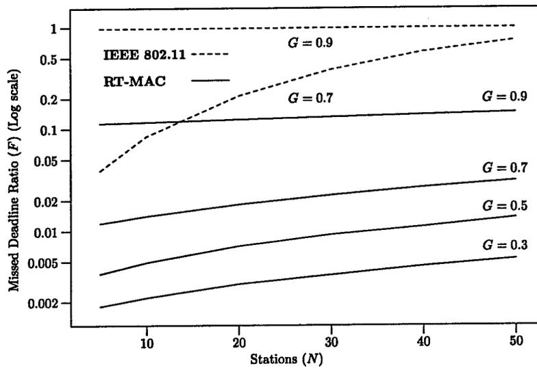
Figure 7.14: Missed Deadlines – Avionics Traffic Model (2 of 2)
