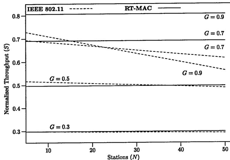
Figure 7.9: Normalized Throughput – Avionics Traffic Model
