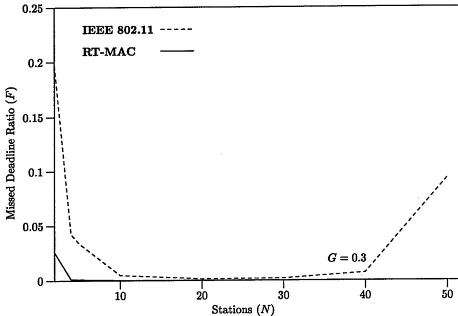
Figure 6.11: Telemetry Missed Deadline Ratio (2-50 Stations) - Ideal Channel
