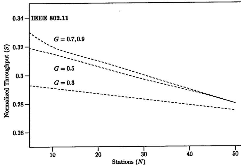
Figure 7.3: Normalized Throughput - Telemetry Traffic Model (1 of 2)
