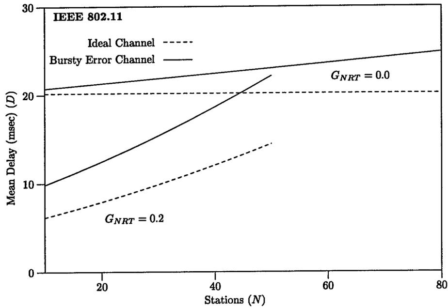
Figure 7.27: Mean Delay - Voice Traffic Model (10 Mbps) (1 of 3)
