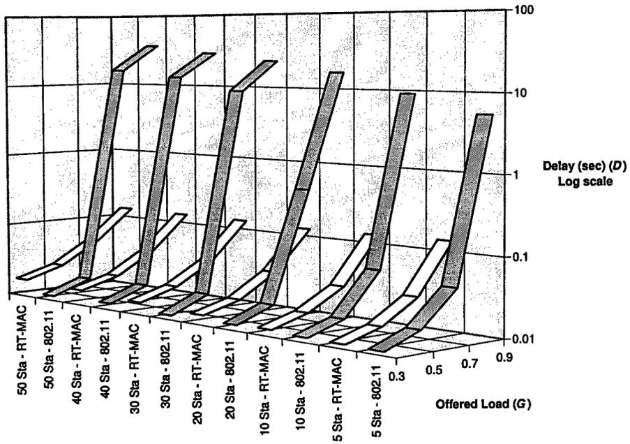
Figure 6.20: Avionics Mean Delay - Bursty Error Channel
