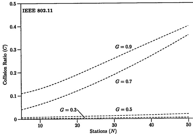
Figure 7.15: Collisions – Avionics Traffic Model (1 of 2)
