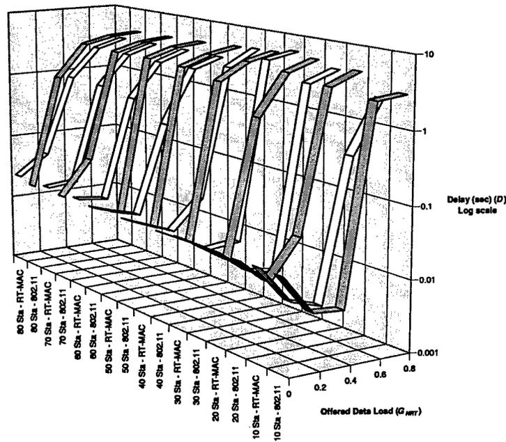
Figure 6.50: Voice Mean Delay - Ideal Channel (10 Mbps)
