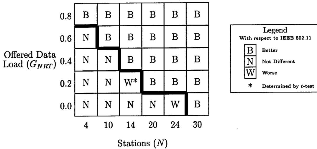
Figure 6.31: Voice Throughput Performance Comparison - Ideal Channel (1 Mbps)
