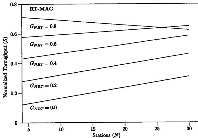
Figure 7.18: Normalized Throughput – Voice Traffic Model (1 Mbps) (2 of 2)
