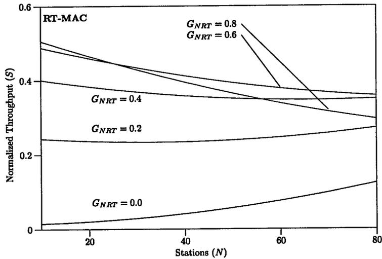
Figure 7.26: Normalized Throughput – Voice Traffic Model (10 Mbps) (2 of 2)
