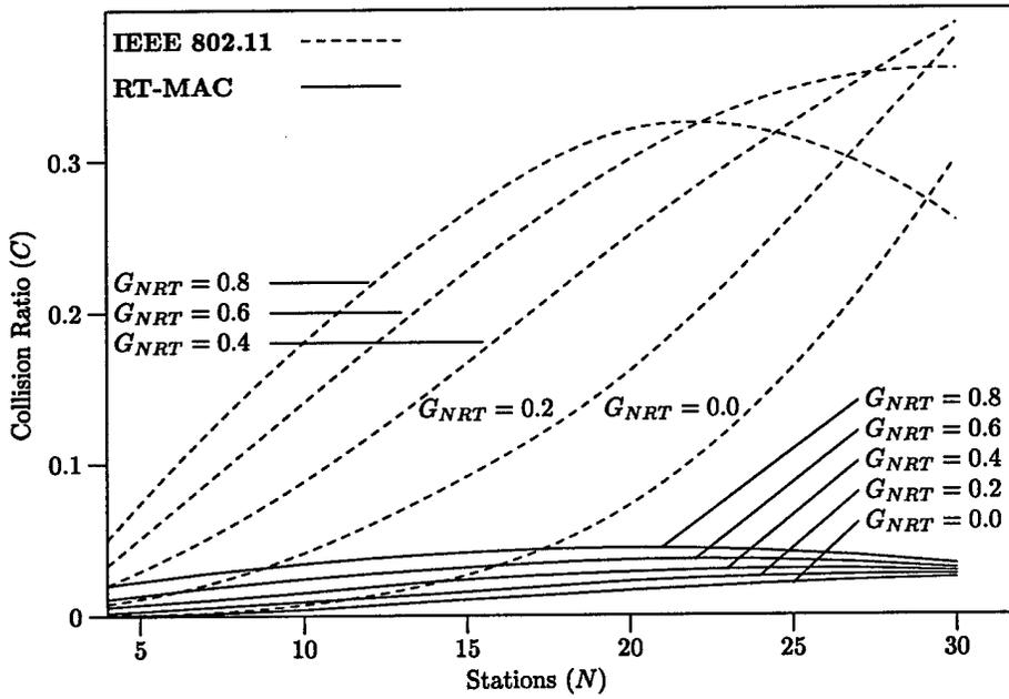
Figure 7.24: Collisions – Voice Traffic Model (1 Mbps)
