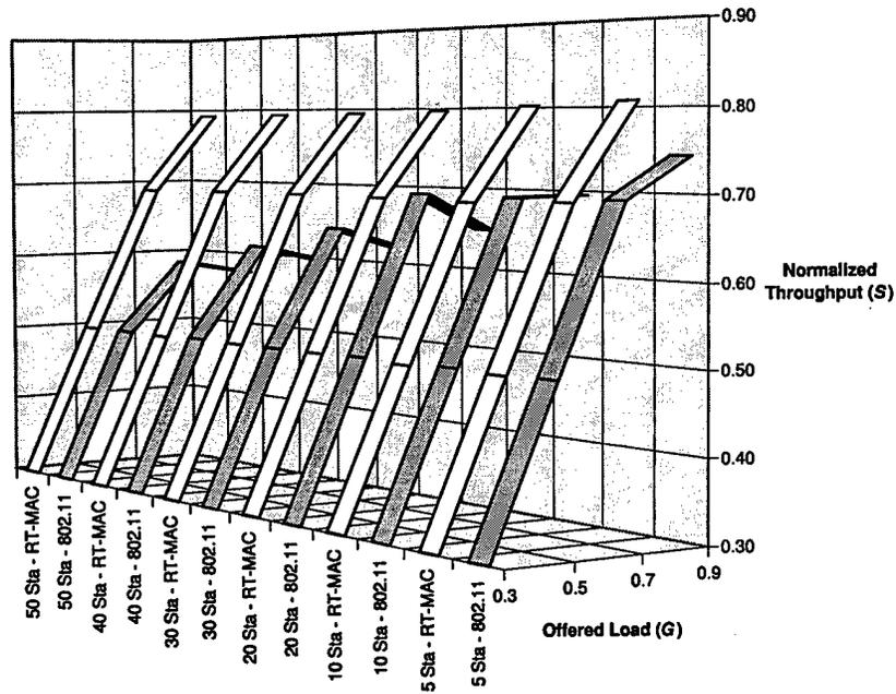
Figure 6.15: Avionics Throughput - Bursty Error Channel
