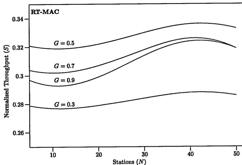
Figure 7.4: Normalized Throughput - Telemetry Traffic Model (2 of 2)
