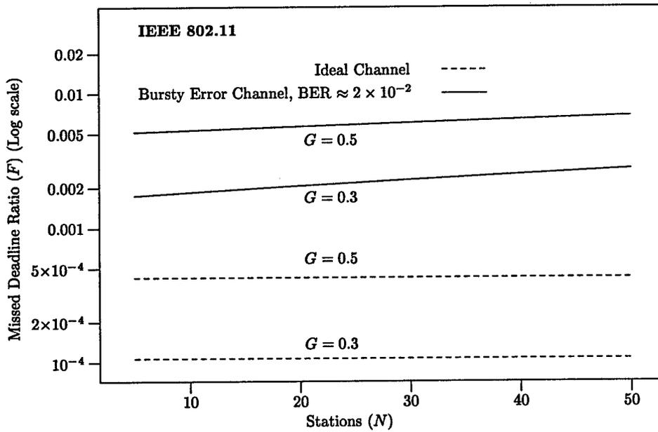
Figure 7.13: Missed Deadlines – Avionics Traffic Model (1 of 2)
