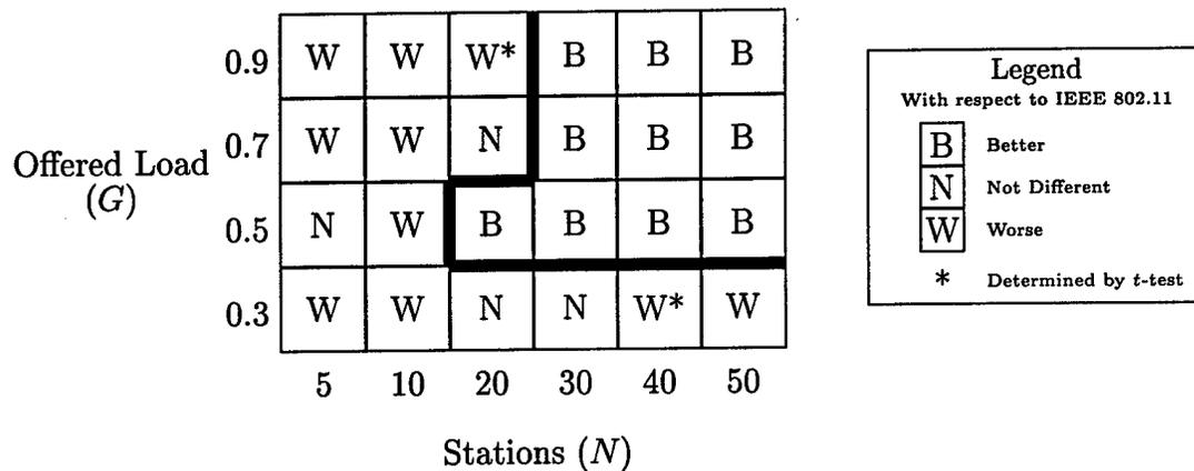
Figure 6.4: Telemetry Throughput Performance Comparison - Bursty Error Channel
