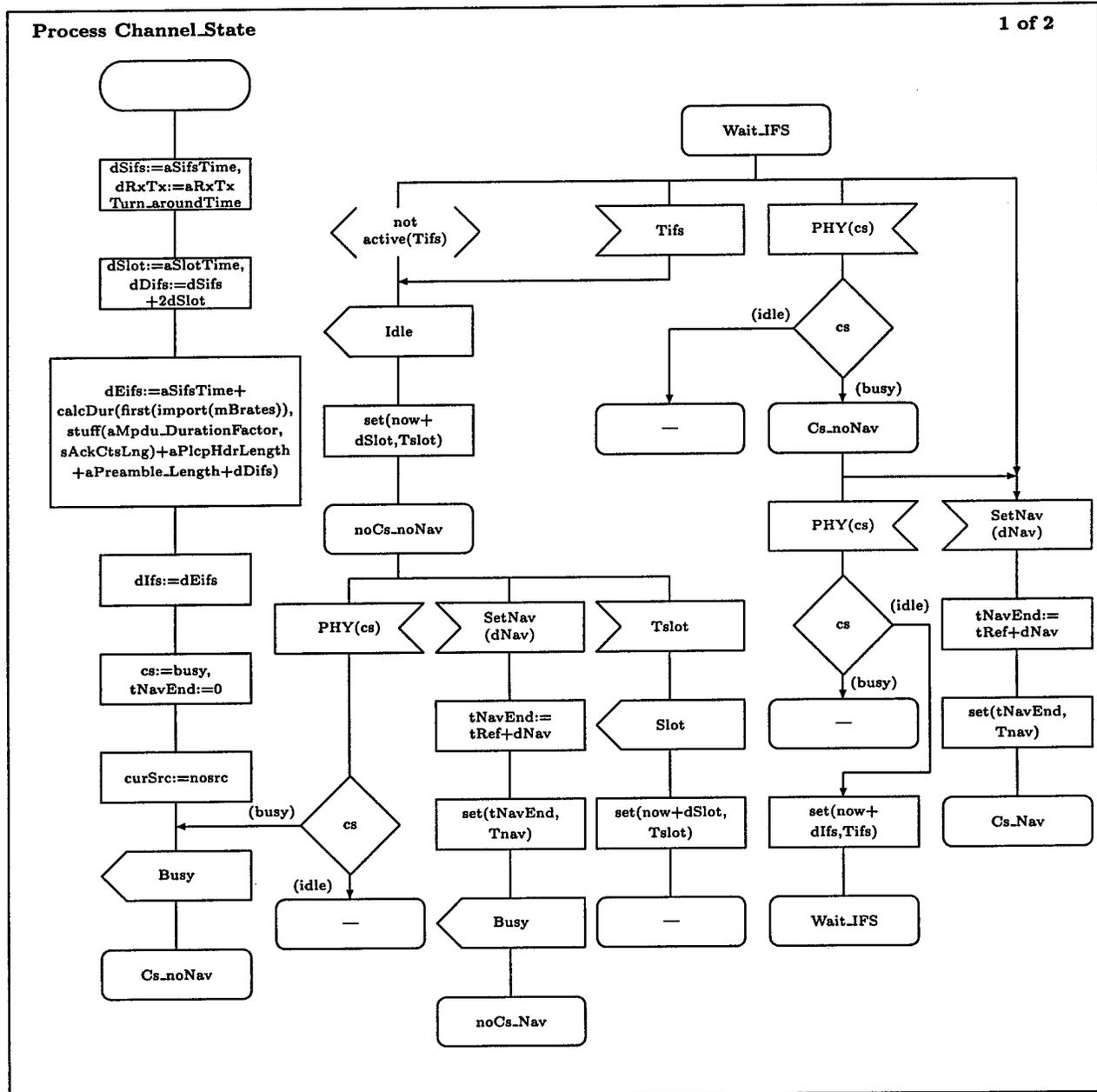
Figure A.22: Channel\_State – SDL Description (1 of 2)
