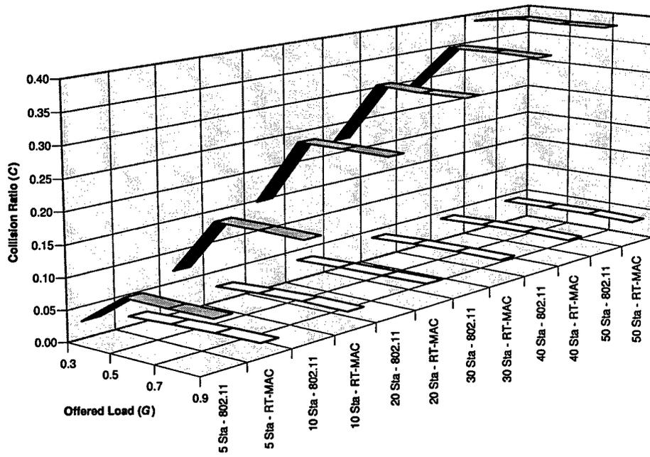
Figure 6.12: Telemetry Collision Ratio - Ideal Channel
