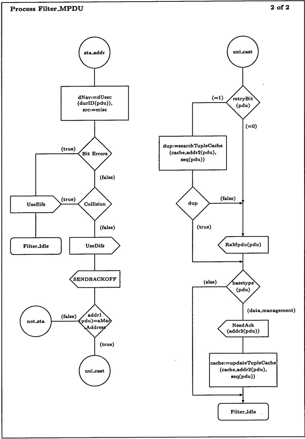
Figure A.20: Filter\_MPDU – SDL Description (2 of 2)
