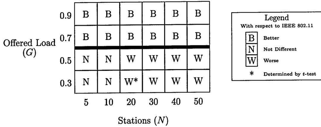
Figure 6.25: Avionics Missed Deadline Performance Comparison - Ideal Channel
