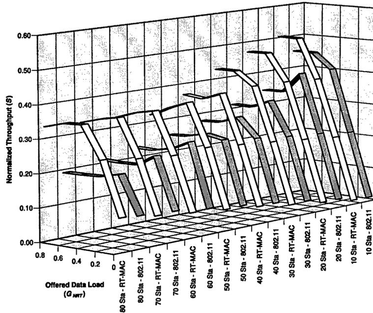
Figure 6.47: Voice Throughput - Bursty Error Channel (10 Mbps)
