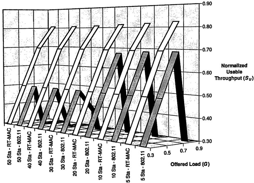
Figure 6.18: Usable Avionics Throughput - Ideal Channel
