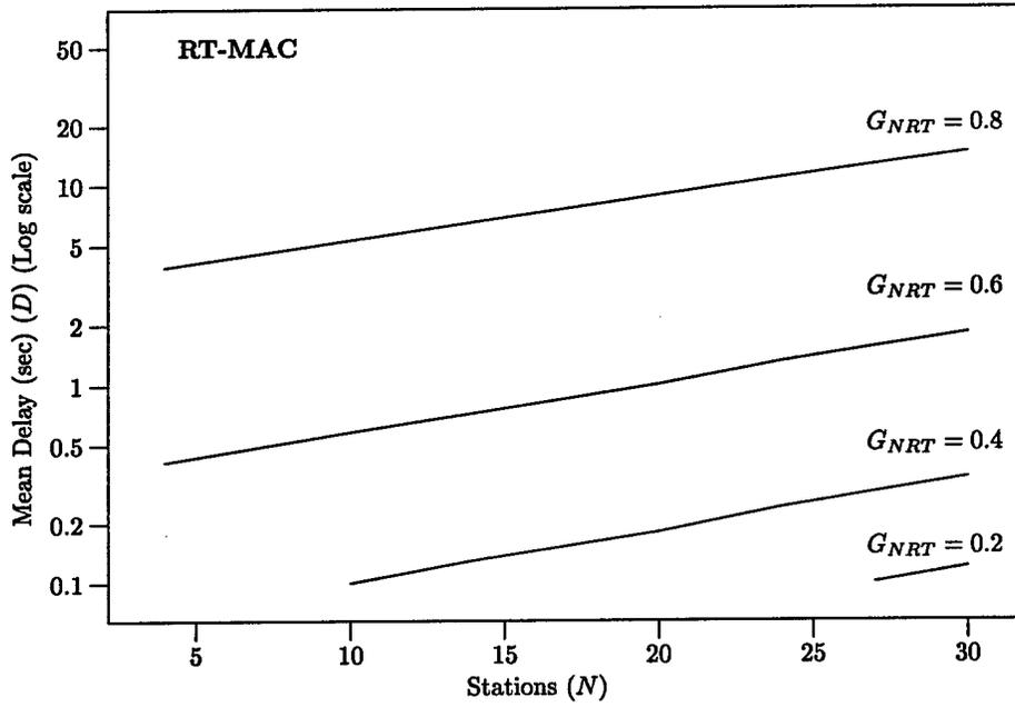
Figure 7.21: Mean Delay – Voice Traffic Model (1 Mbps) (3 of 3)
