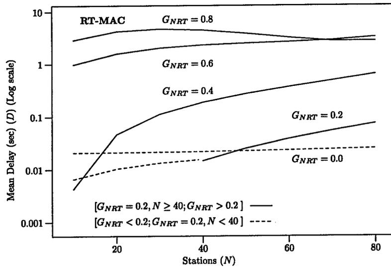
Figure 7.29: Mean Delay – Voice Traffic Model (10 Mbps) (3 of 3)
