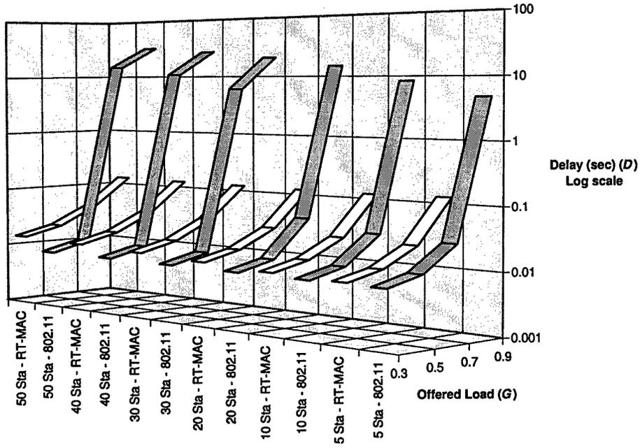
Figure 6.19: Avionics Mean Delay - Ideal Channel
