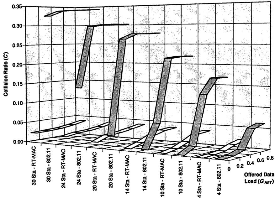
Figure 6.44: Voice Collision Ratio - Ideal Channel (1 Mbps)
