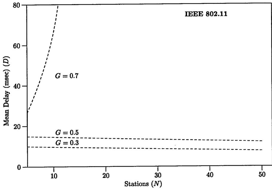
Figure 7.11: Mean Delay - Avionics Traffic Model (2 of 3)
