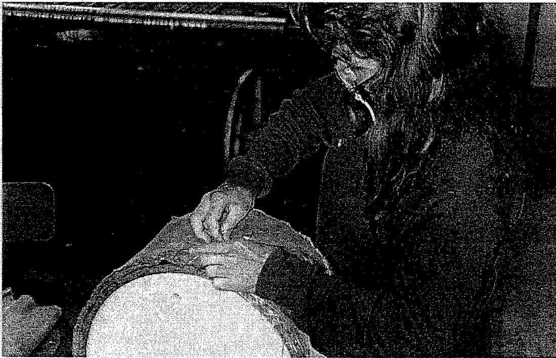
FIGURE 33. LAYUP OF PBO CONTAINMENT RING
