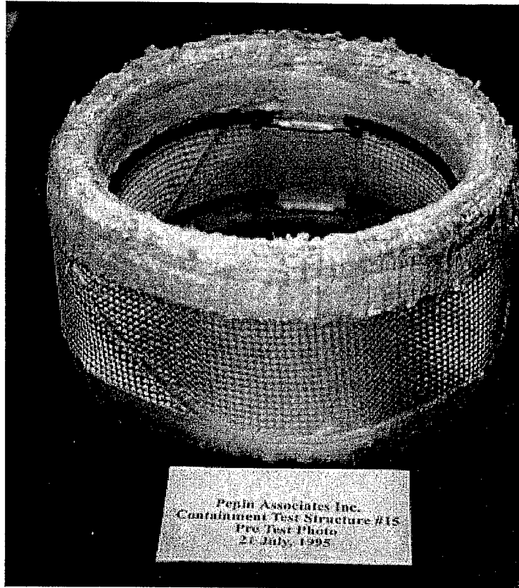
FIGURE 6. S GLASS RING WITH \pm 45^\circ REINFORCEMENT
