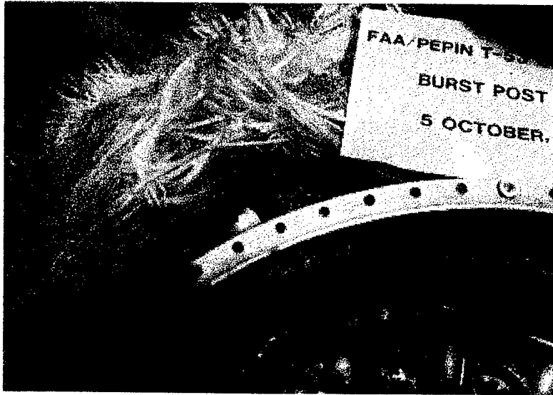
FIGURE 19. CLOSE-UP PHOTO OF AREA BETWEEN COMBUSTOR CASE AND CONTAINMENT RING AFTER TEST OF FIRST LARGE-DIAMETER KEVLAR CONTAINMENT RING
