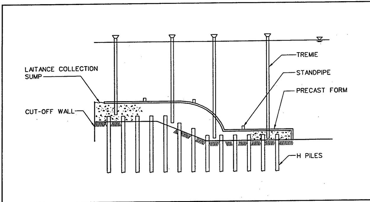
Figure 2. Tremie concreting into precast concrete form
