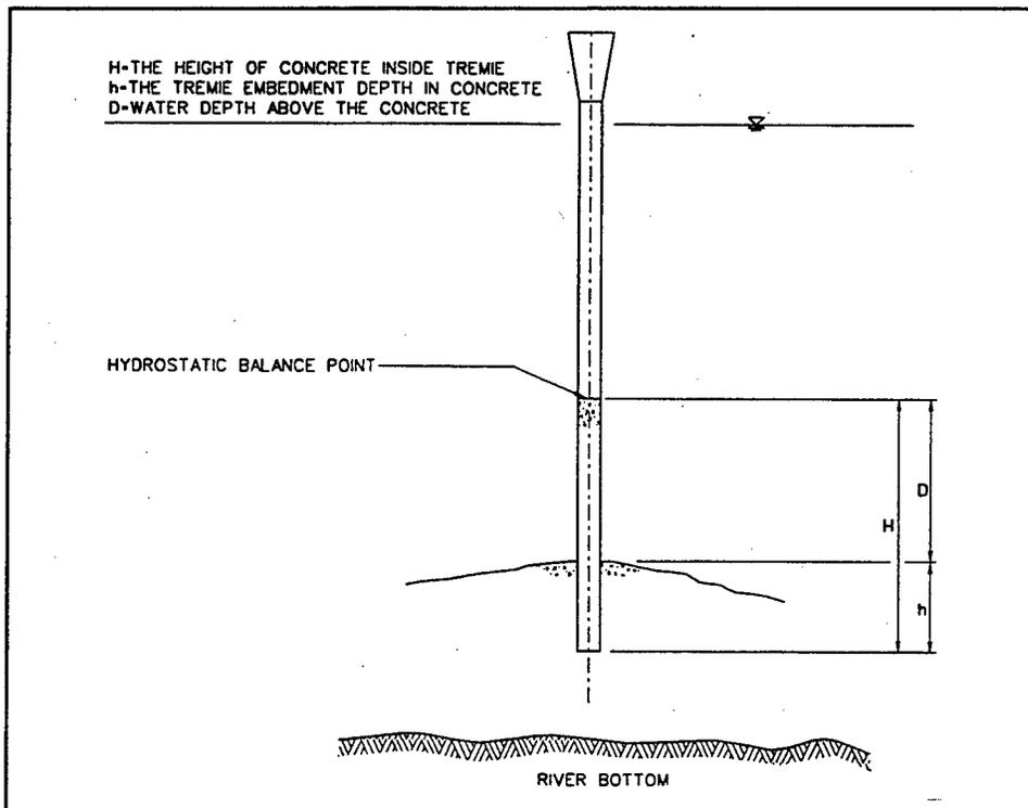
Figure 14. Hydrostatic balance point in a tremie system
