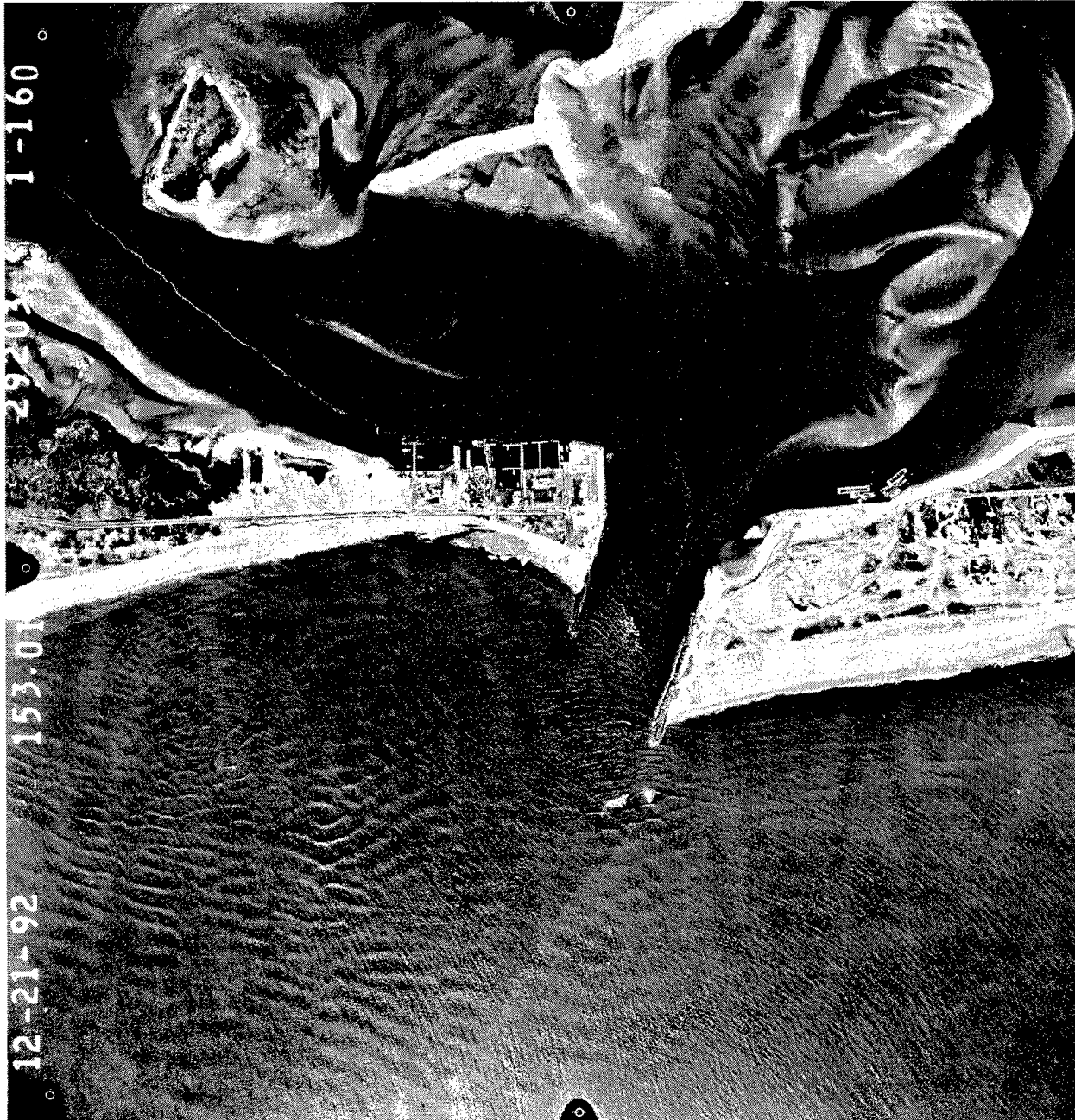
Figure A40. 21 December 1992 (Similar conditions as previous photographs taken 3 days earlier. Waves still appear to be concentrated along the east shore where part of the jetty has failed. T-shaped sandbar in flood shoal has been divided into two sections)
