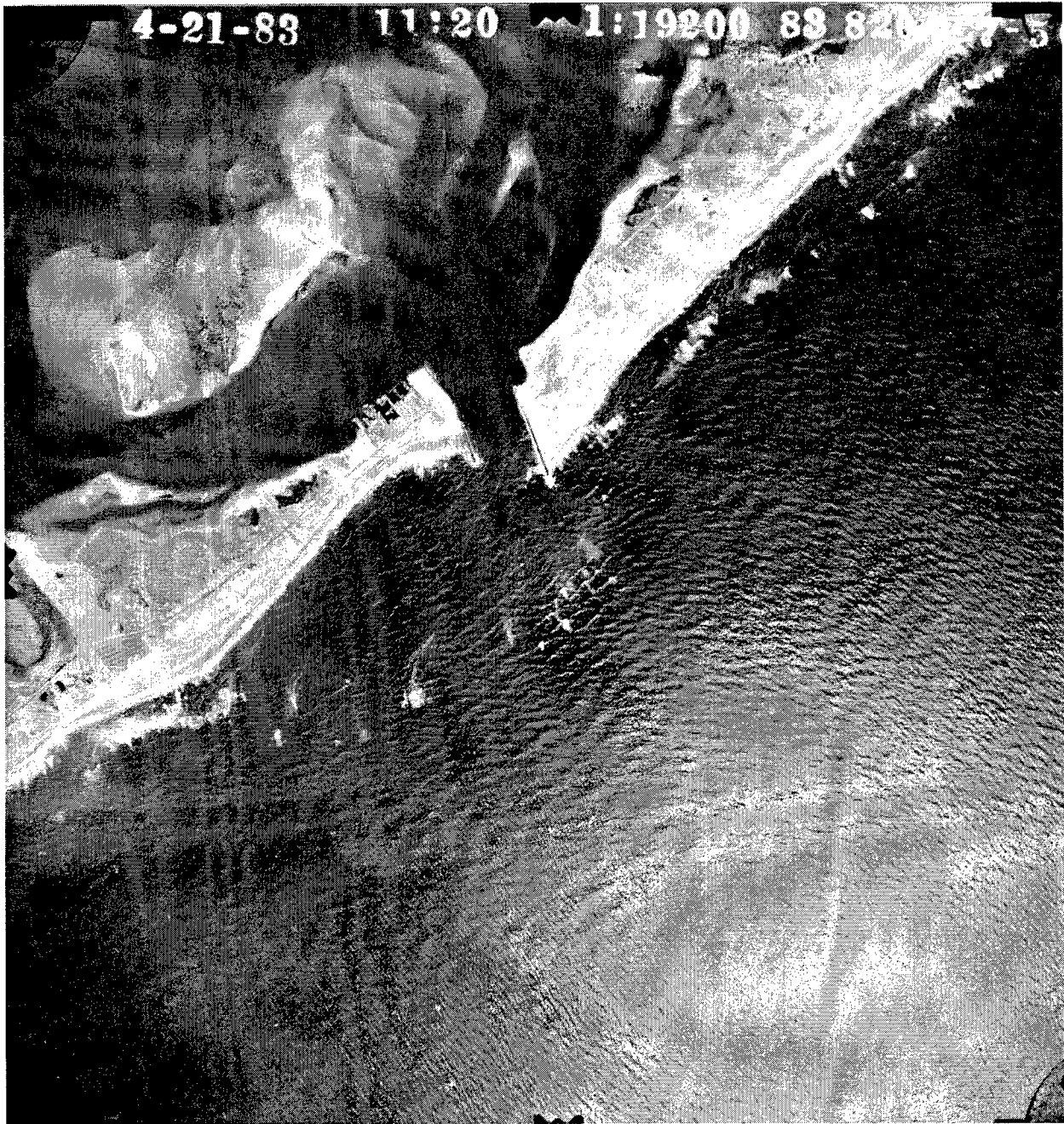
Figure A28. 21 April 1983 (Oval ebb shoal is outlined by breaking waves. The shoal attaches to downdrift (west) beach at the bulge in the shoreline. Bulge has moved about 500 m west compared with 1976)
