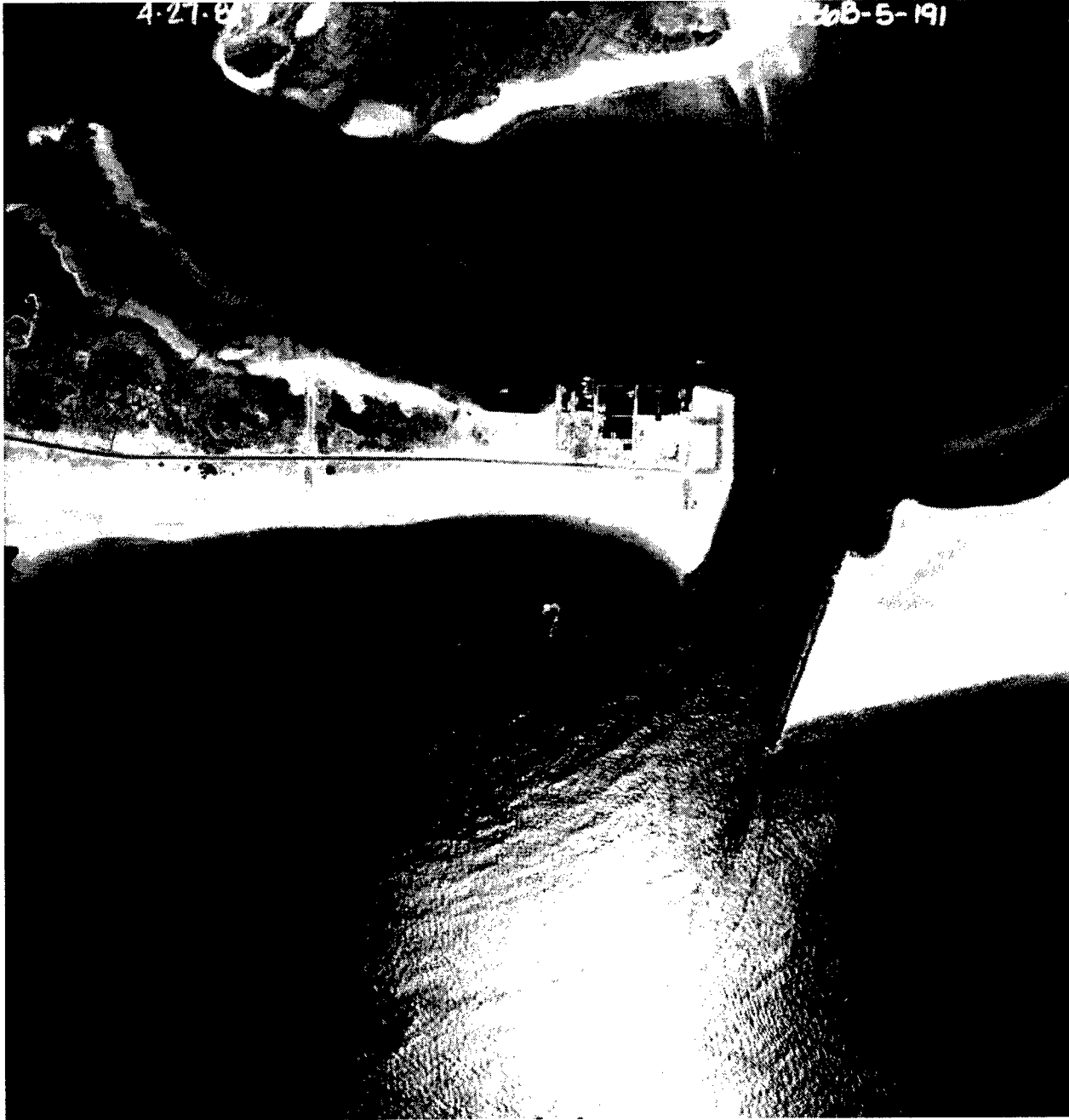
Figure A29. 27 April 1984 (Only minor shoreline changes have occurred since 1983. However, the dunes on the west beach have eroded further, and vegetation line now stops well west of the fishing docks) (Photograph courtesy of Moffatt & Nichol Engineers)
