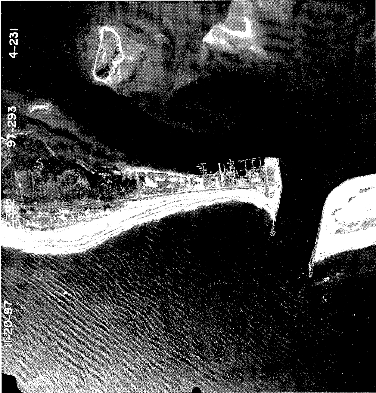
Figure A52. 20 November 1997 (In only a month, west beach had notably receded. Image shows how narrow the west beach is near fishing docks and, therefore, how vulnerable to breaching. The shoreline bulge where ebb shoal attaches to beach has continued to advance seaward. Because of clear water, sandbars off the east beach are visible)
