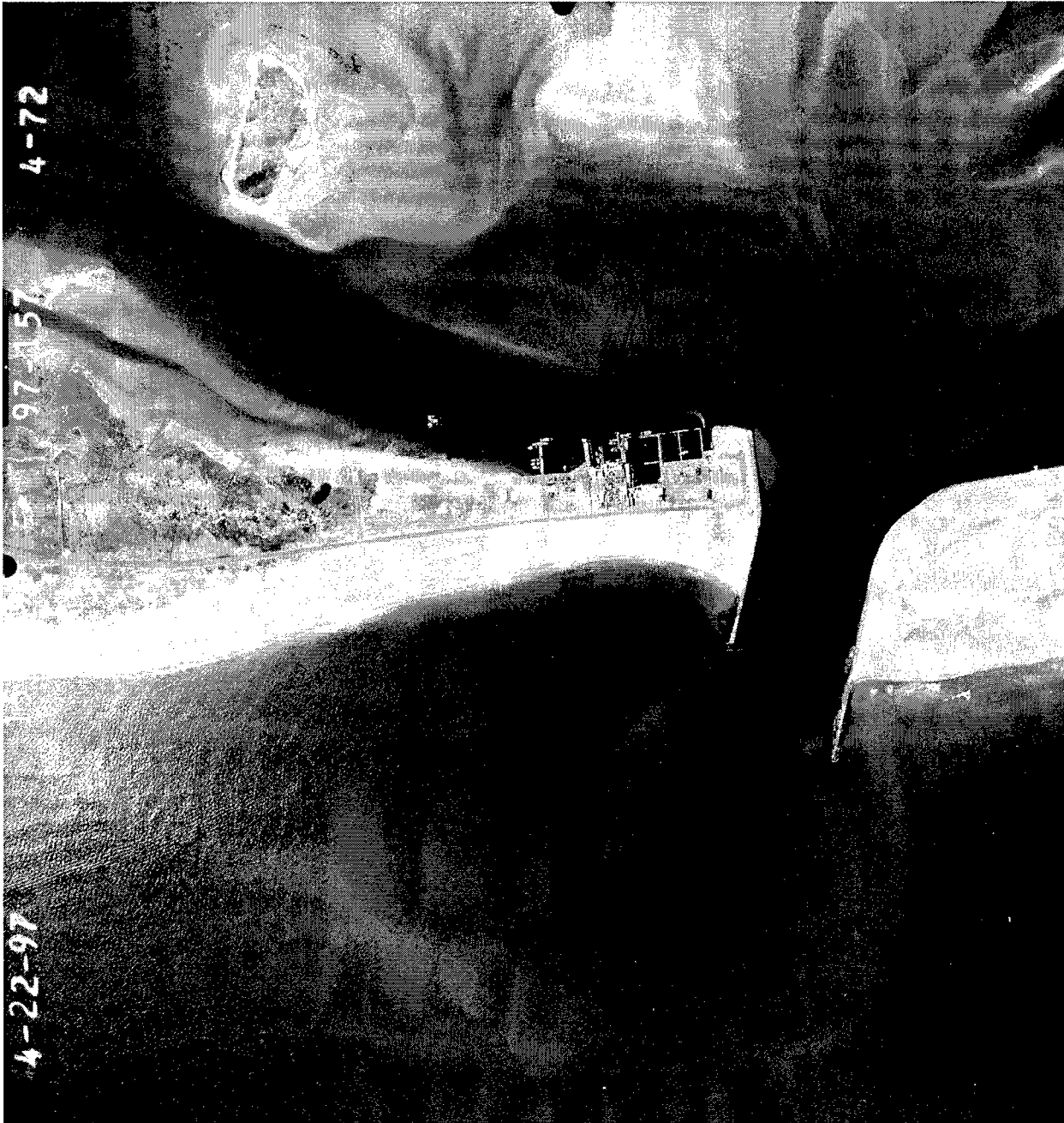
Figure A50. 22 April 1997 (Edge of ebb shoal is clearly visible in this image, taken on a day with almost no waves. Water depth at the bar is about 3 m (10 ft). Dark water off the mouth of the inlet is the dredged deposition basin. A ridge of sand that projects seaward from the west jetty and a deep hole to its west were measured by bathymetric surveys (see Appendix B))
